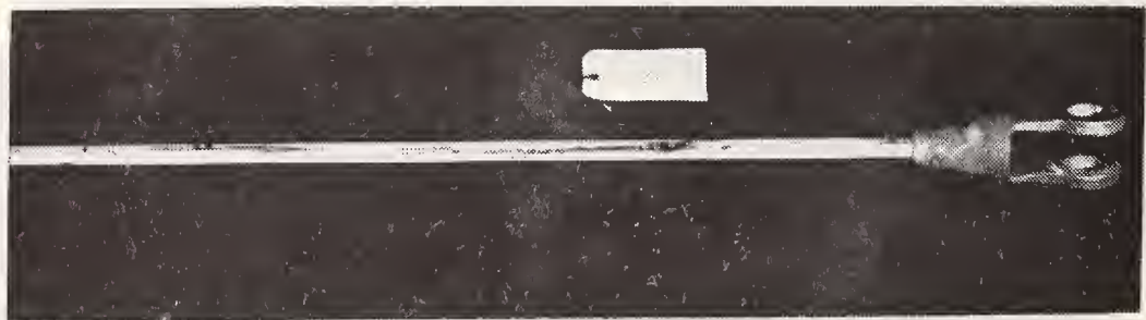
Figure 17. Upper end of Rod X16 showing long carbonaceous track on the surface opposite to that depicted in Figure 16.
