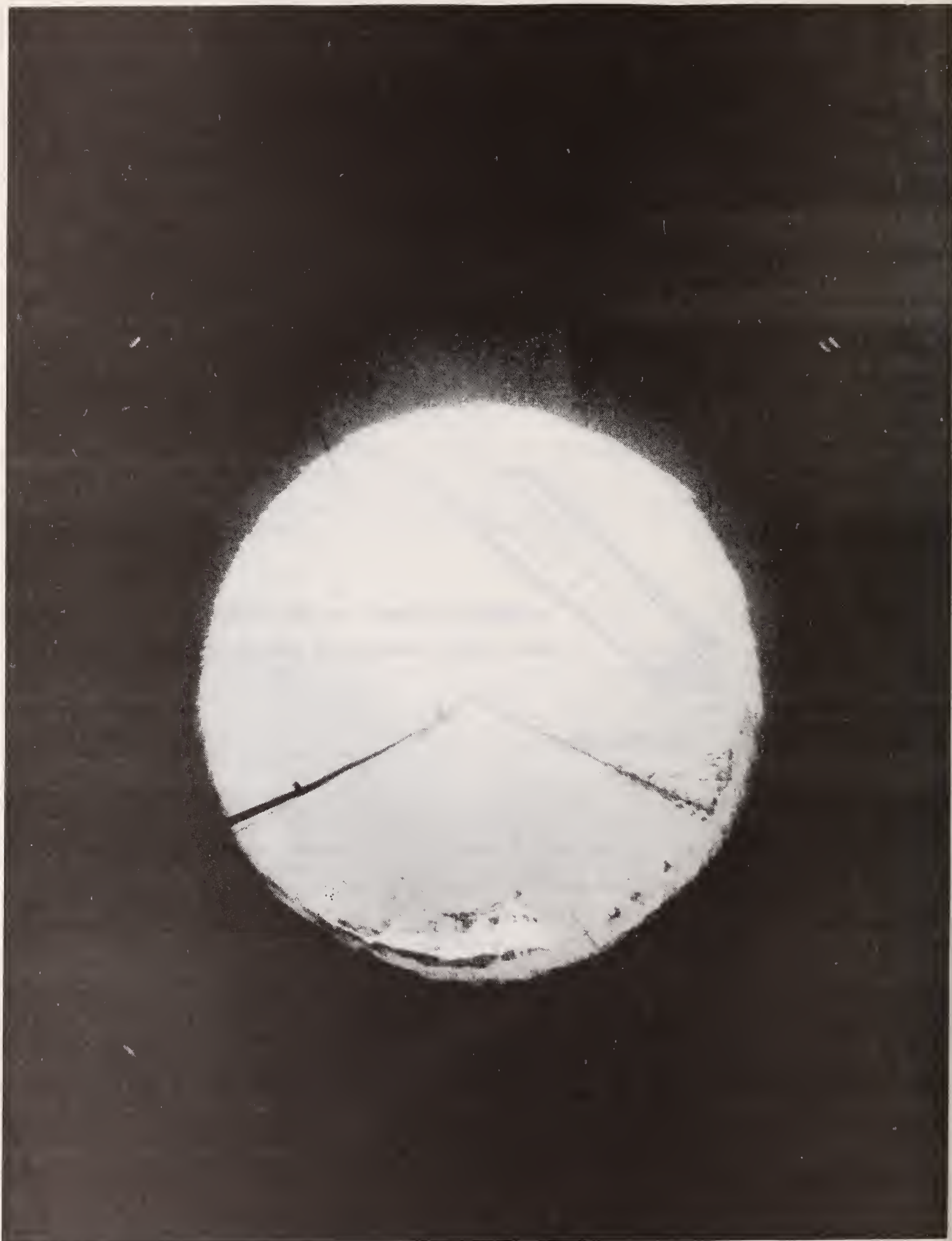
Fig. 2 Photograph in the zenith direction from 10 meters showing the Snell circle, with details of the ship. The four bright spots separated by 90^\circ mark the horizontal direction underwater.
