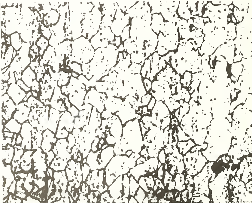
Fig. 9B. Photomicrograph of 310 SS after testing at 1000°F at a constant strain rate of 8.43 \cdot 10^{-7} \text{ S}^{-1} . Etched for 5 seconds at 5 volts in 10% oxalic acid. 500 X
