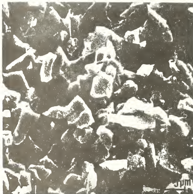
Fig. 2 Examples of 5 \mu\text{m} sized \text{Al}_2\text{O}_3 abrasive particles.
