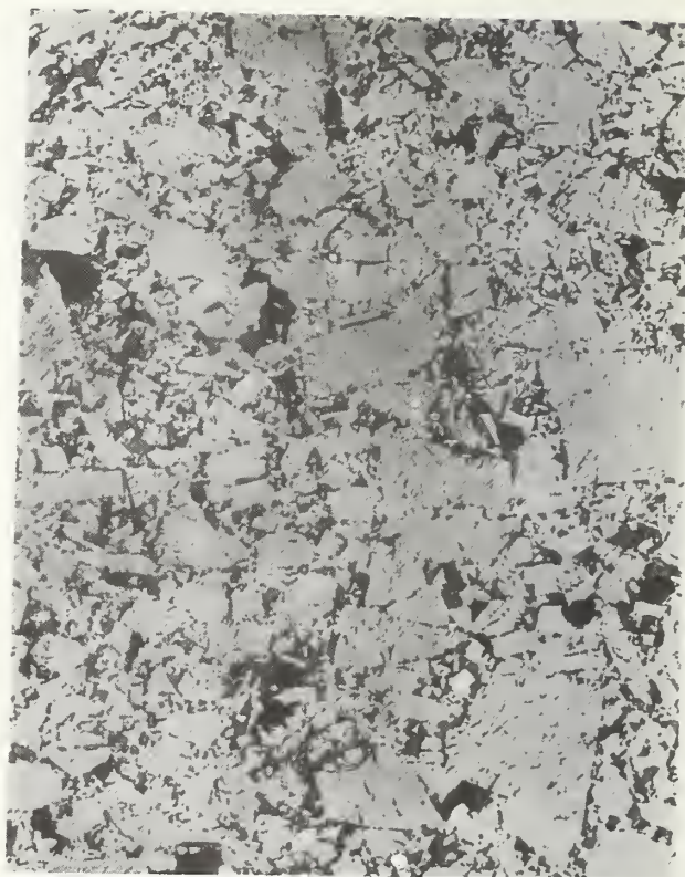
Figure B.4.3. Representative Microstructures of MgO Insulator C-1 with Hot Pressing Direction Parallel to MgO Surface (As-Polished).
