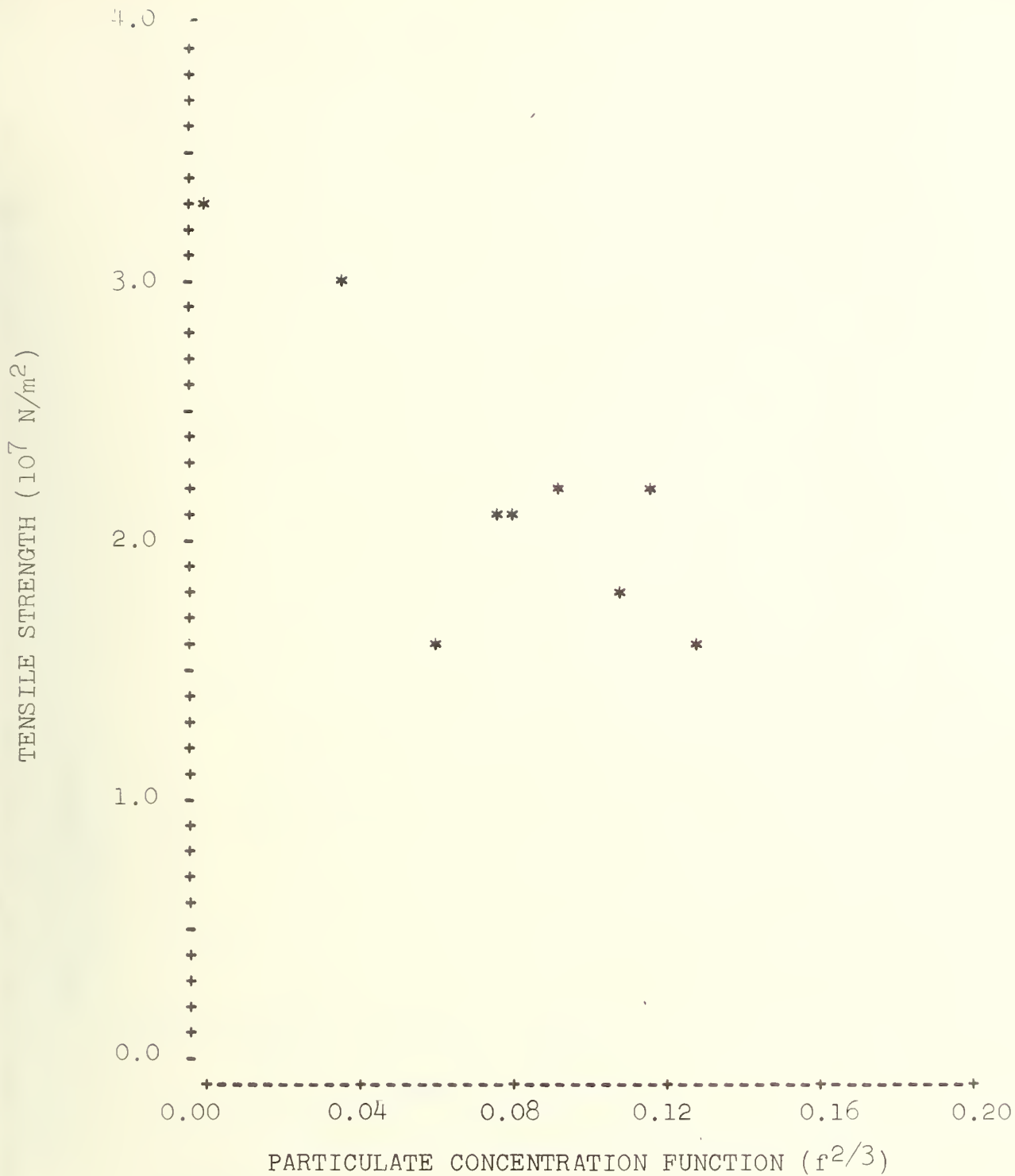
Fig. 3 : Tensile strength as a function of f^{2/3} for averages of replicate specimens of uncoated HA in Bis-GMA polymer. (Polymerization initiated by a single 15-minute exposure to sun lamp.)
