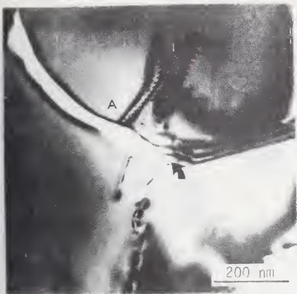
Fig. 9. Tip of grain boundary crack in Fig. 8a showing dislocation arrays extending into adjacent grains.
