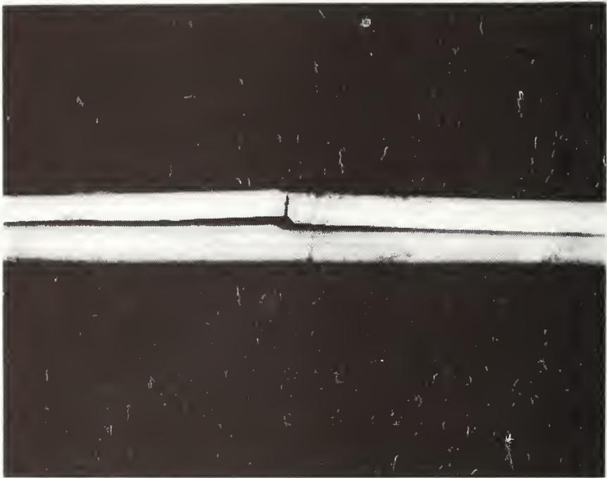
Figure 8. Failed section of glass fiber-reinforced-plastic tower guy.
