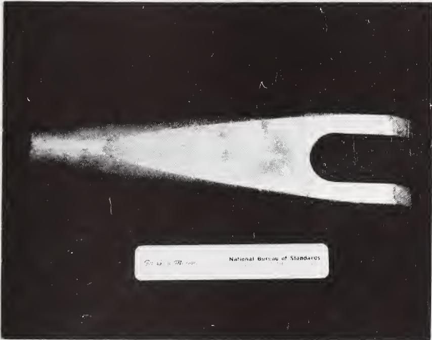
Figure 5. Proprietary, potted, compression-type end fitting. (NBS designation: Type S.)
