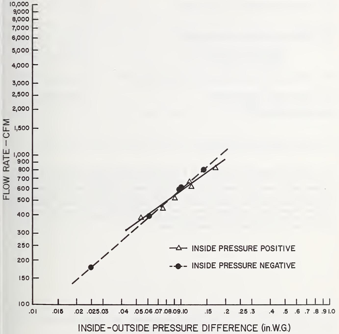
Figure 9 Comparison of Air Leakage Induced by Positive or Negative Pressurization of Mobile Home
