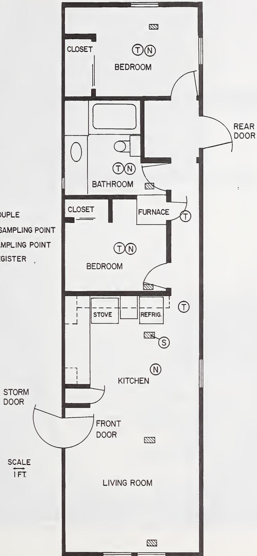
Figure 1 Floor Plan of Mobile Home
