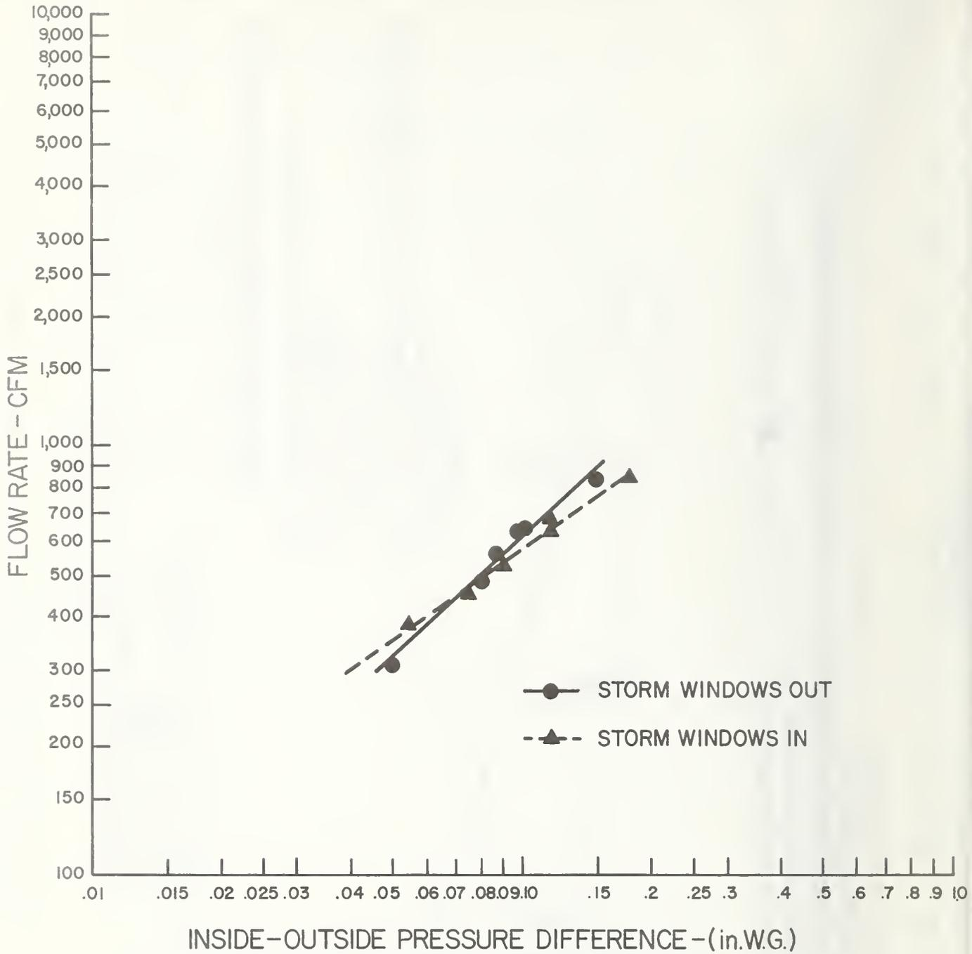
Figure 8 Effect of Storm Windows on Mechanically Induced Air Leakage - Pressure in Mobile Home Negative
