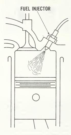
Envision a conventional spark ignition engine with the spark plugs replaced by fuel injectors. The intake valve delivers only air and the upward moving piston compresses it to such a high pressure and temperature that combustion is spontaneous the instant fuel is delivered by the injector. This combustion drives the piston down in the normal manner to deliver power to a crankshaft. The spent gases are then pumped out through a standard exhaust valve.
