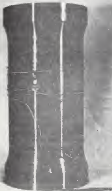
Figure 7 - Load cell showing the strain gage installation
