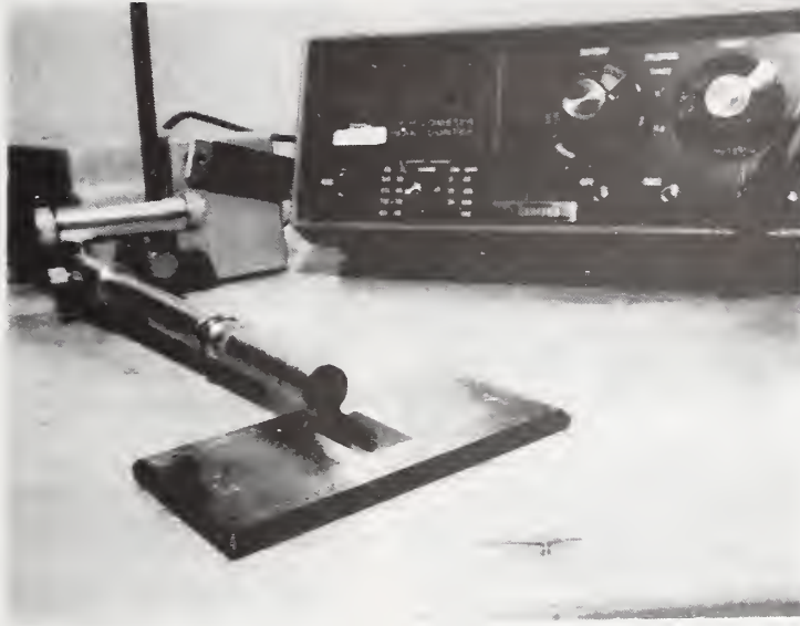
Figure 4: Typical stylus instrument
