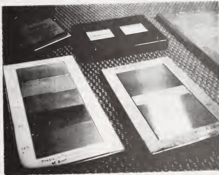
Figure 5: Precision reference specimens of roughness
