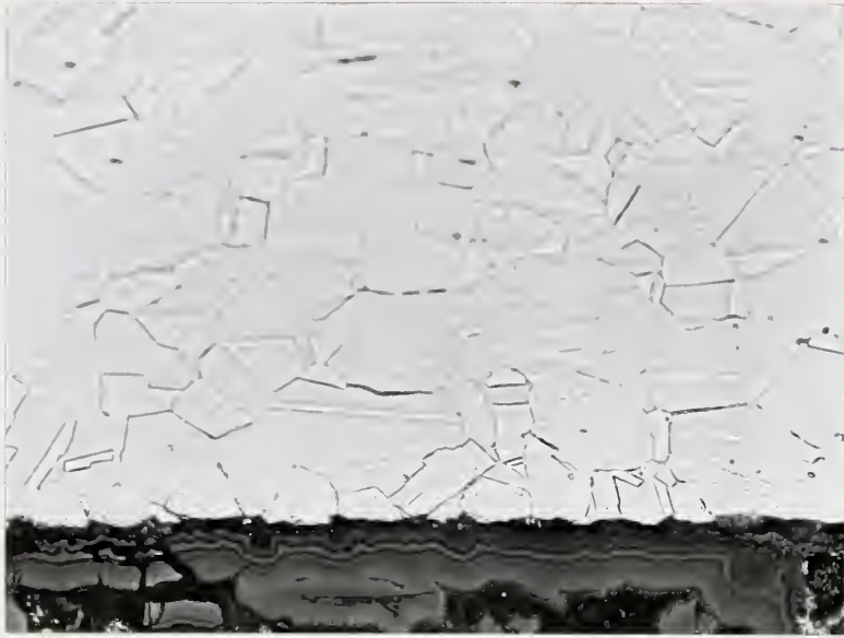
Figure 13a. Grain structure of the dome metal near the crevice at some point between A and B in Figure 8.
