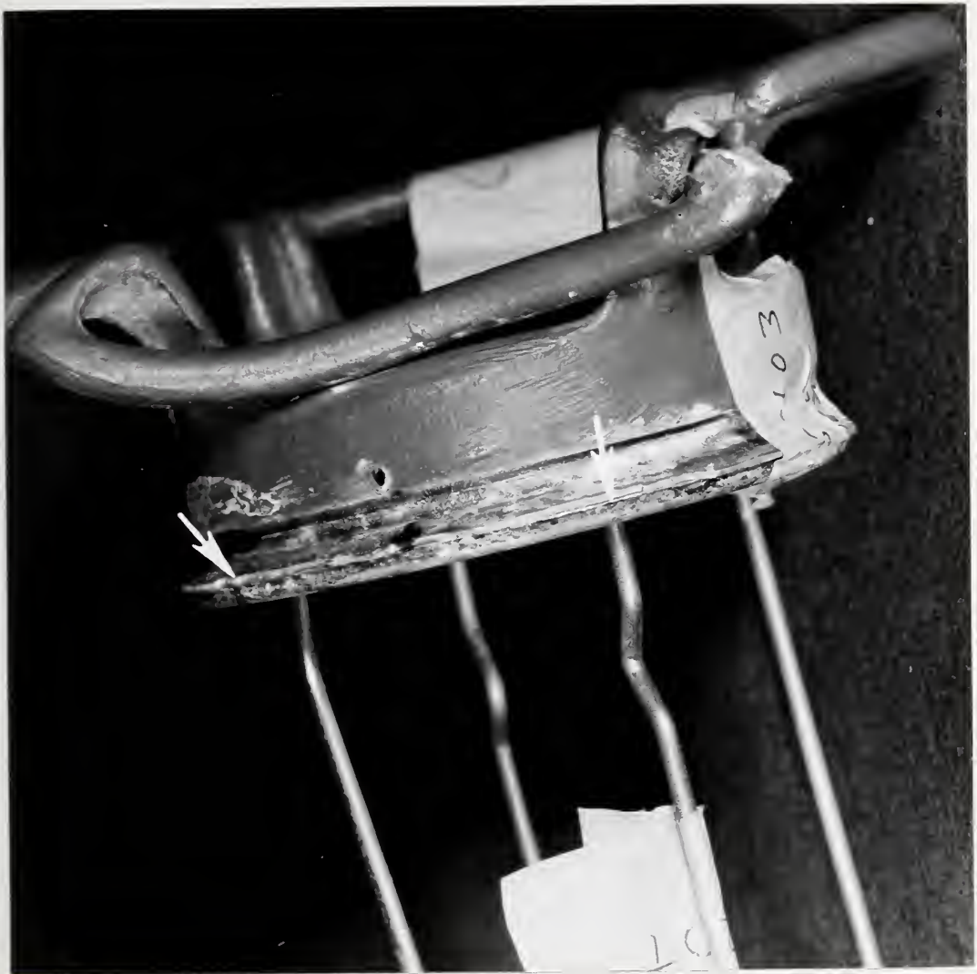
Figure 2a. Cap-collar assembly showing the ring of dome metal which remained attached to the collar - arrow at left. A fin-like projection of what is believed to be joining metal appears at the arrow - right center.
