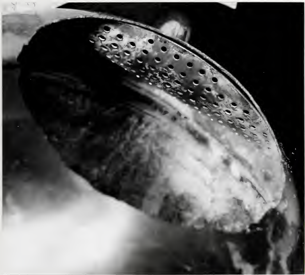
Figure 4a. Close-up view of the circumferential tear. X 1 1/4
