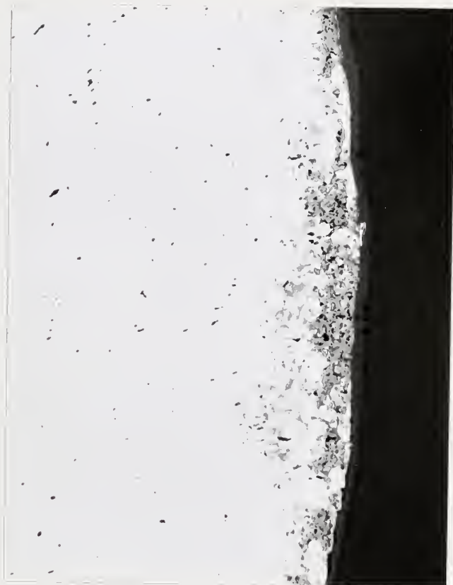
Figure 15. A section of the collar metal near D in Figure 8, showing surface film of corrosion product.
