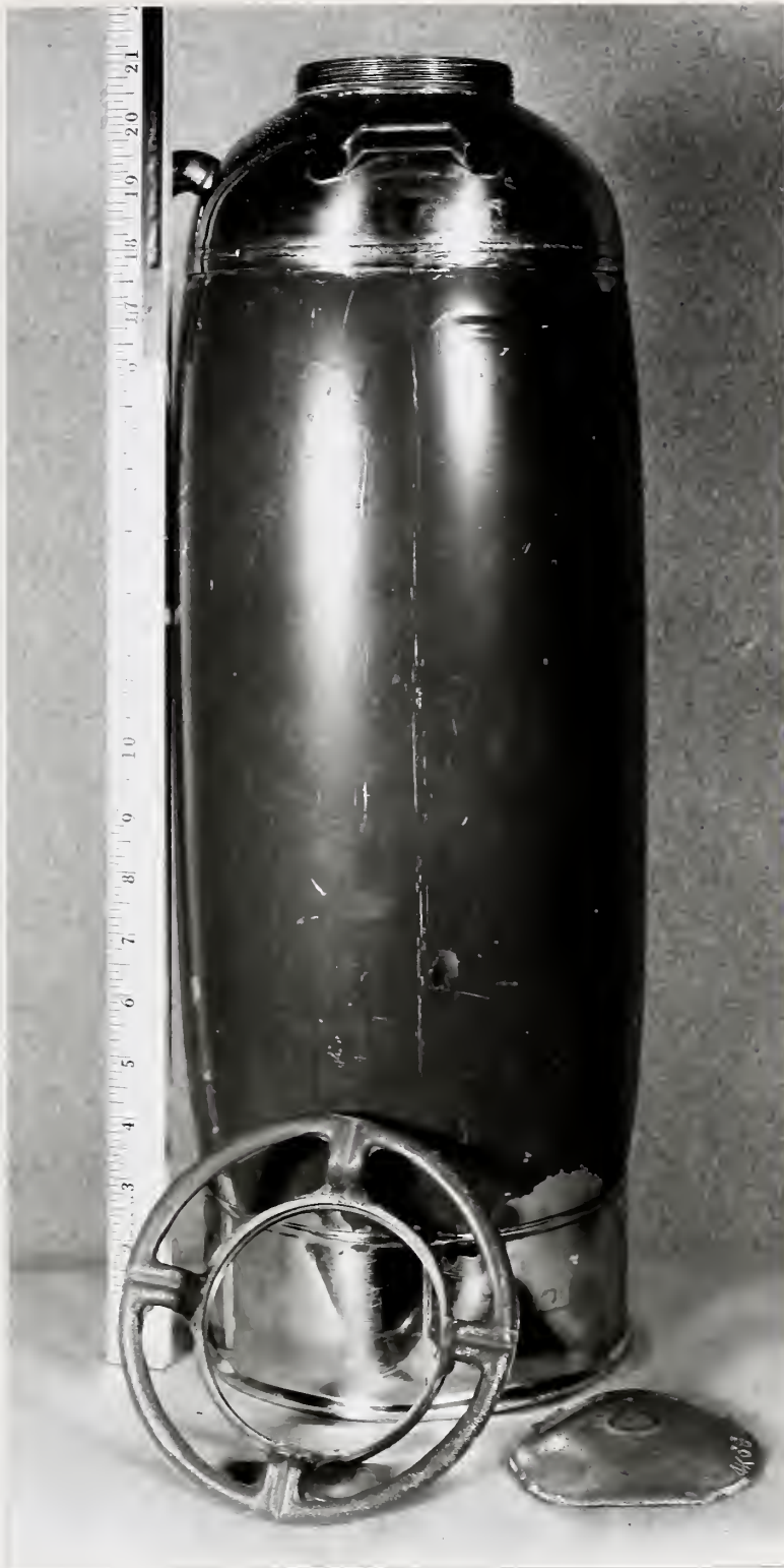
Figure 18. Fire extinguisher number F 701019 pressurized to burst. The extinguisher bulged significantly, but remained structurally intact. Failure occurred at 850 psig when the center section of the cap blew out.
