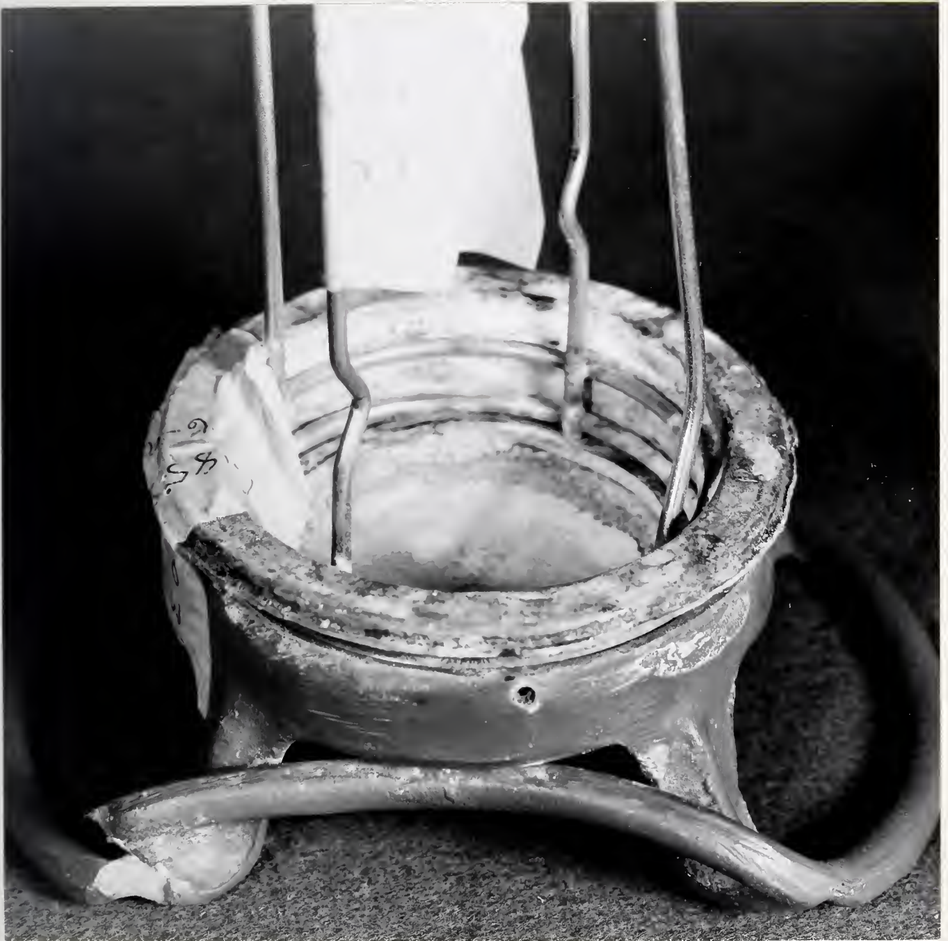
Figure 2c. Inside view of the cap-collar assembly, showing the collar and some of the fracture surface of the dome metal. Note the white substance, which is probably sodium bicarbonate. X 1 1/4
