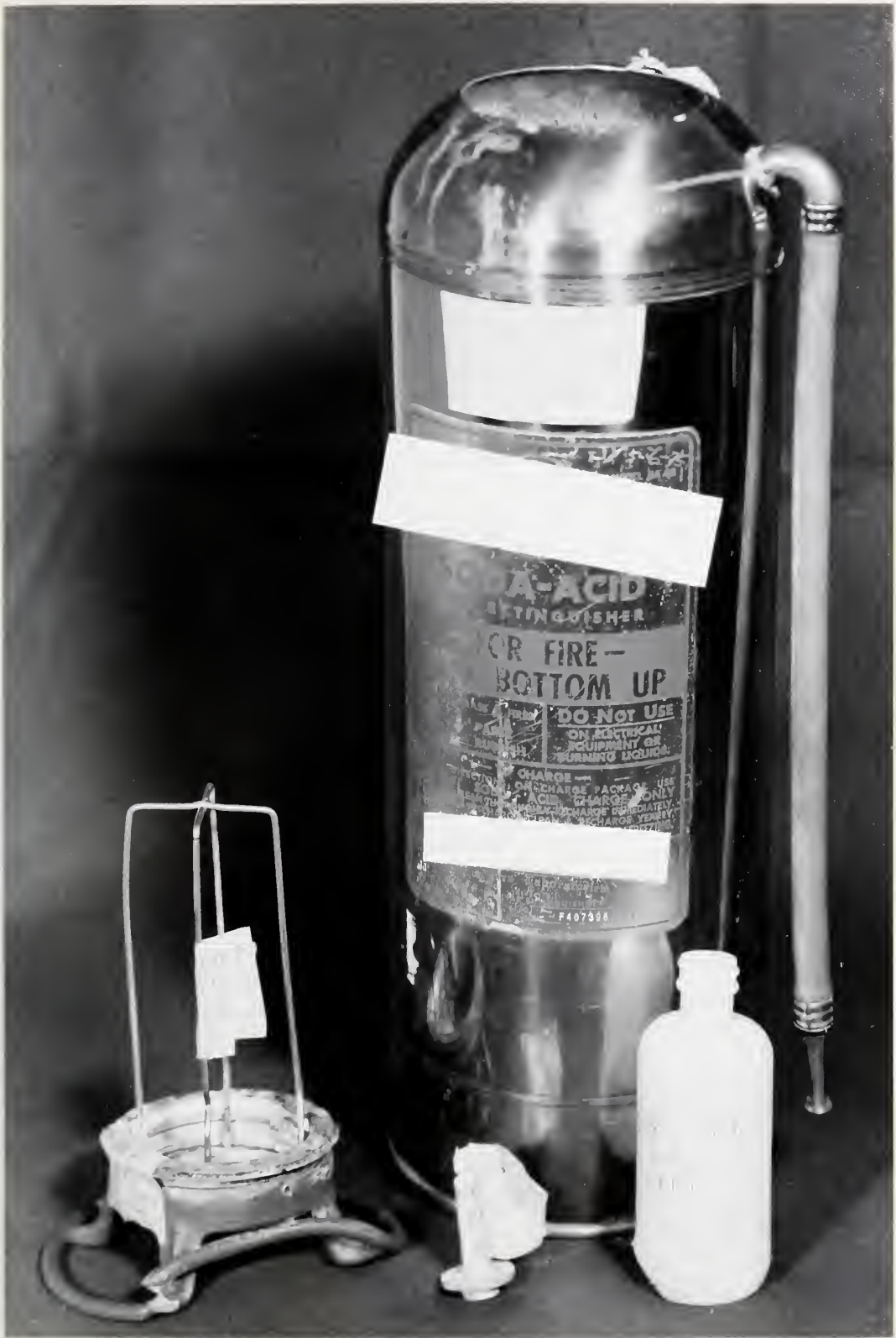
Figure 1. View of the fire extinguisher which exploded. The cap and collar assembly at lower left separated from the dome via a circumferential tear. The acid bottle is positioned with the stopple-end up in the wire cage attached to the cap-collar assembly when the extinguisher is ready for service. Note the identifying number stamped on the lower part of the label. X 1/3
