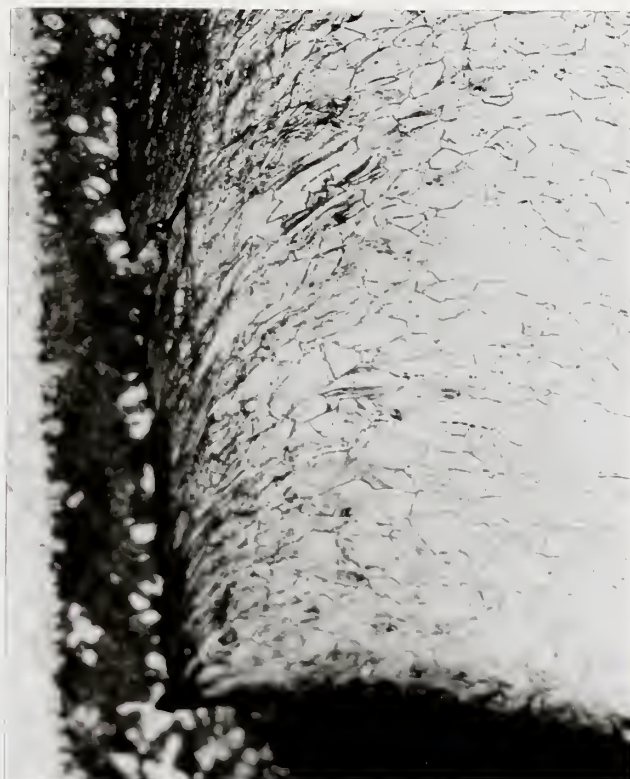
Figure 9a. End of the dome metal under the outside fillet of joining metal. Note severely distorted grains at end indicating localized distortion.
