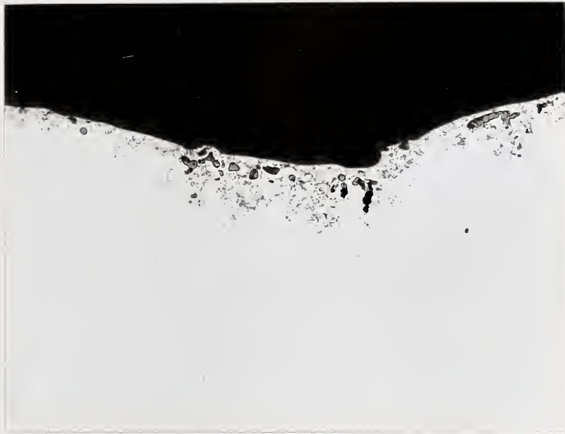
Figure 16. A section of the joining metal near C in Figure 8, showing film of corrosion product.
