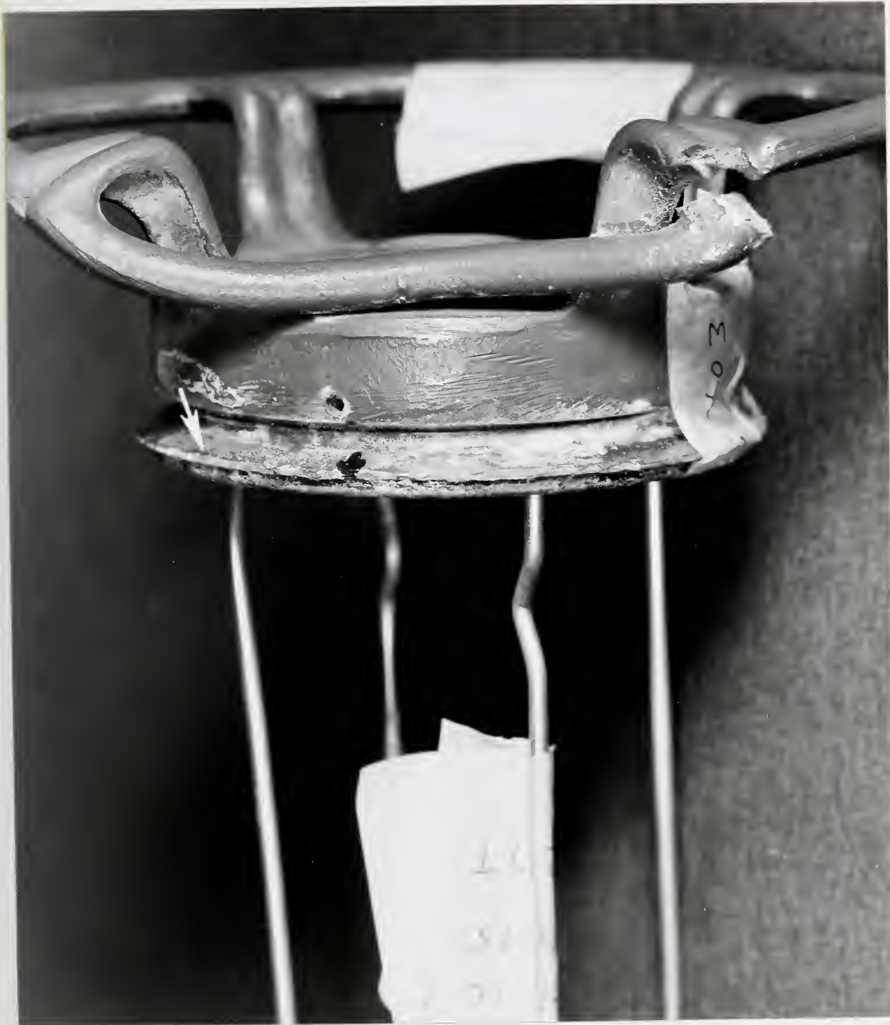
Figure 2b. Close up of the view in Figure 2a. The hole in the cap facilitates venting during filling for hydrotesting. X 1 1/4
