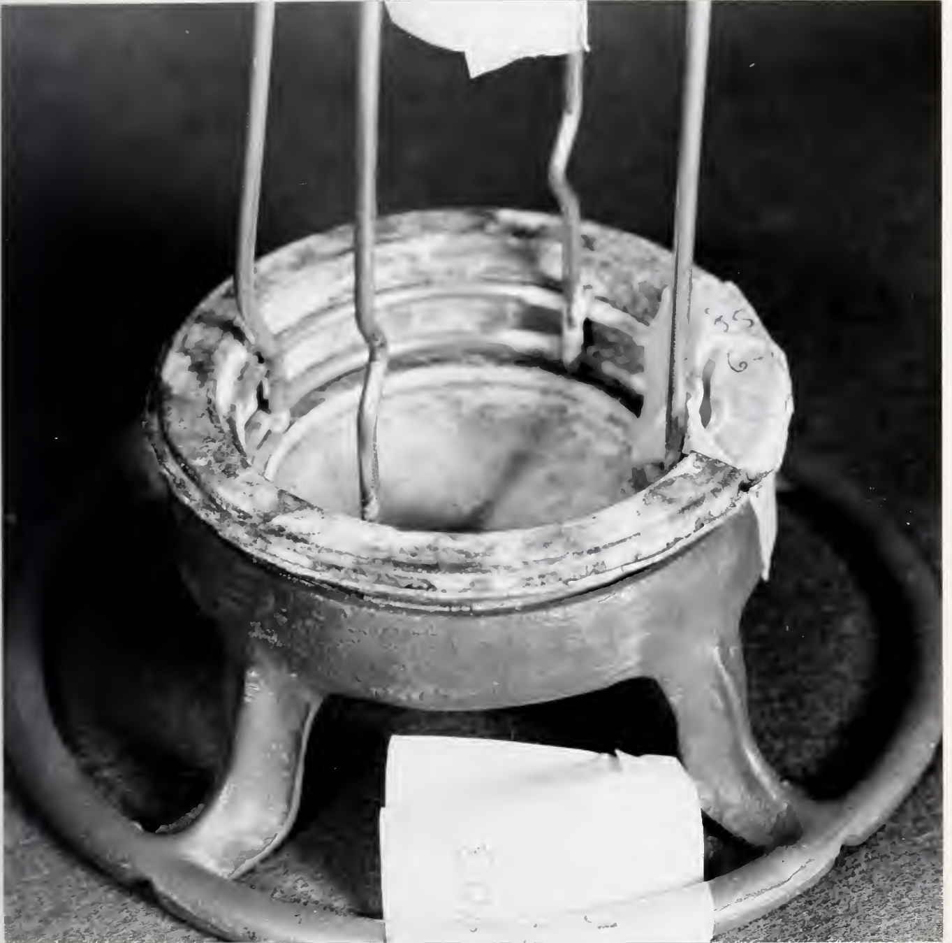
Figure 2d. View of the cap-collar assembly almost opposite that shown in Figure 2c, showing more of the fracture of the dome metal. X 1 1/4
