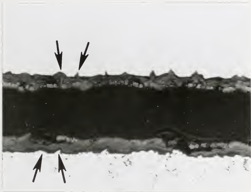
Figure 11. Close-up of the crevice between dome metal (top) and joining metal (bottom) at some point between A and B in Figure 8. Note the good matching of the profiles of the dome metal and the joining metal at the arrows.
