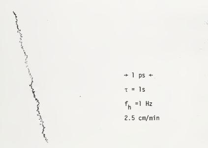
Warm up phase drift was about 50 ps over the first hour; but stabilizing to a peak of about 10 ps thereafter in an overnight run with  $\pm$  2° C ambient temperature fluctuations.
