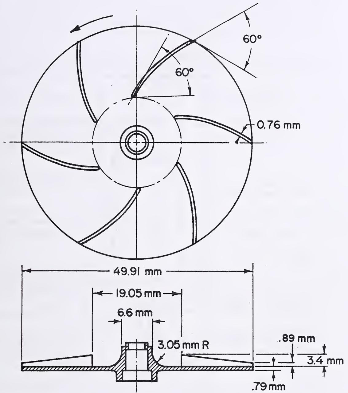
Figure 15. Centrifugal impeller for helium pump.
