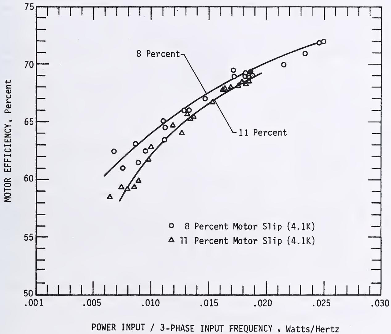
Figure 10. Induction motor efficiency, 8 and 11 percent slip.
