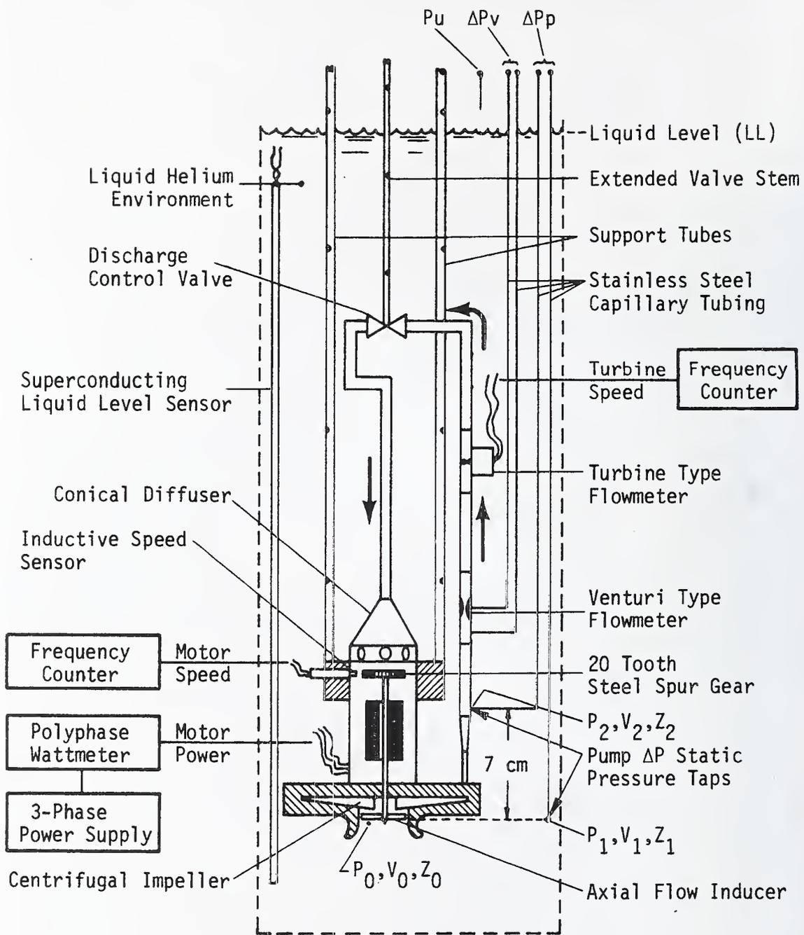
Figure 16. Helium pump test loop and instrumentation.
