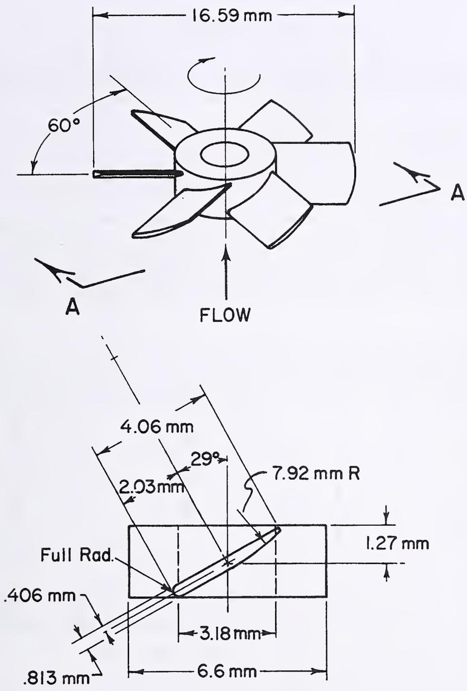
Figure 31. Axial flow inducer.
