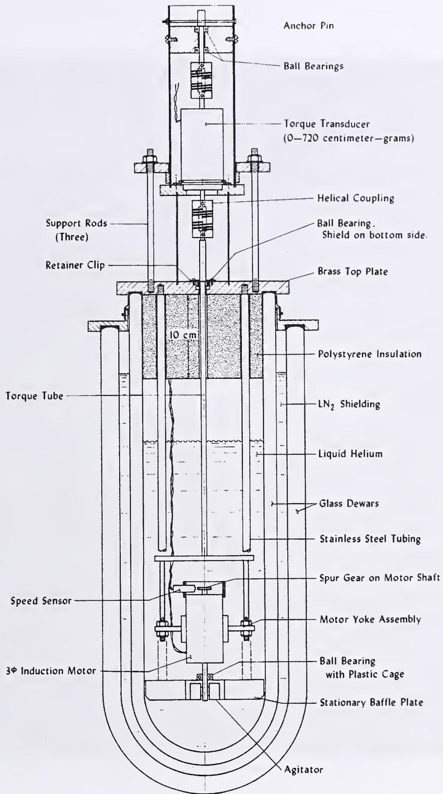
Figure I. Motor Efficiency Test Apparatus
