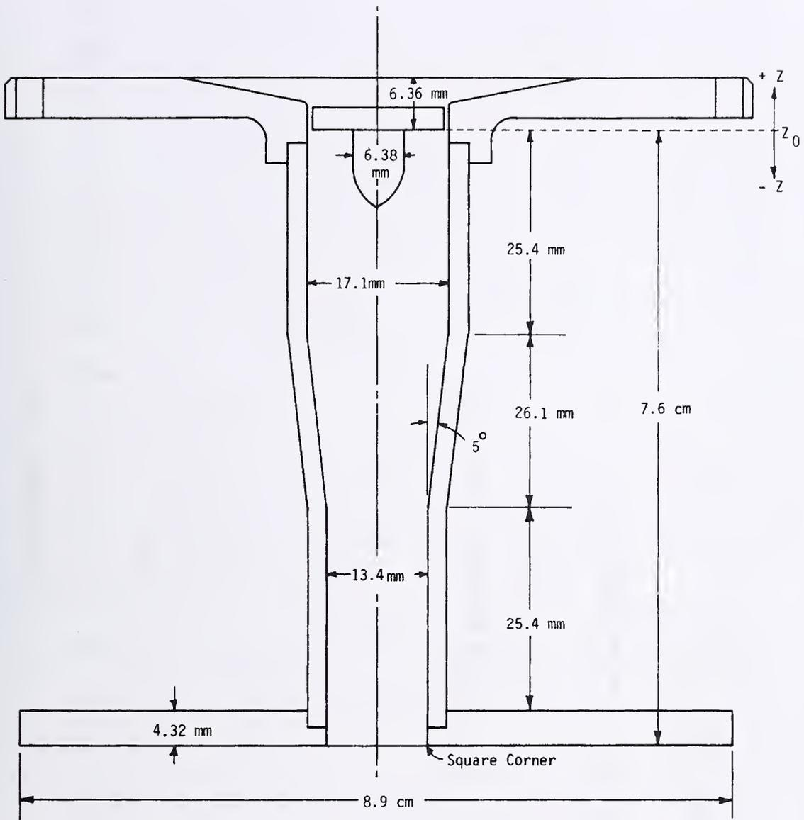
$Z_0$  is the arbitrary pump datum plane for all cavitation data.
