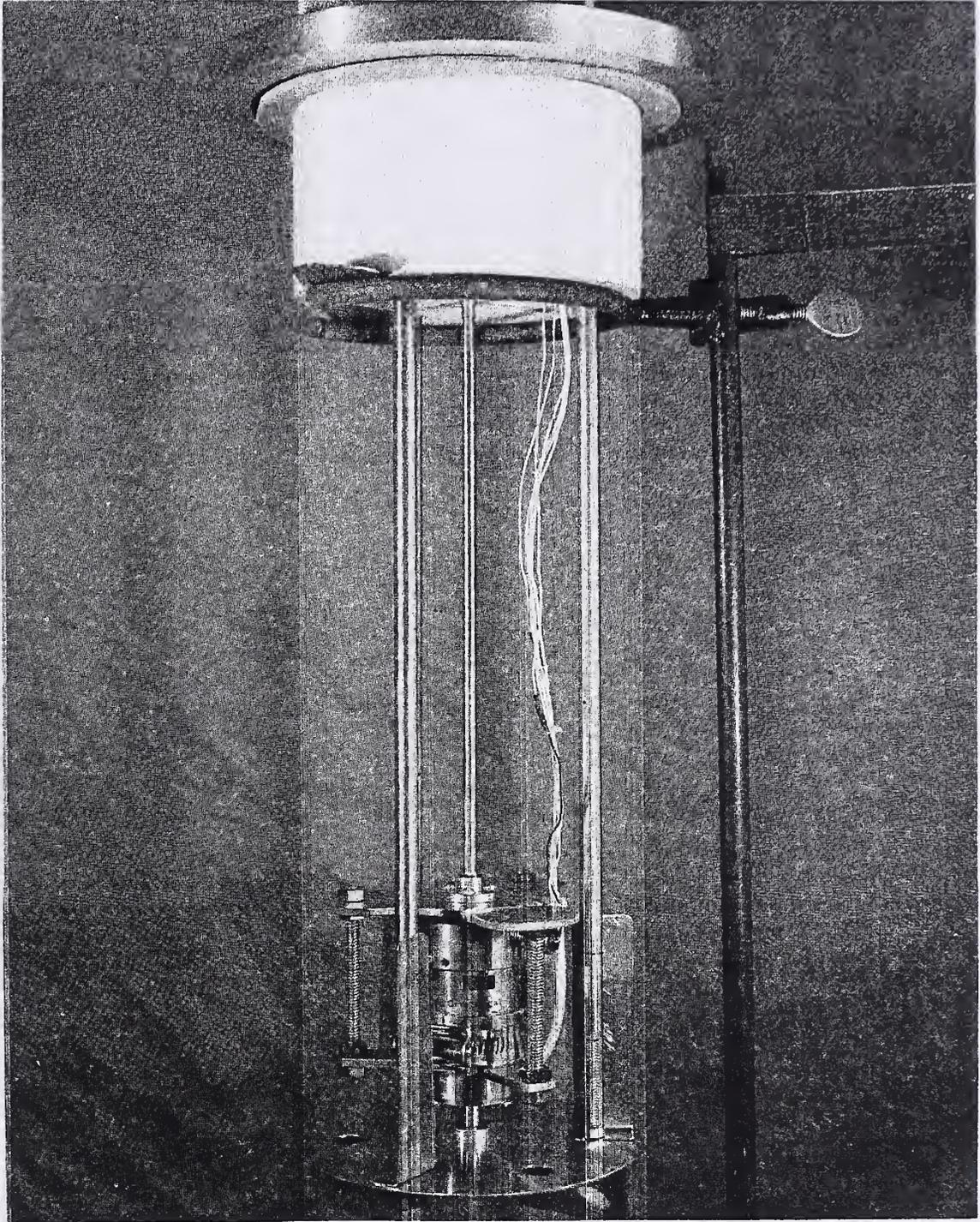
Figure 3. Photo, motor efficiency test apparatus.
