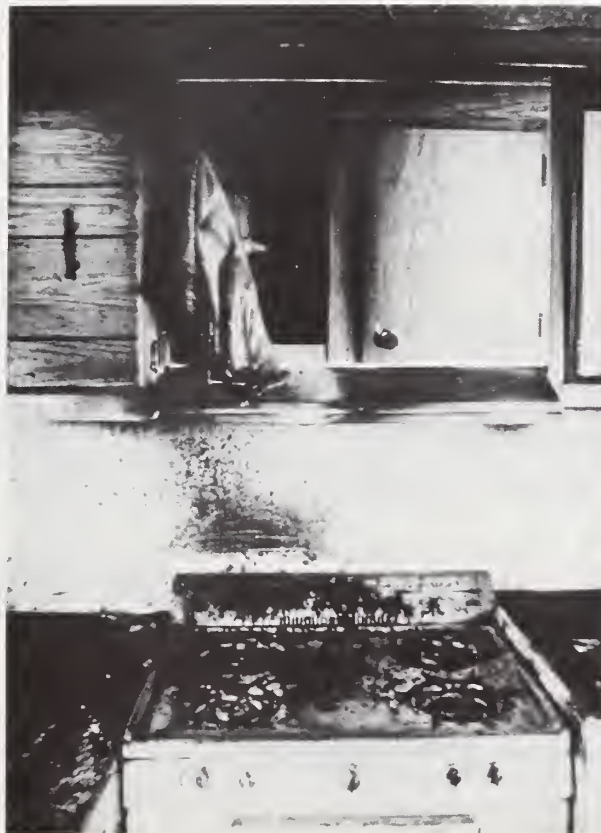
Figure 11. Illustrates the Performance of a Molded Polystyrene Cabinet Door (left) and a Printed Particle Board Cabinet Door (right) to a Test Fire. In this Test a Metal Range Hood was Installed.
