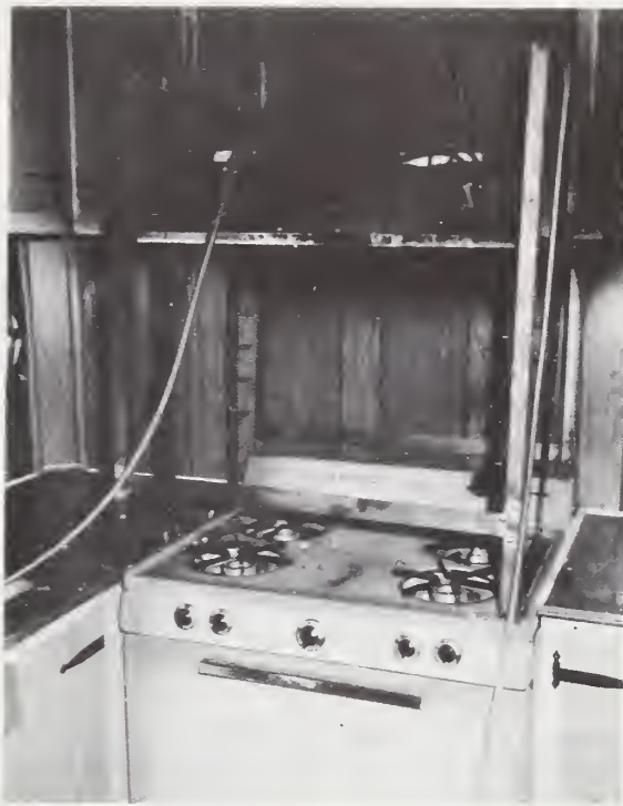
Figure 5. Test Apparatus for Measuring Incident Heat Flux
