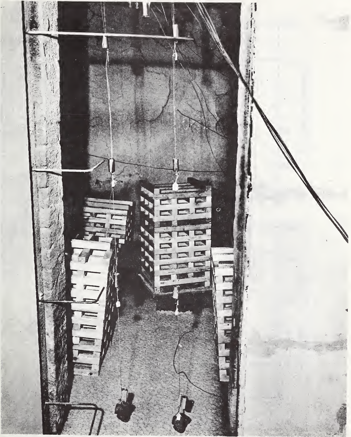
Figure 5. View in Burn-Room Door Showing Wood Cribs. Center Crib on Load Cell. Thermocouples and Pitot Tubes in Doorway.
