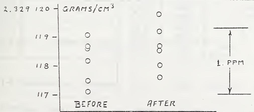
FIGURE 3. MEASURED VALUES OF THE DENSITY OF SILICON CRYSTAL DESIGNATED X5 BEFORE AND AFTER ETCHING. FROM THIS DATA WE CONCLUDE THAT OUR MEASUREMENTS ARE INADEQUATELY PRECISE TO DEFINE ANY POSSIBLE DENSITY CHANGE.
