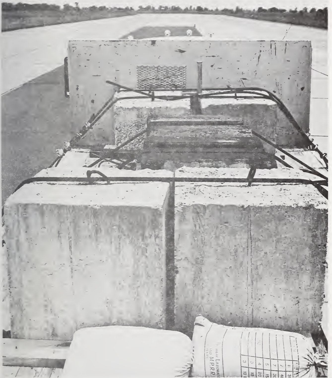
Figure 5. A view of the test vehicle body showing placement of the various weights used to provide tire loading.
