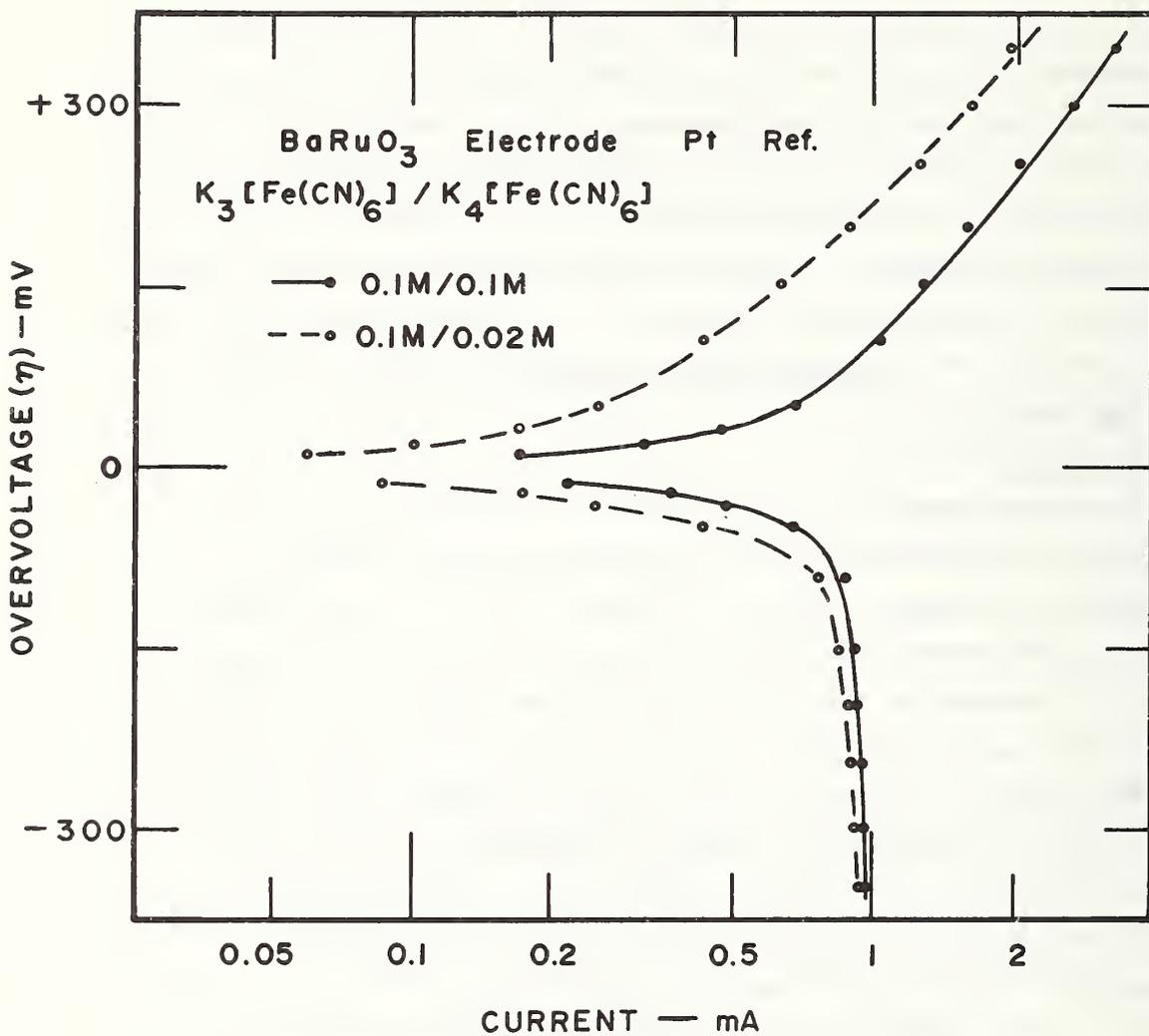
Figure 11. Ferro-ferricyanide reaction. Steady-state performance of Type II BaRuO<sub>3</sub> electrode. Plot of overvoltage versus logarithm of current. M = mol/l.
