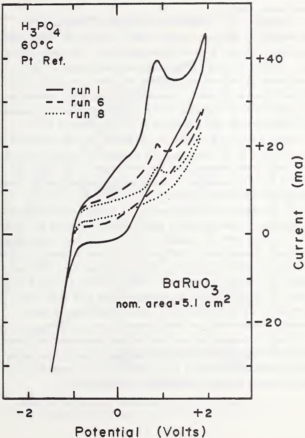
Figure 6. Current-potential curves for a Type II  $\text{BaRuO}_3$  electrode in concentrated phosphoric acid at  $60^\circ\text{C}$ . The decrease in current with time is probably related to dissolution of the sample.
