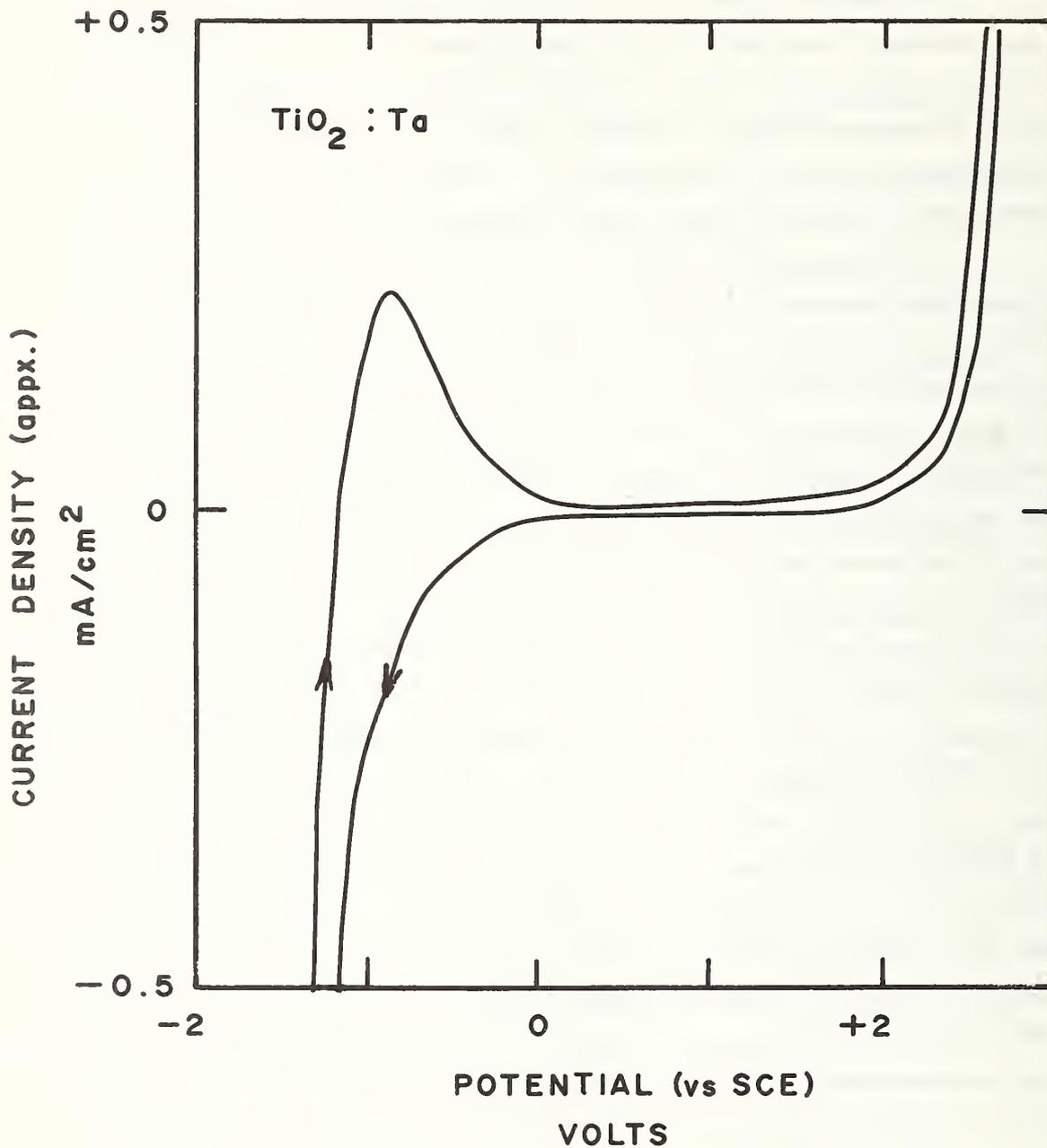
Figure 4. Current-potential curve for 95 TiO<sub>2</sub>: 5 Ta<sub>2</sub>O<sub>5</sub> in 5 mol/l H<sub>3</sub>PO<sub>4</sub> at room temperature. Type I electrode configuration.
