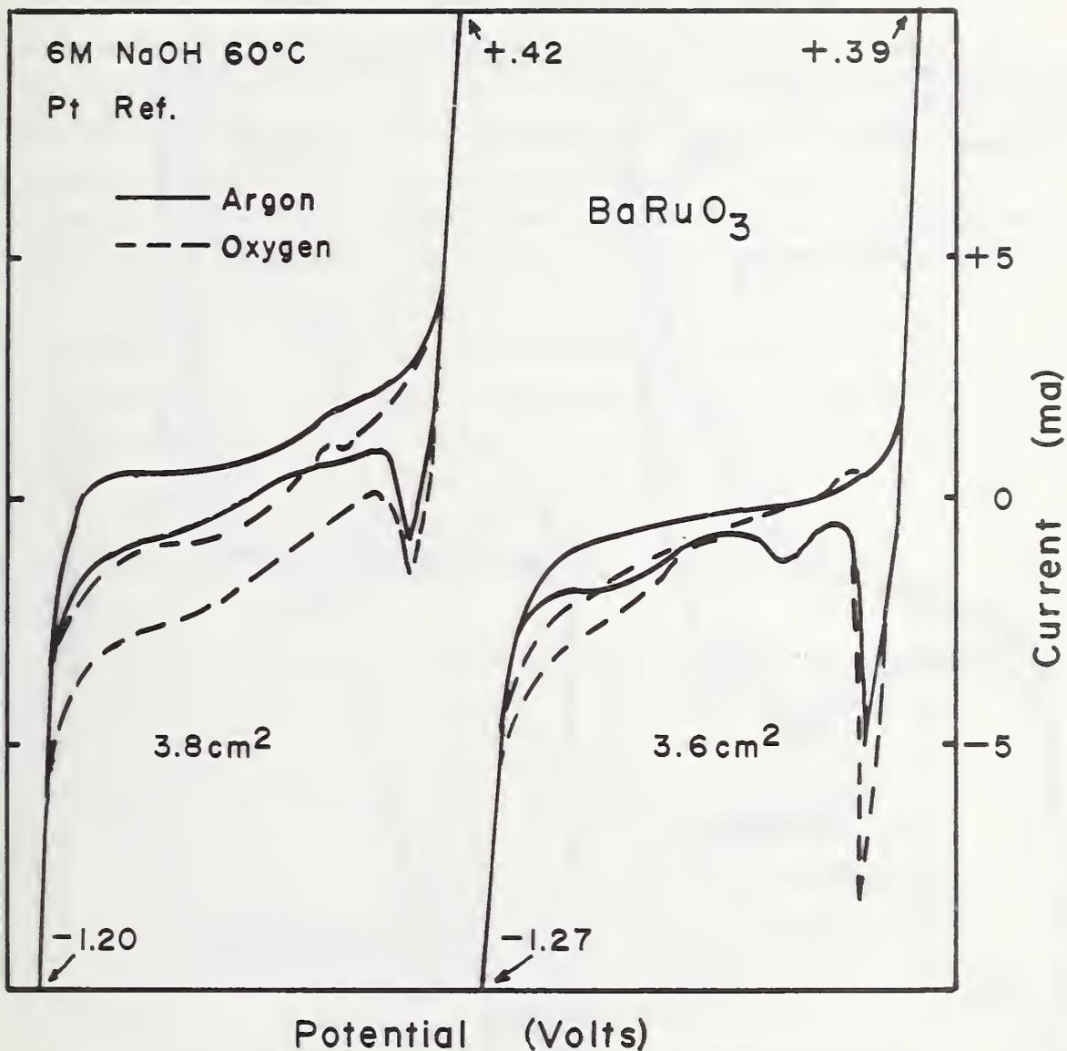
Figure 9. Comparison of two BaRuO<sub>3</sub> electrodes (Type II) in 6 mol/l (=M) NaOH at 60 °C.
