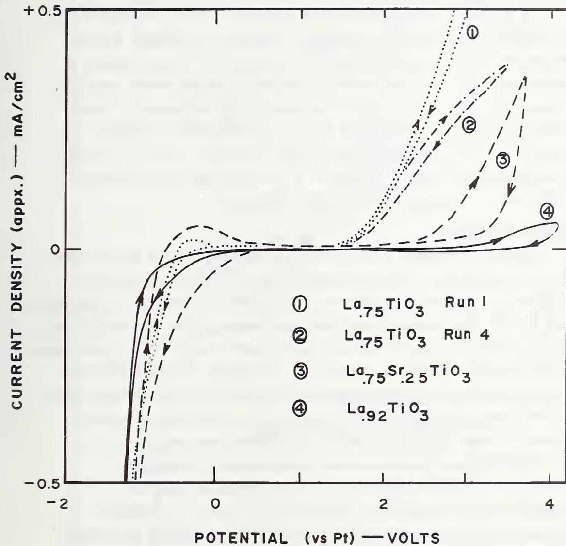
Figure 5. Current-potential curves for the Lanthanum Titanates at room temperature. Type I electrodes in 5 mol/l  $\text{H}_3\text{PO}_4$ .
