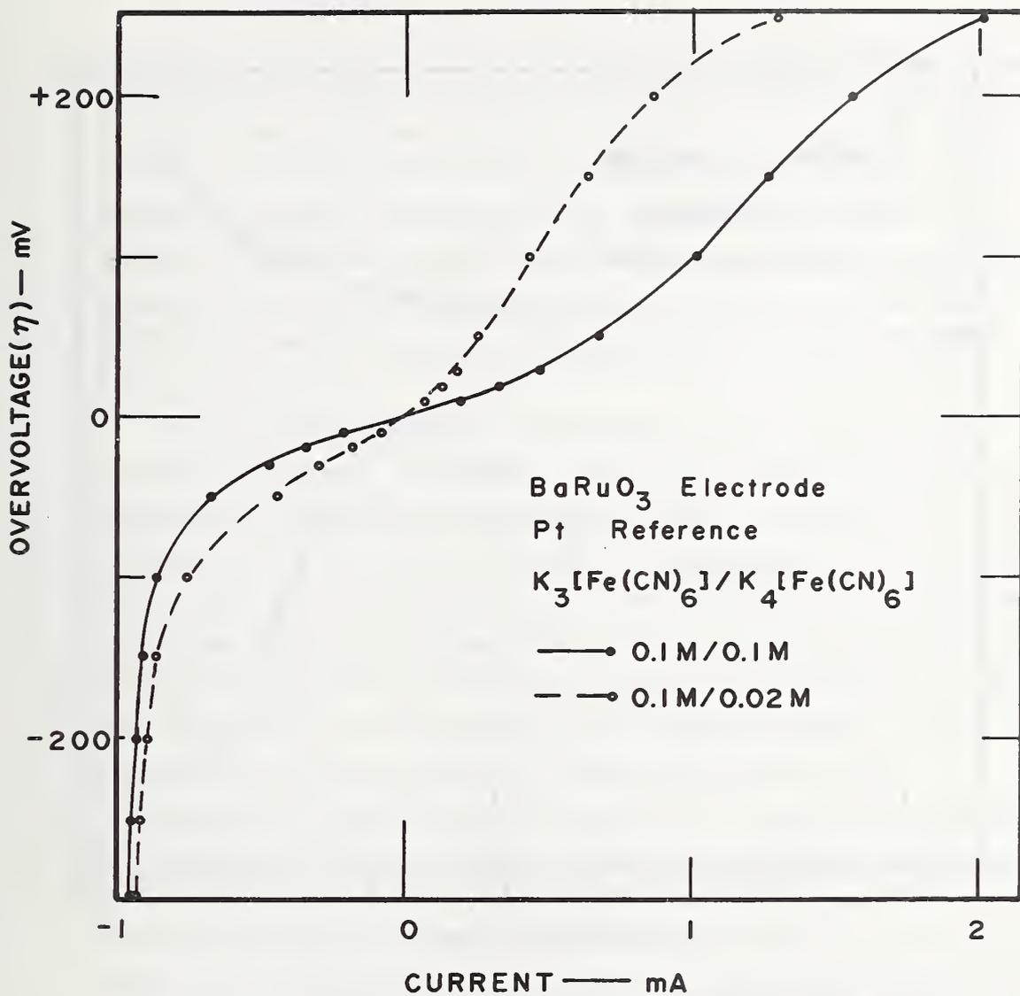
Figure 12. Ferro-ferricyanide reaction. Steady-state performance of Type II. BaRuO<sub>3</sub> electrode. Plot of overvoltage versus current. M = mol/l.
