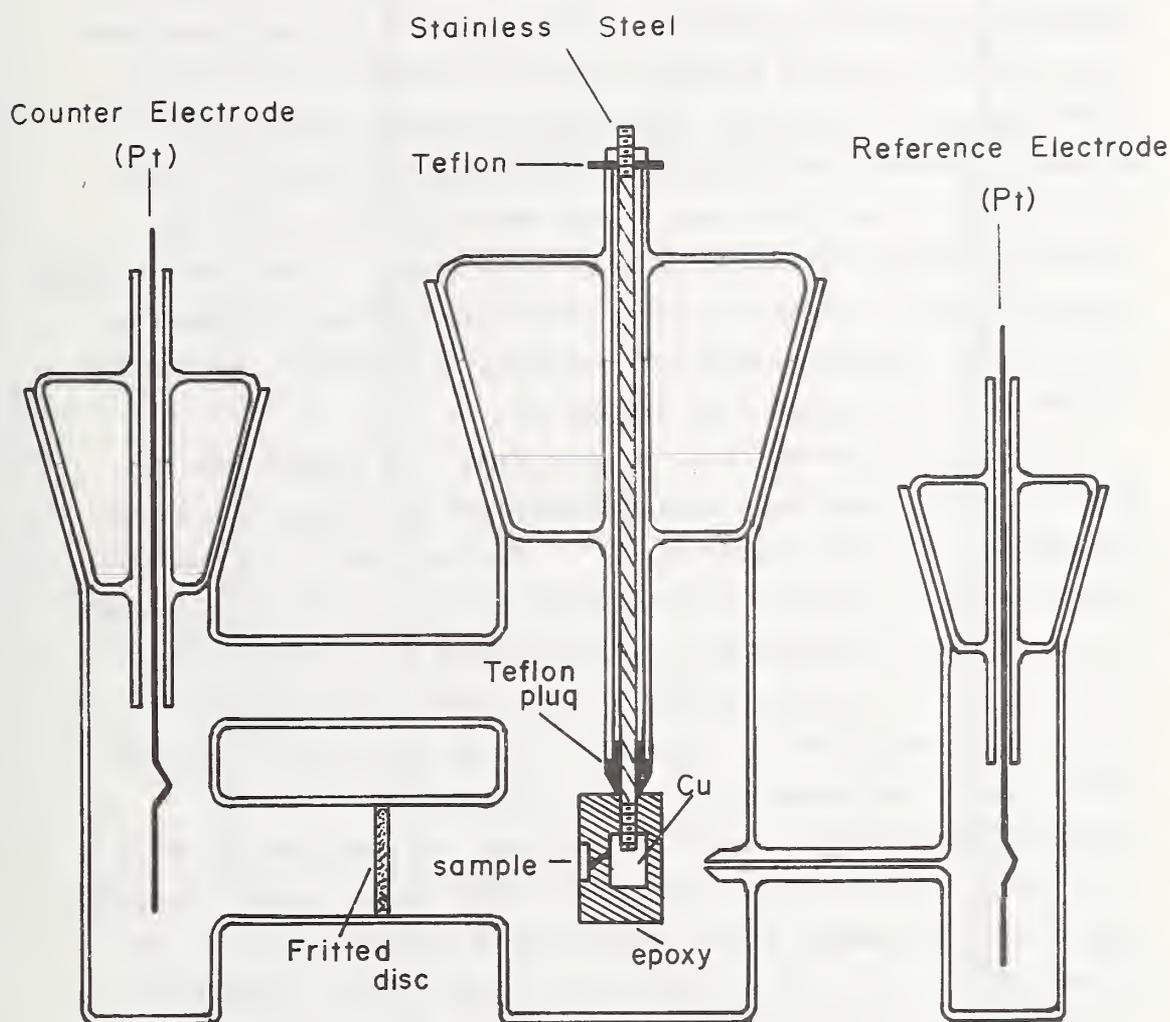
Figure 2. Electrochemical cell used at room temperature with Type I electrodes. This is a cross section of three of the four compartments. Compartment 4, which contains the Calomel reference, is situated behind the compartment for the Pt reference. A type I electrode is also shown in cross section. The heavy black line, connecting sample and Cu block, denotes a Pt wire for electrical contact.
