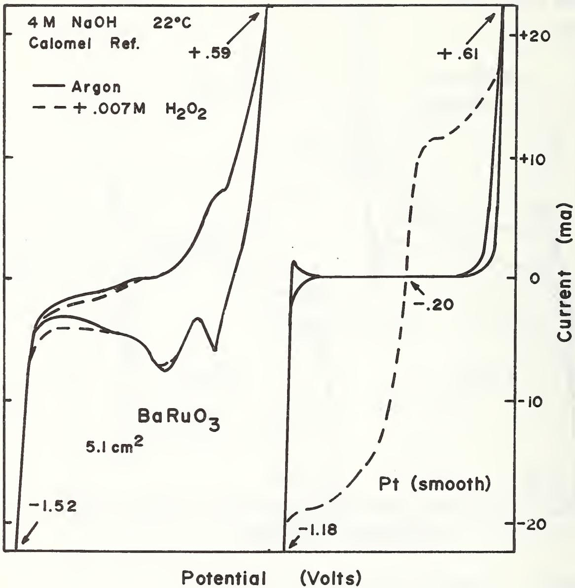
Figure 10. The effect of 0.007 M H<sub>2</sub>O<sub>2</sub> on a Type II BaRuO<sub>3</sub> and on smooth Pt.
