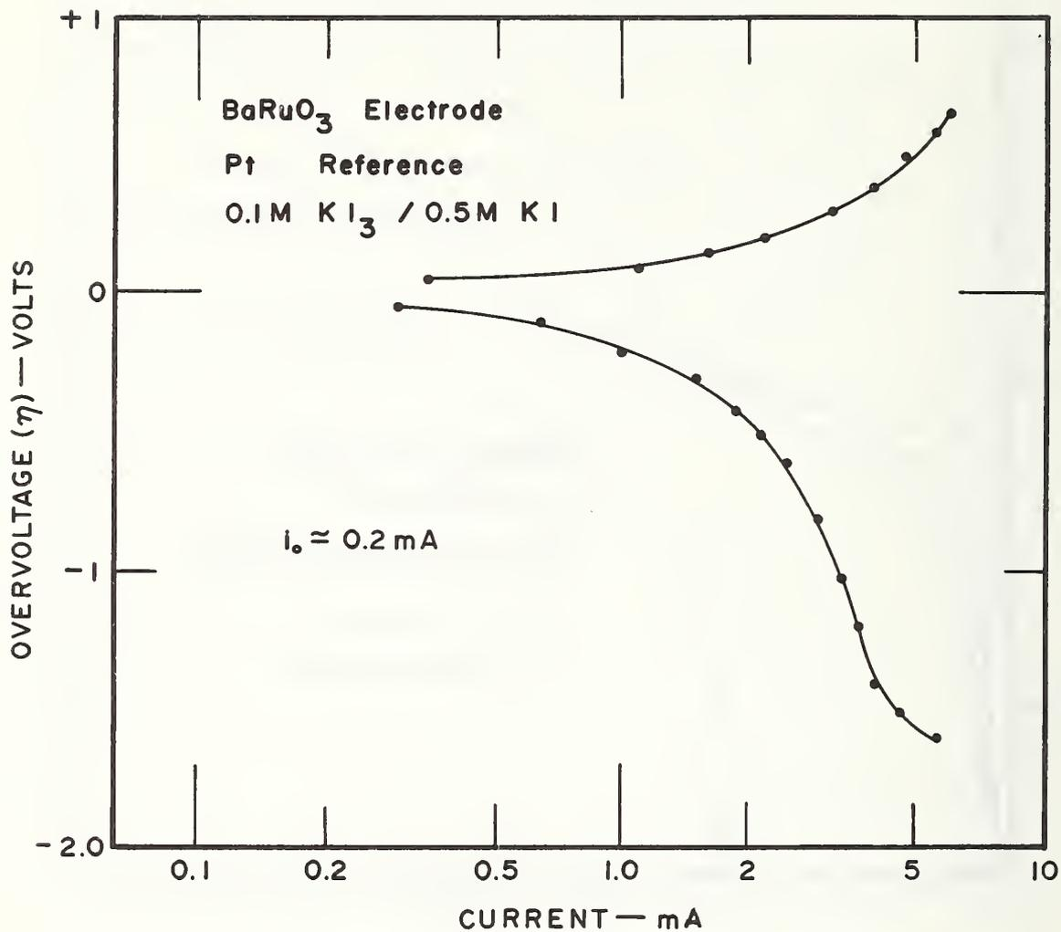
Figure 13. Iodine-iodide reaction. Steady-state performance of Type II BaRuO<sub>3</sub> electrode. Plot of overvoltage versus logarithm of current. M = mol/l.
