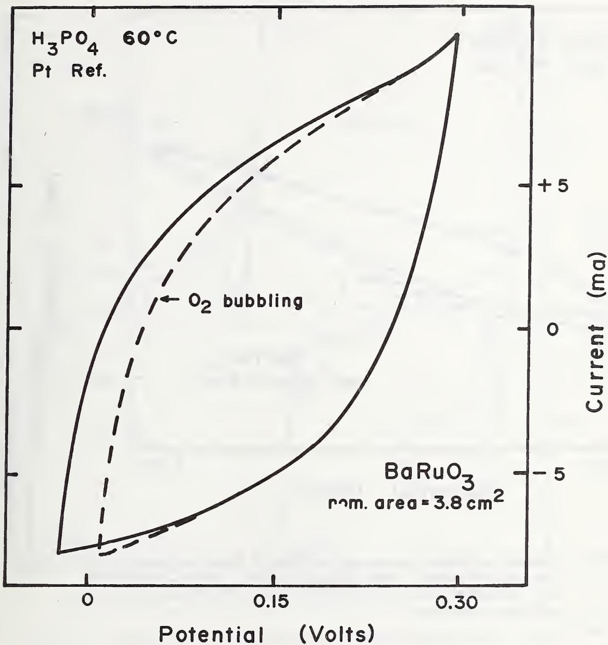
Figure 7. Effect of oxygen and the current-potential curve for a Type II BaRuO<sub>3</sub> electrode.
