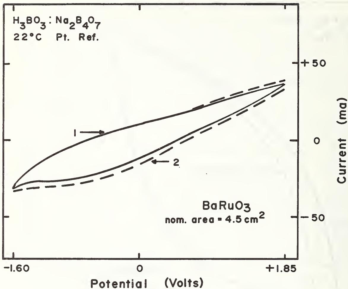
Figure 8. Current-potential curve for a Type II BaRuO<sub>3</sub> electrode in neutral solution. Scan range limited. Curve 1 is for an air saturated electrolyte. Curve 2 is for O<sub>2</sub> bubbling over electrode surface.
