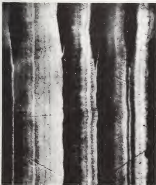
Fig. 1. Photomicrograph of cross section of electroless nickel deposit. Knoop indentations were made for indexing purposes.
