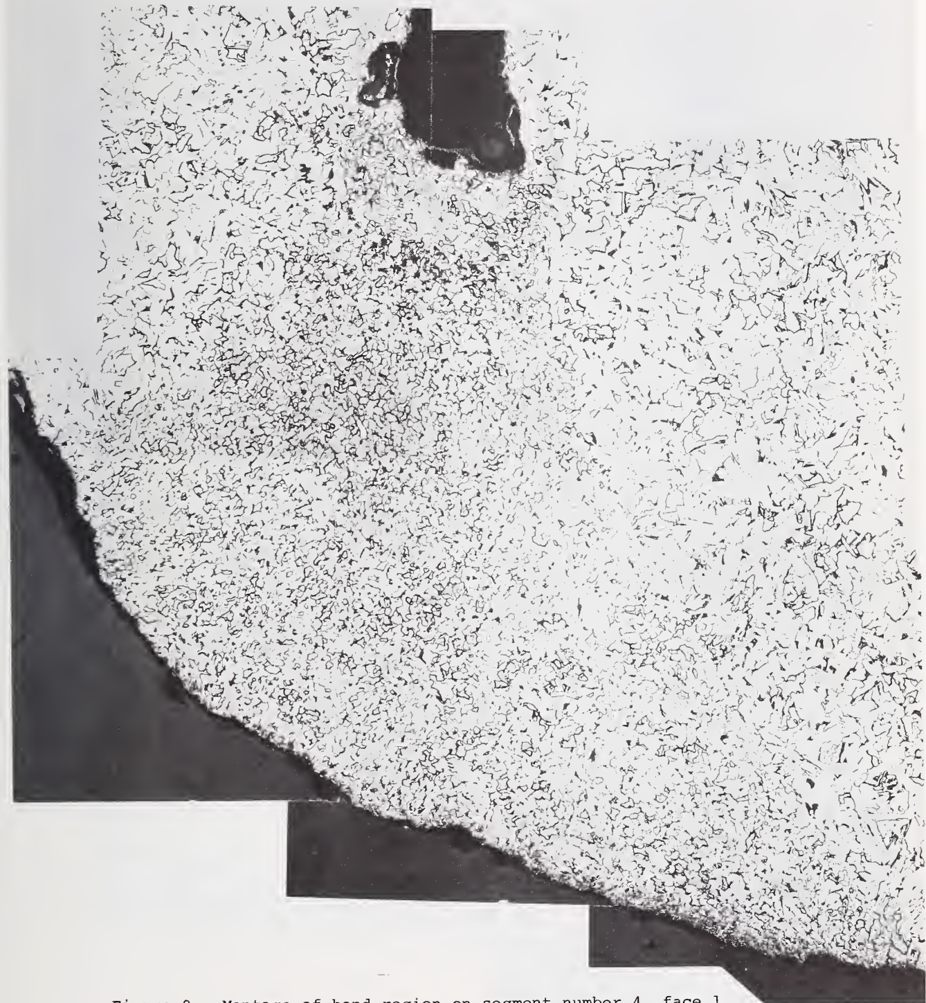
Figure 8. Montage of bond region on segment number 4, face 1. X 40
