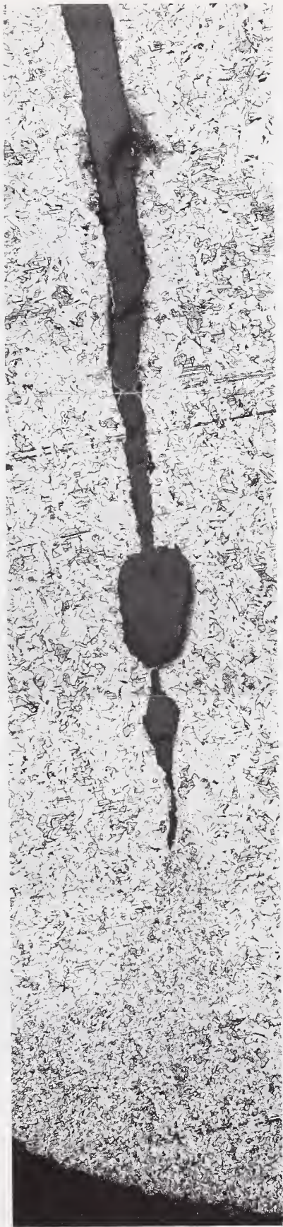
Figure 7. Montage of bond region on segment number 2, face 1. X 40
