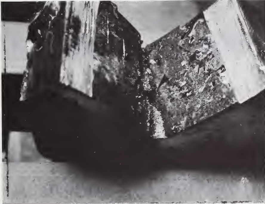
Figure 10. Segment number 5 after being wedged open to examine for cracks, showing the location of a dark region (at the arrow) which represents a possible pre-existing path through the tac weld.
