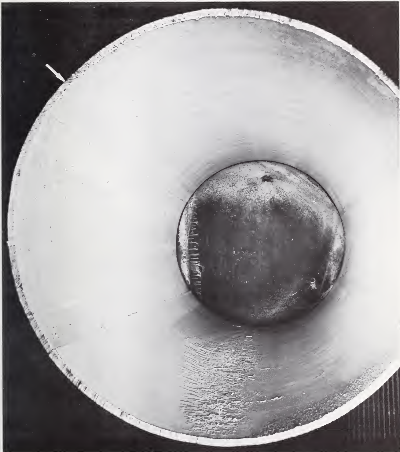
Figure 6. Inside of tank after removal of the end that leaked. The arrow marks a faint corrosion line located at saw-cut boundary of segments 4 and 5, which were taken from the flame-cut section of the tank. This arrow is also approximately centered on 2 white marks at 9 o'clock and 12 o'clock. These marks show the limits of the flame-cut section.
