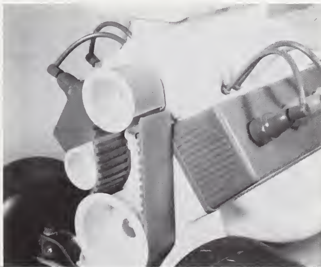
Figure 13. Broken fan belt on RO-43 which occurred during abuse test.
