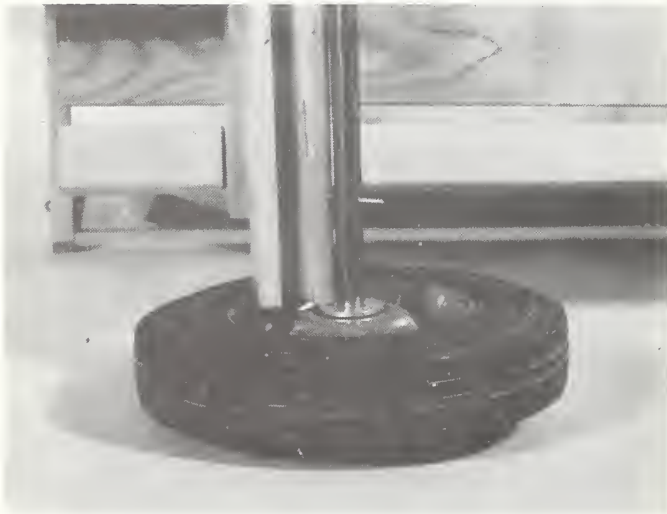
Figure 19. Sharp ends of screws which were exposed after wheel and axle assembly of W-7 pulled loose from wood frame during abuse test.
