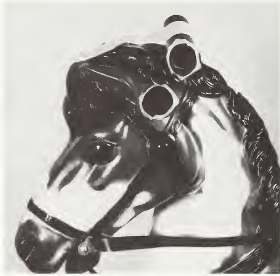
Figure 14. Sharp edges resulting from broken hand grip on RO-45 which occurred during abuse test.
