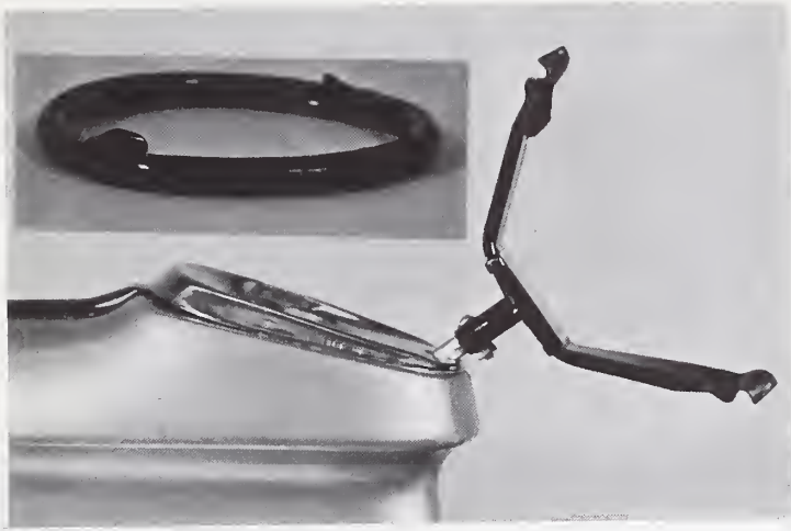
Figure 16. Jagged edges of metal steering wheel broken from R0-59 during abuse test.
