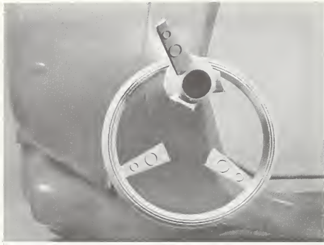
Figure 18. Sharp edges exposed when steering wheel of RI-11 broke during abuse test.
