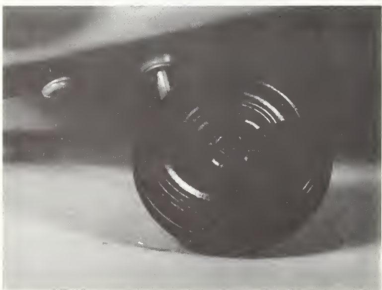
Figure 2b. Rear wheel of RO-29 after collapsing under 18.1 kg (40 lb) test weight during static stability test.
