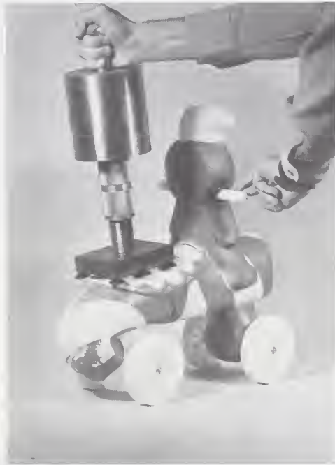
Figure 1. Specimen RO-27 collapsing under 18.1 kg (40 lb) test weight.
