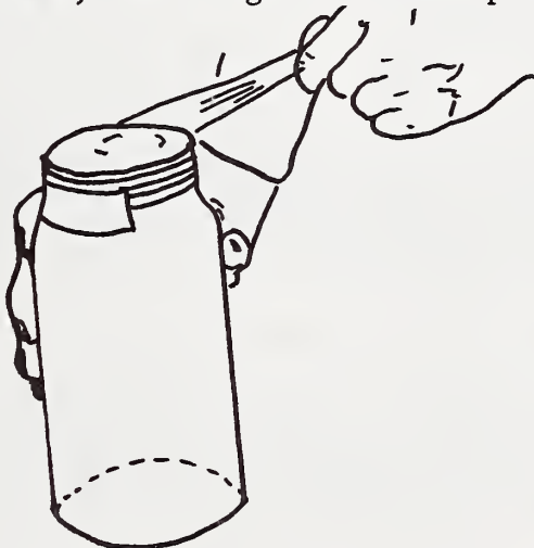
Figure 65. Use of tape as a secondary closure for glass containers.
