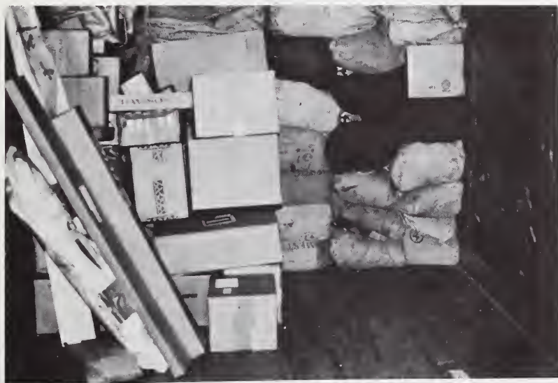
Figure 16. Truck being loaded for transit. (Long parcels are loaded last.)
