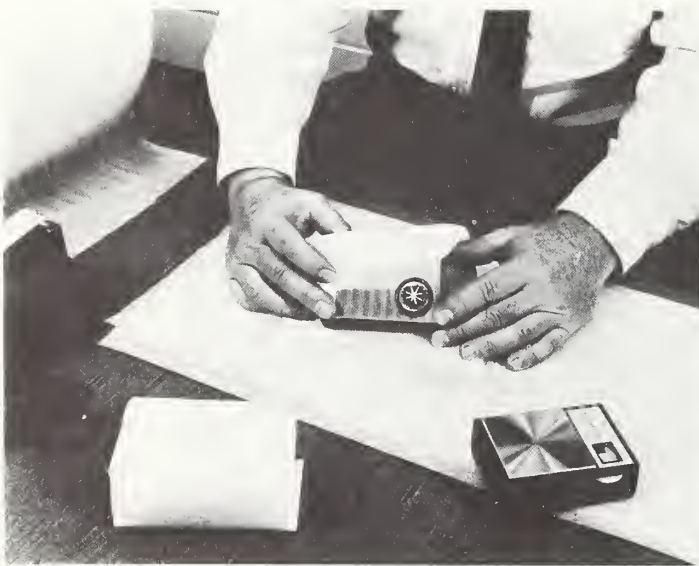
Use of plastic foam sheeting.
