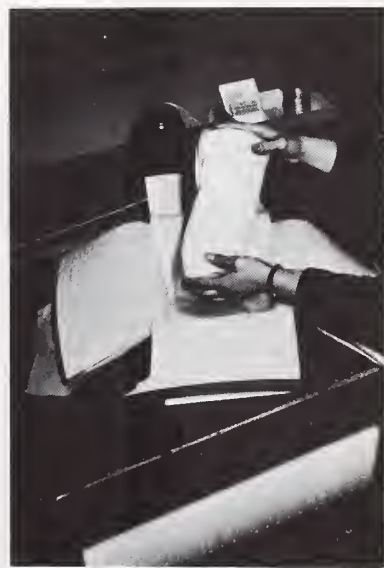
(d) The wrapped and taped product is placed in the lined container.
