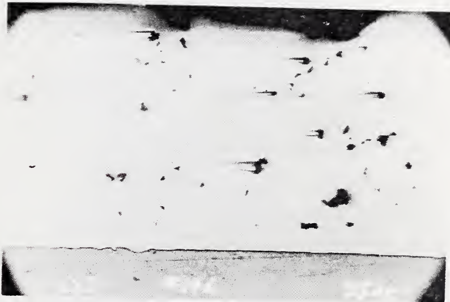
FIGURE 20. Cross-section of deposit made with 1 g/l TlNO_3 added in increments, one-half first then two additions of one-fourth at equal time intervals. Deposit made in 200 g/l CrO_3 bath plus 18 g/l of 15 \mu m nickel coated diamond powder at 55°/50 asd and contained 0.18 wt.% diamond. Original 350X.
