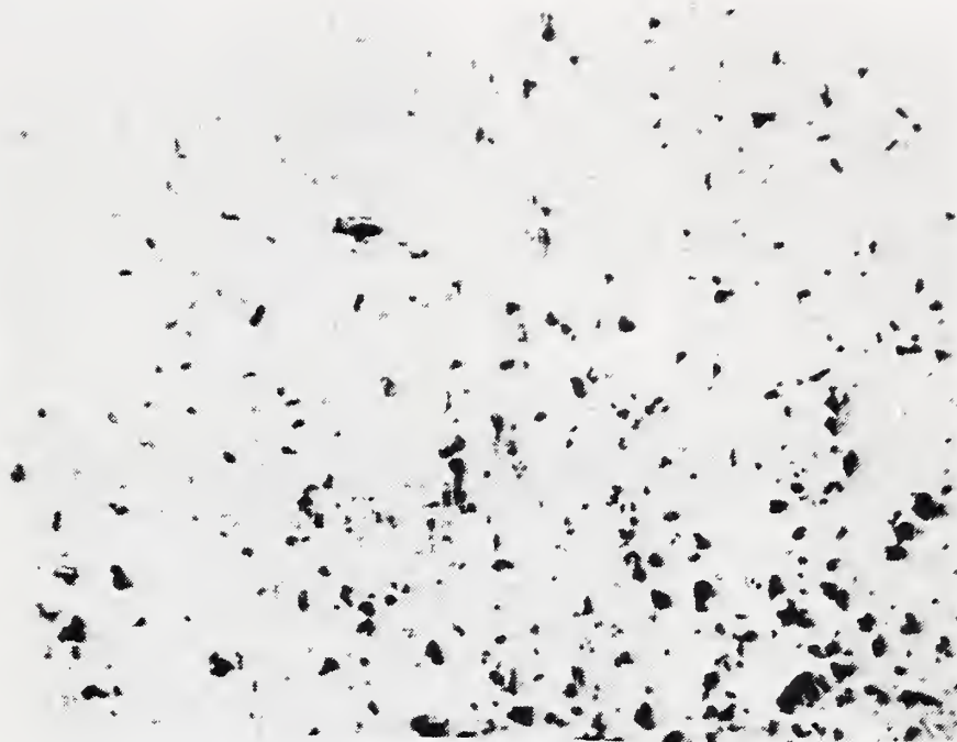
FIGURE 4. Cross-section of deposit that appeared to have inclusion of TiO_2 but gave no positive analytical test for Ti. Dark areas are probably oxides of chromium or small voids in the chromium. Original 550X.
