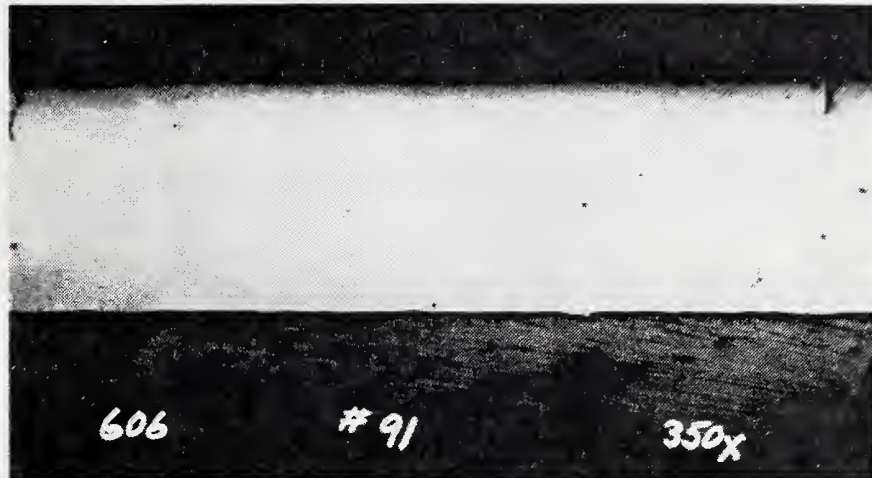
Figure 12 A & B. Cross-sections of similar chromium deposits with (607) and without (606) the addition of 5 g/l of thallium to the bath. Chromium plated from 200 g/l \text{CrO}_3 standard bath at 60^\circ/40 asd. 607 contains 1.5 wt.% diamond powder. Original 350X.
