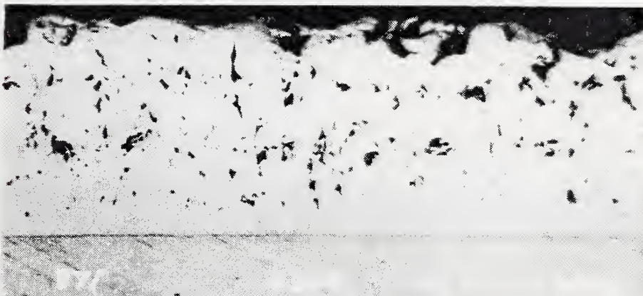
Figure 33. Comparison of effect on structure of 5 g/l \text{LiNO}_3 (top), about 4 g/l \text{NH}_4\text{NO}_3 (center), and 5 g/l \text{TlNO}_3 . Wear for the deposits would be less than for standard chromium. Appreciable inclusions were contained in all, but were loosely held in the discontinuities rather than firmly anchored in the chromium matrix.
