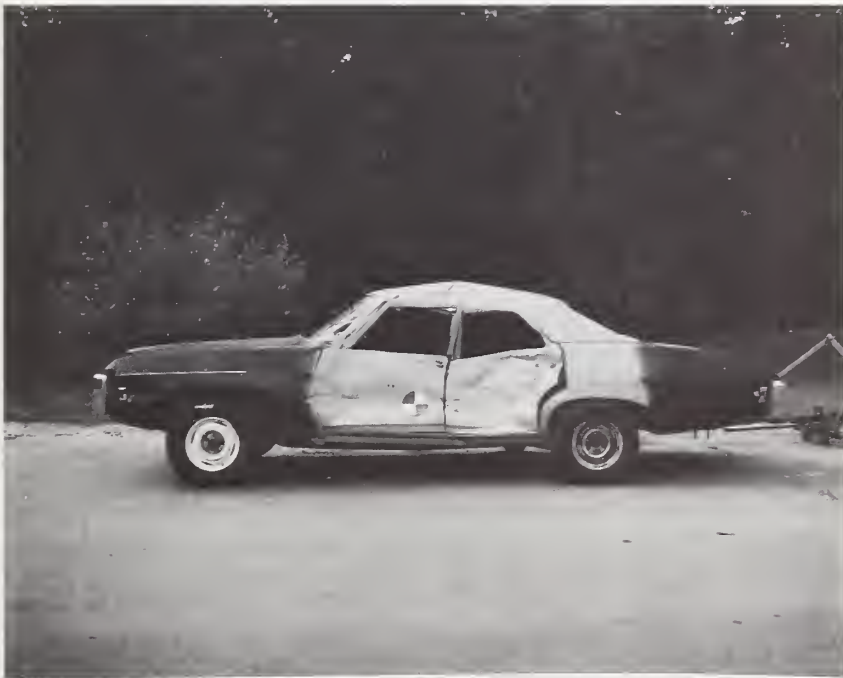
Figure 34 - EXTERNAL SIDE DEFORMATION AFTER STATIC TEST OF VEHICLE "B-1" (UPPER) AND DYNAMIC TEST OF VEHICLE "B-2" (LOWER)
