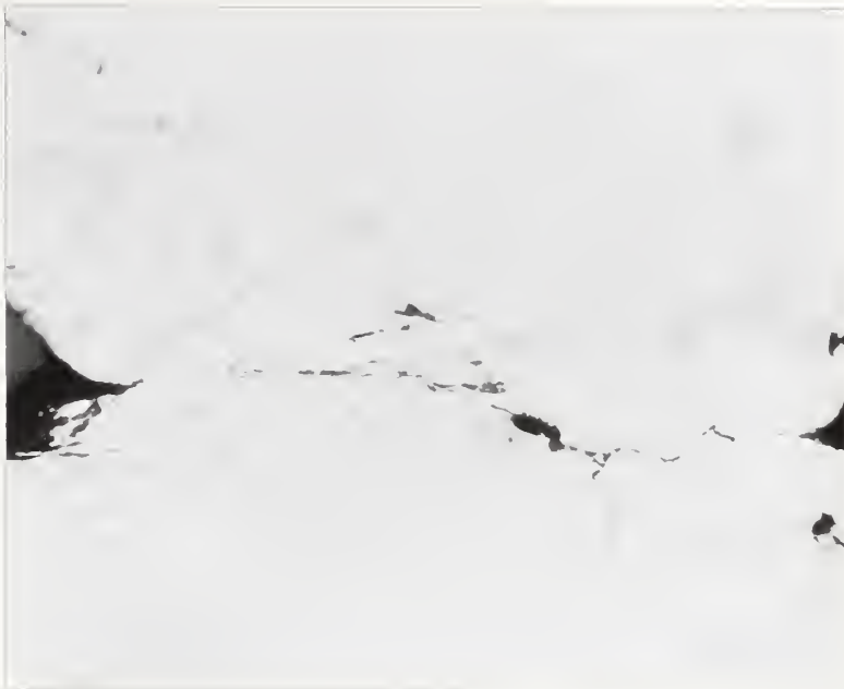
Figure 6. Close-up of near-surface crack appearing in Figure 5a. (Ohio material: Specimen Number 8040-1.)
