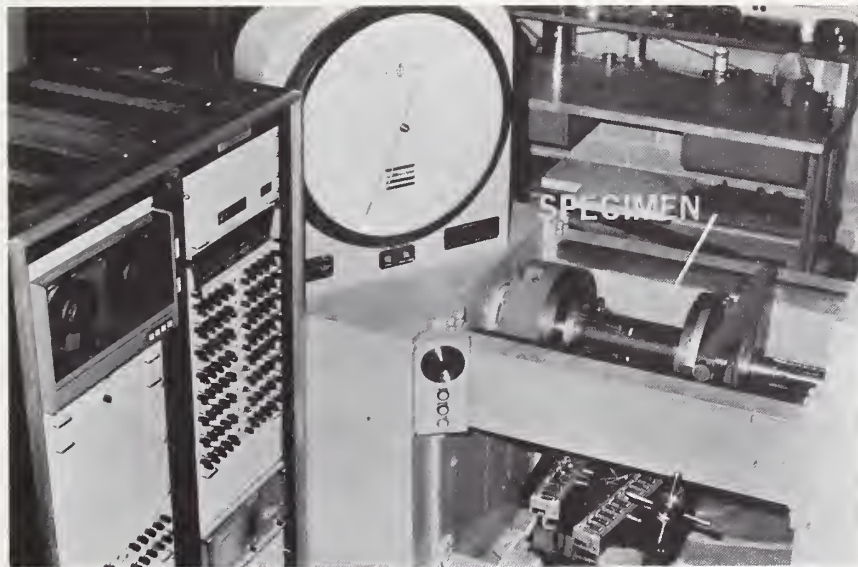
FIG. 6a 40,000 lbf-in TORSION TEST SET-UP
