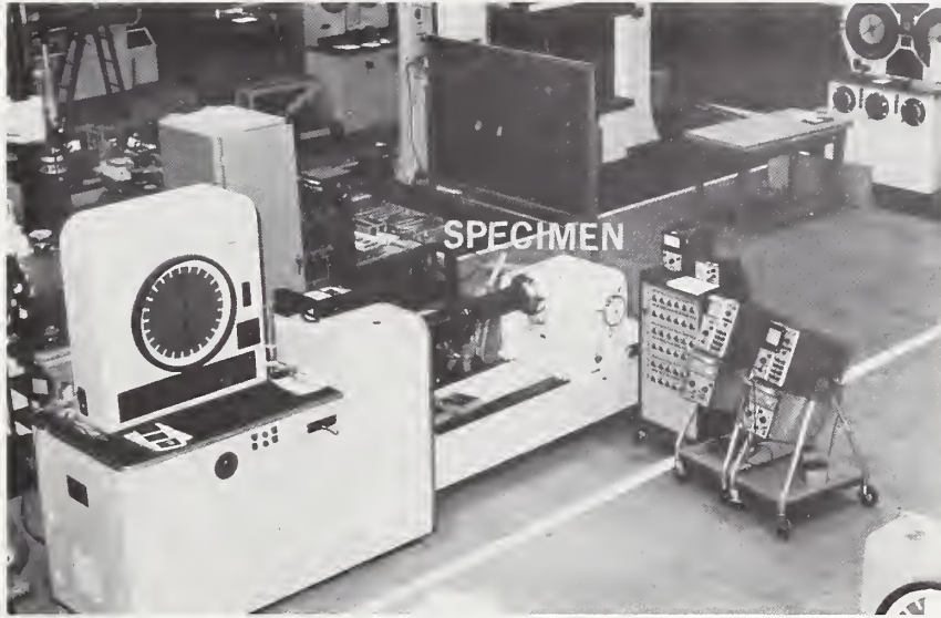
FIG. 6b 60,000 lbf-in TORSION TEST SET-UP
