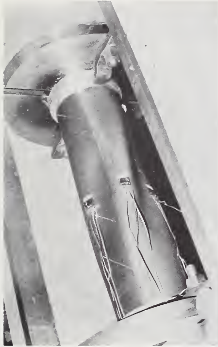
FIG. 8f SPECIMEN BL11 LOADED NEGATIVE
