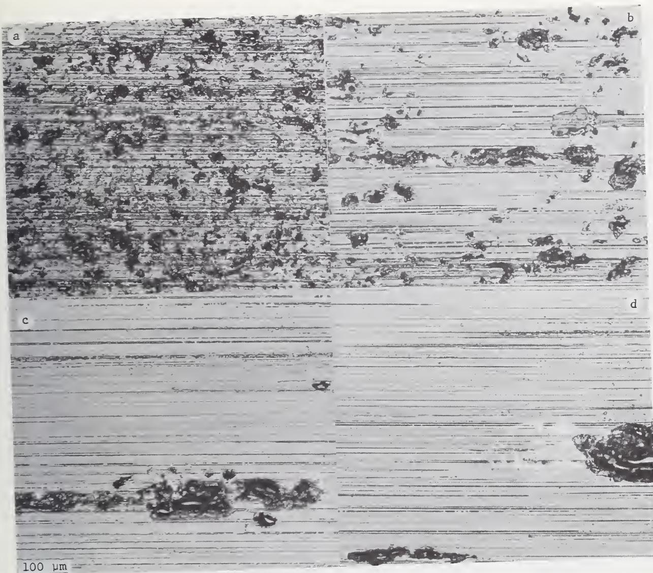
Figure 12. Wear surface of the glass spheres formed by abrasion against the silicon carbide plate. Track changed every 10 seconds to approximate continuous wear. (a) water, (b) butyl alcohol, (c) heptyl alcohol, and (d) dodecyl alcohol.
