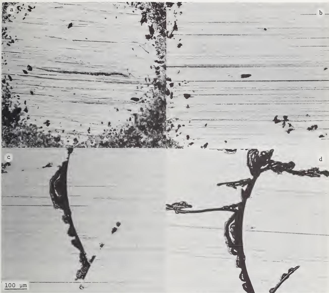
Figure 14. Wear surface formed by abrading the soda lime silicate glass spheres against the silicon carbide plate in decyl alcohol. (a) after ~6 cm of sliding, (b) after ~100 cm of sliding (3 seconds), (c) after ~6000 cm of sliding (5 minutes), (d) same as (c), but etched with H.F. The large curved crack in (c) and (d) was not formed by the abrasion process. Cracks of this sort were frequently observed in the as-received spheres.
