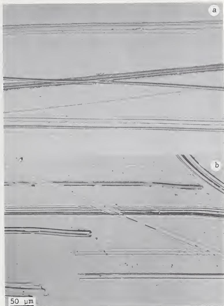
Figure 8. Wear surfaces formed during the first few millimeters of sliding (a) abrasive paper and (b) silicon carbide plate
