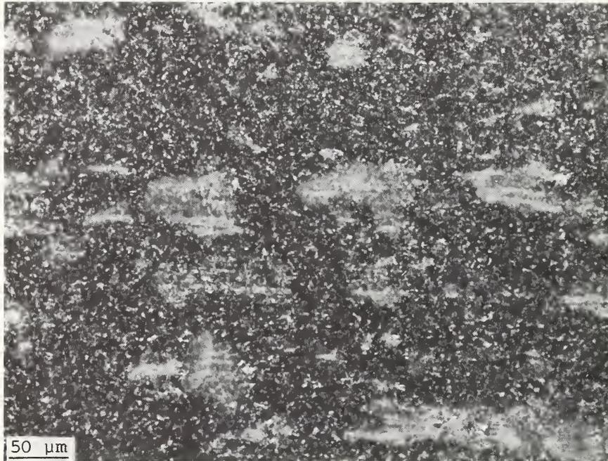
Figure 11. Wear debris formed at the cutting asperities on the silicon carbide plate (ethyl alcohol as lubricant)
