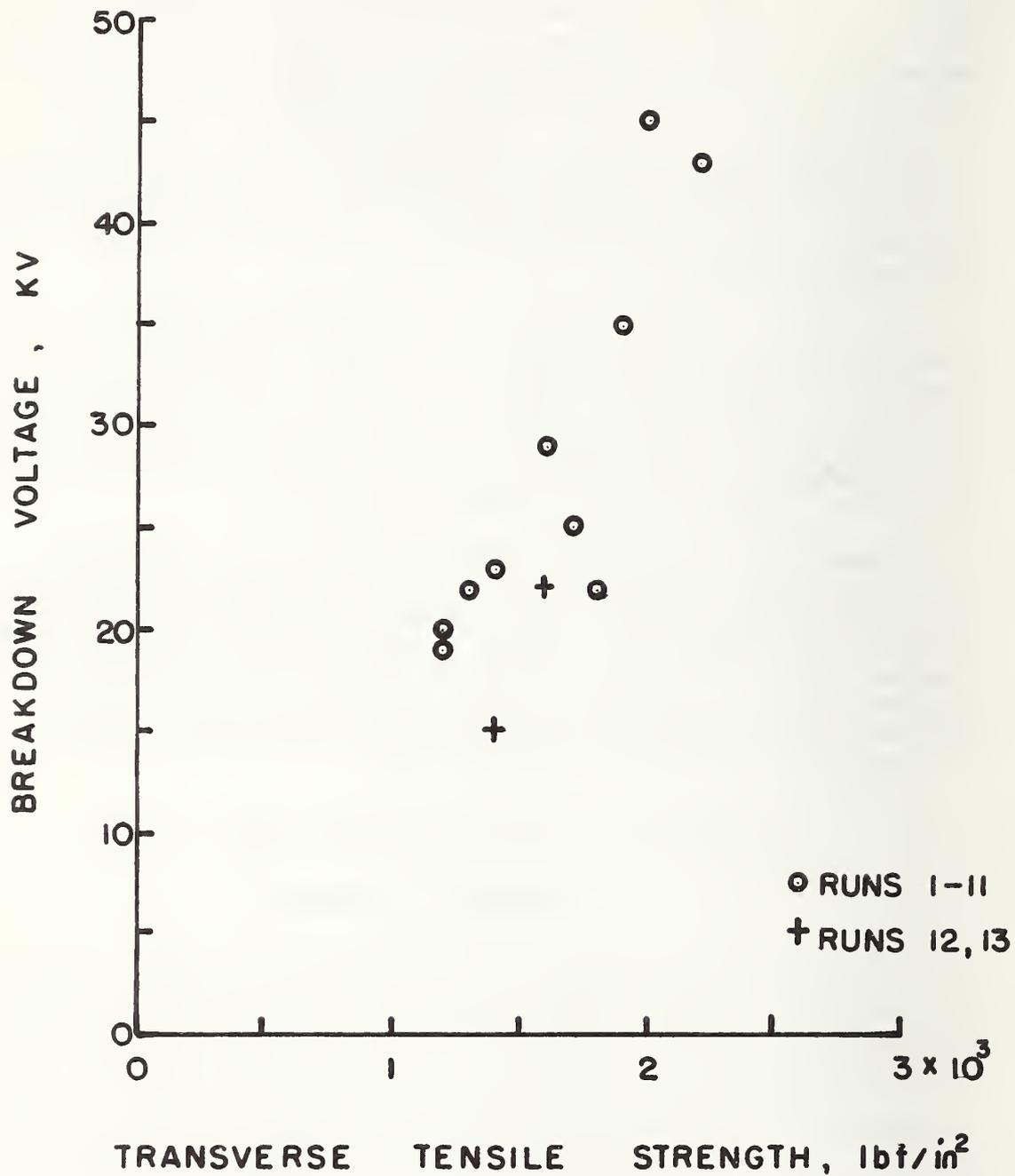
Figure 6 - Electrical breakdown voltage vs transverse tensile strength.
