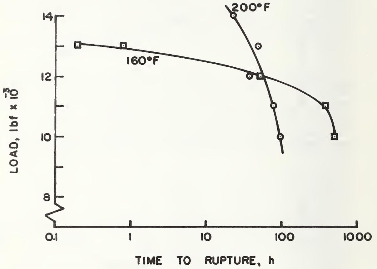
Figure 5 - Stress-rupture properties of rod from Run 2 under saturated humidity.
