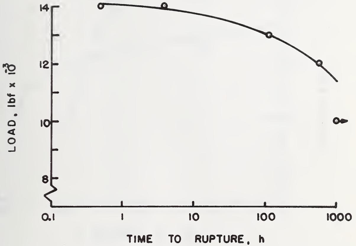
Figure 4 - Stress-rupture properties of rod from Run 1 at 200 °F under saturated humidity.
