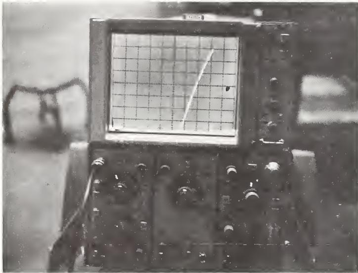
Figure 3 - Storage oscilloscope used in high-speed tensile tests, showing a typical trace of load (ordinate) vs time (abscissa).
