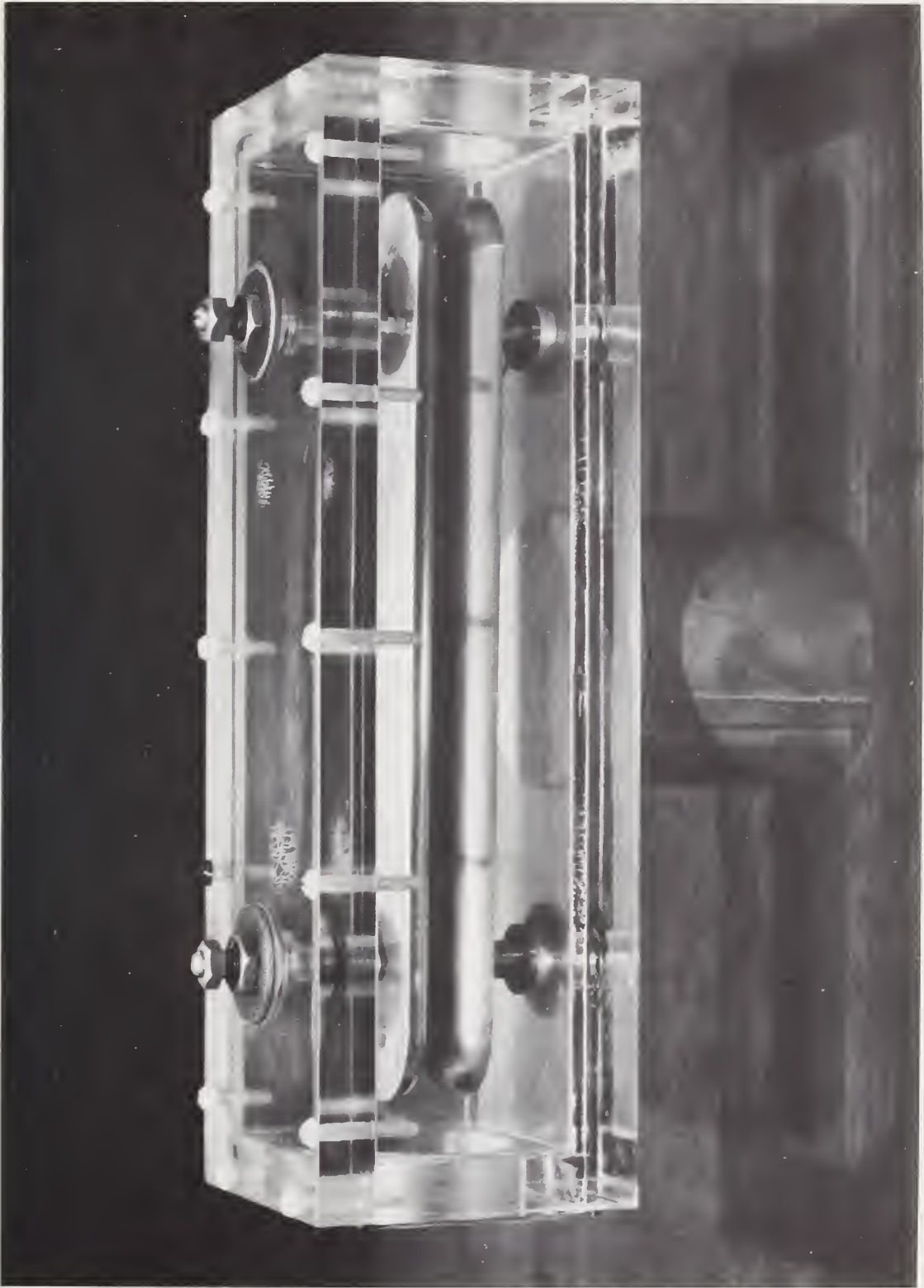
Fig. 4 Plastic cell used for measurement of the Kerr coefficient of water. The plate spacing is adjustable between about 0.25 and 1 cm.
