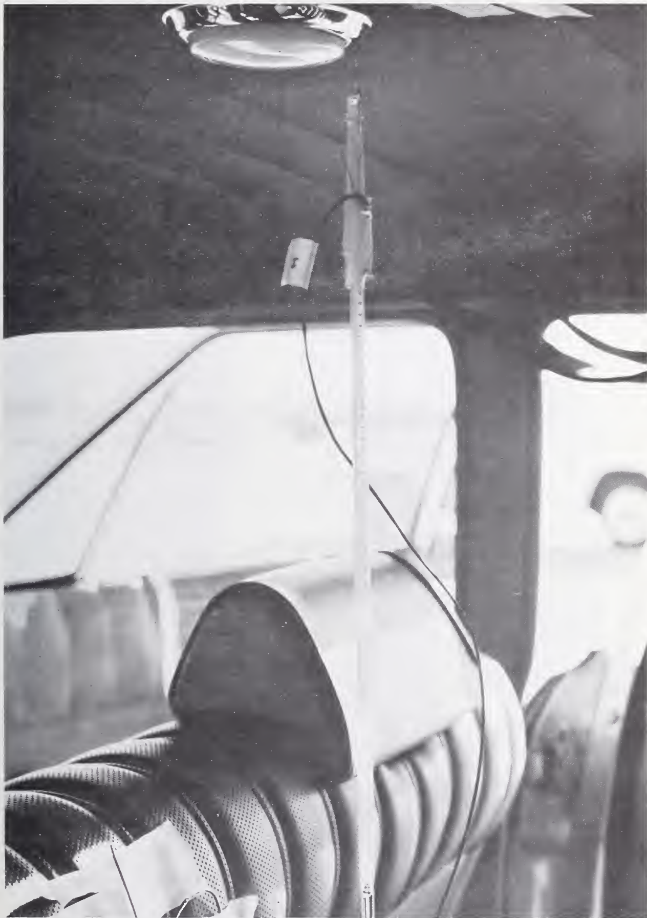
Fig. 2 Mounting of a liquid-in-glass thermometer inside of a test car.
