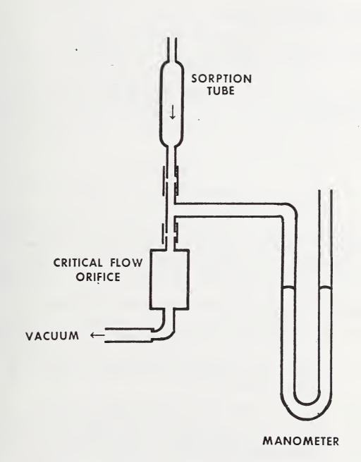
Figure 6. Pressure Drop Measurement Apparatus
