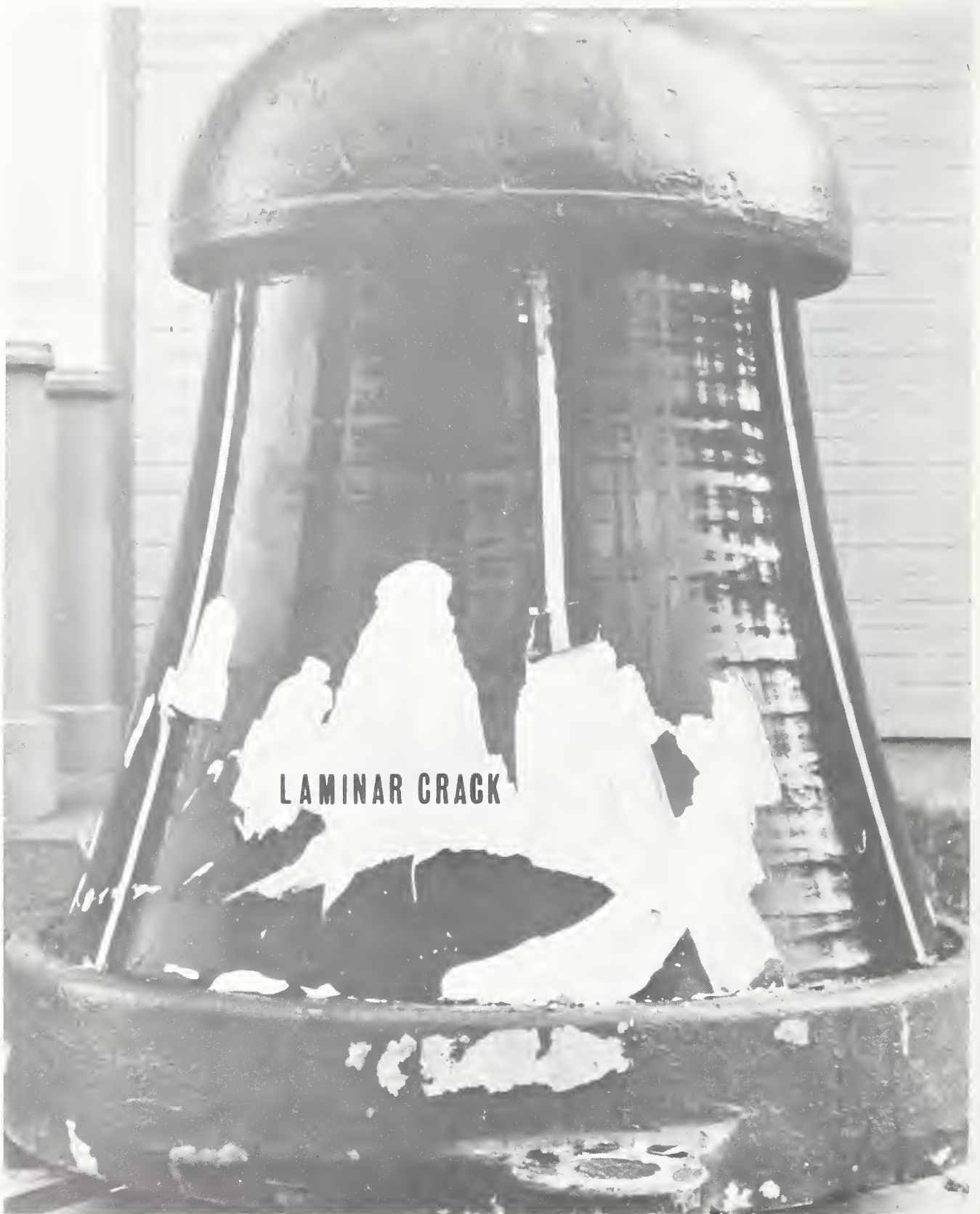
Fig. 5. An example of a laminar crack formed in a cone insulator.
