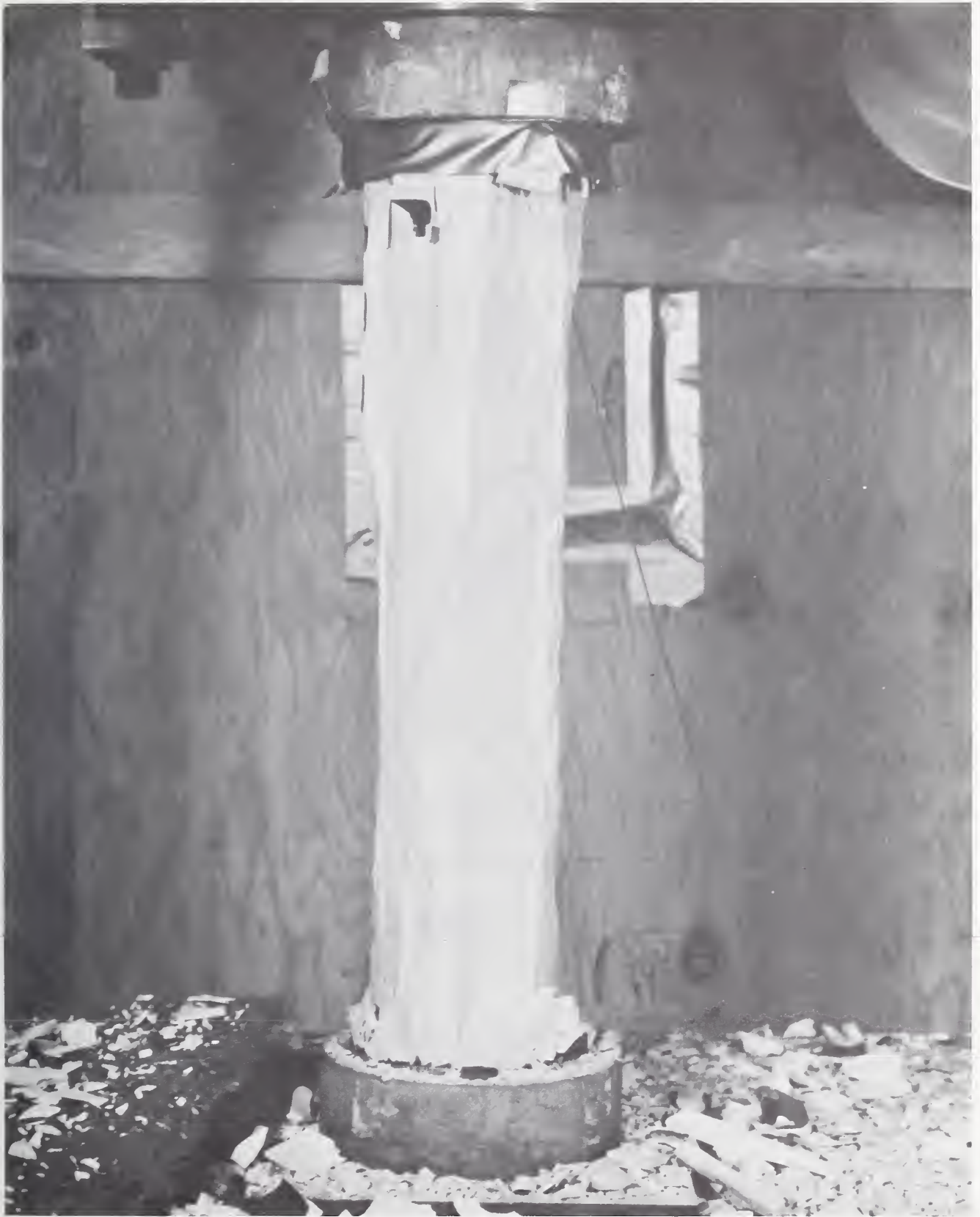
Fig. 10. A post insulator after testing to 7 MN and unloaded to 6 MN.
