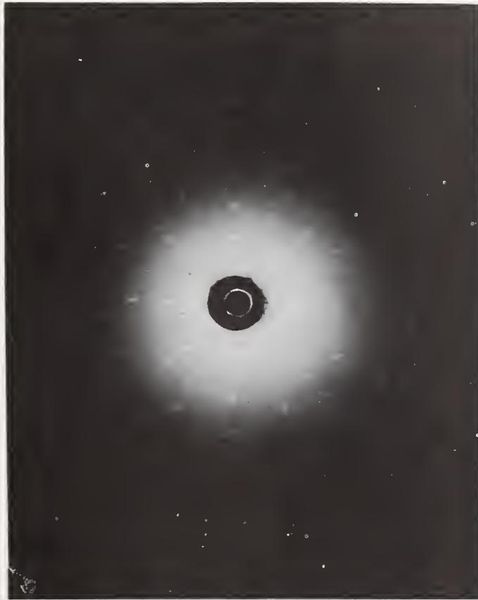
Fig. 8. Laue X-ray photograph of [001] surface.
