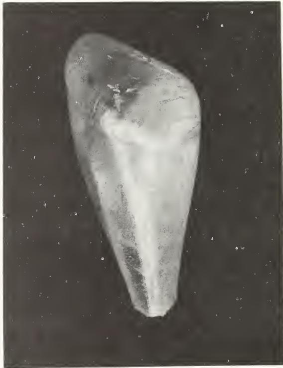
Fig. 6. Early boule of diameter approximately 17 mm grown in tube of type 5(a).
