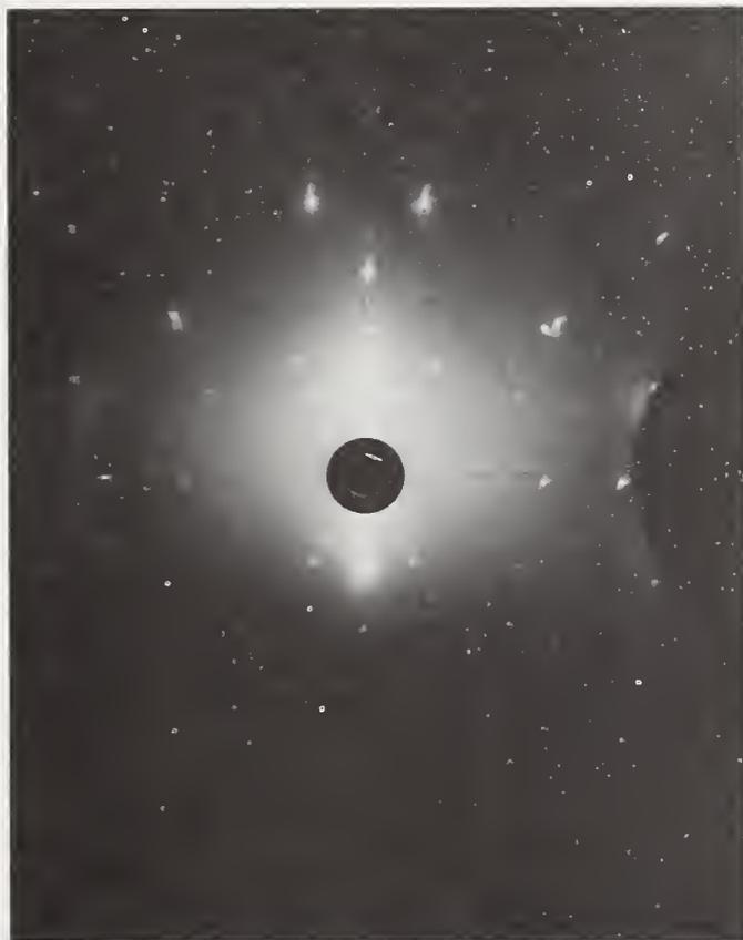
Fig. 10. Laue X-ray photograph of [110] surface. The direction of the c-axis is as shown.
