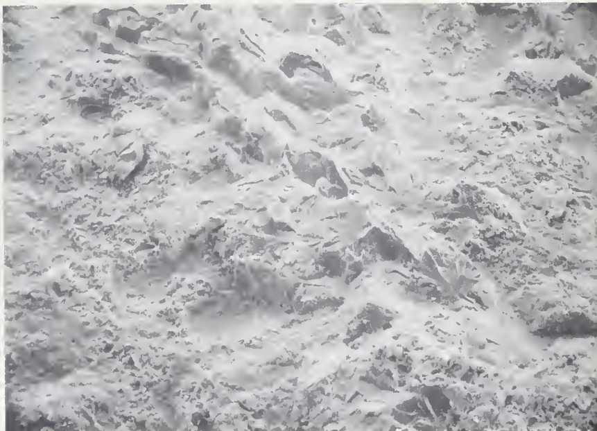
Figure 14. SEM Fractographs Taken at Location A of Figure 3, Showing Quasi-Cleavage Fracture and Oxide Formations Observed Near the Boundary of the Heat-Affected Zone of the Rim.
