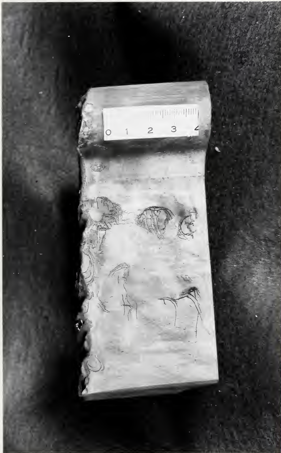
Figure 8. Thermal Checks Observed on the Tread of Section 2 After Hot Etching in 1:1 HCl. Mag. ~ X 1
