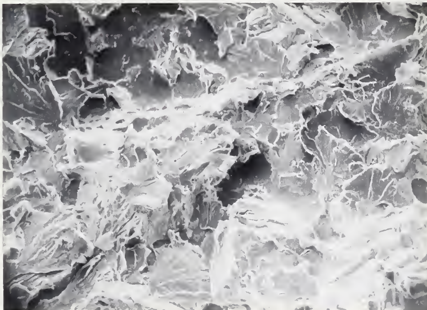
Figure 12. SEM Fractographs Taken at Location C of Figure 3, Showing the Predominately Quasi-Cleavage Fracture Mode Observed in the Rim.
