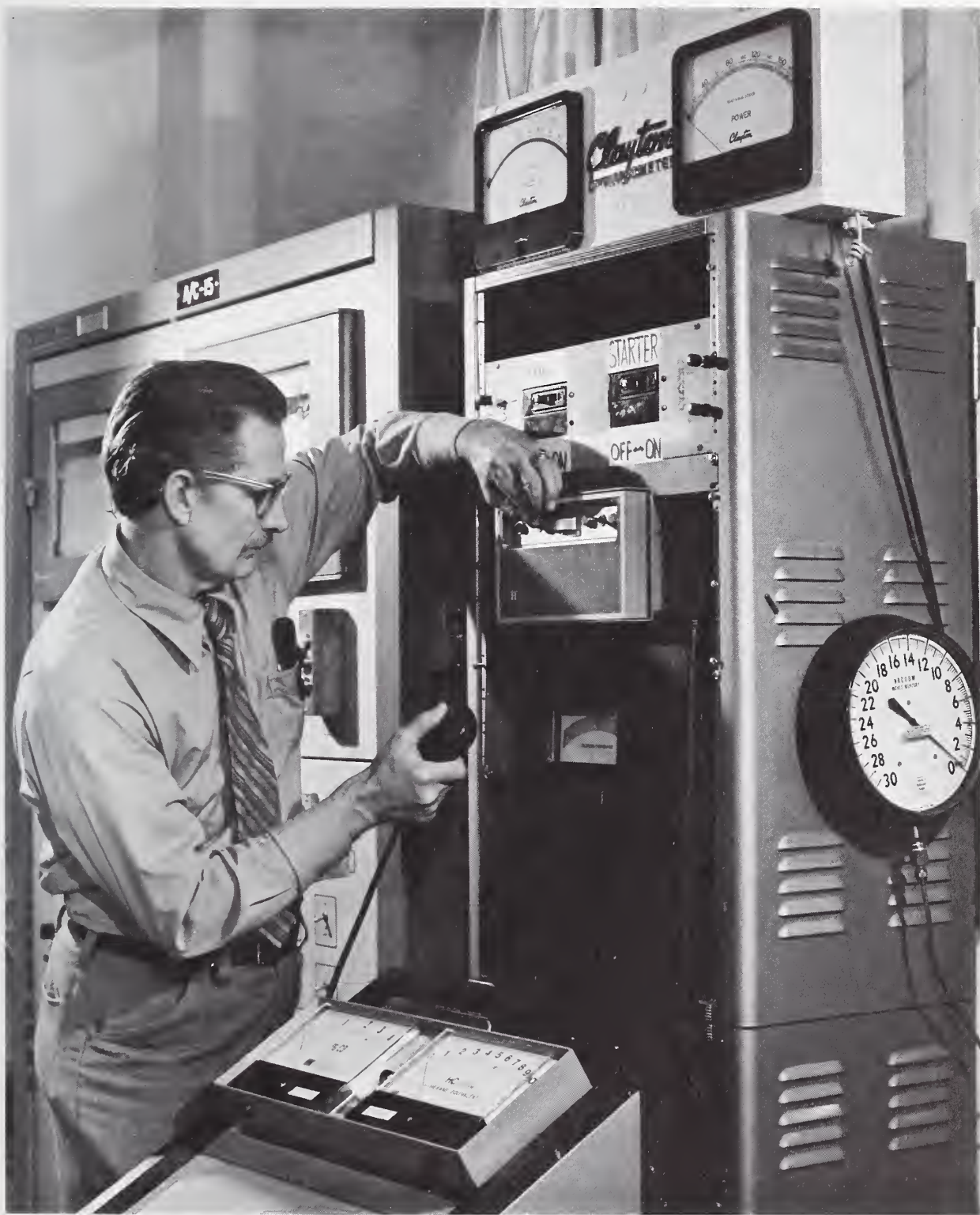
Figure 9 Engine Throttle Position and Dynamometer Adjustments Being Made from the Instrumentation Room
