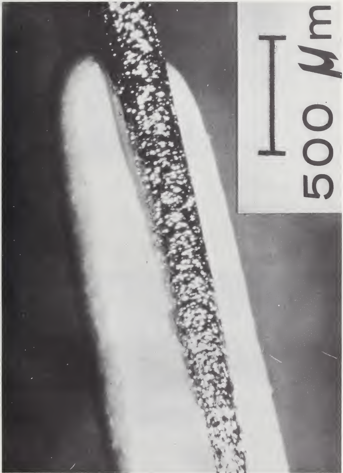
Figure 13. Photomicrograph showing the erosion of the BeO insulator near the measuring junction of an unsheathed thermocouple that was exposed within a tantalum blackbody enclosure for 307 hours at 2400 K in argon.
