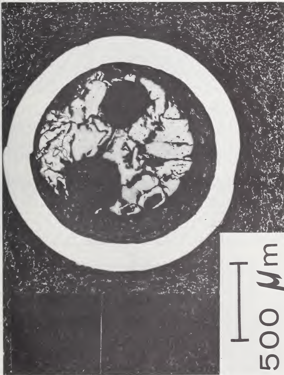
Figure 18. Photomicrograph showing a transverse cross-section of a BeO-Ta sheath assembly after exposure for 50 hours at 2400 K in argon. The cross-section was taken at about 4 cm below the open end of the sheath.
