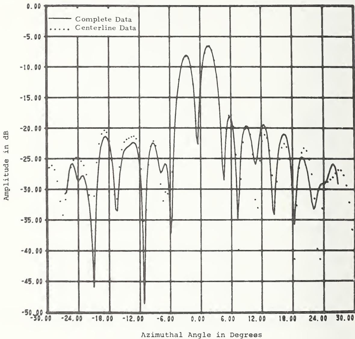
Figure 33. Comparison Between Far-Field Patterns Computed from Complete and Centerline Data. Volphase Antenna, 0° Azimuth Difference Pattern.
