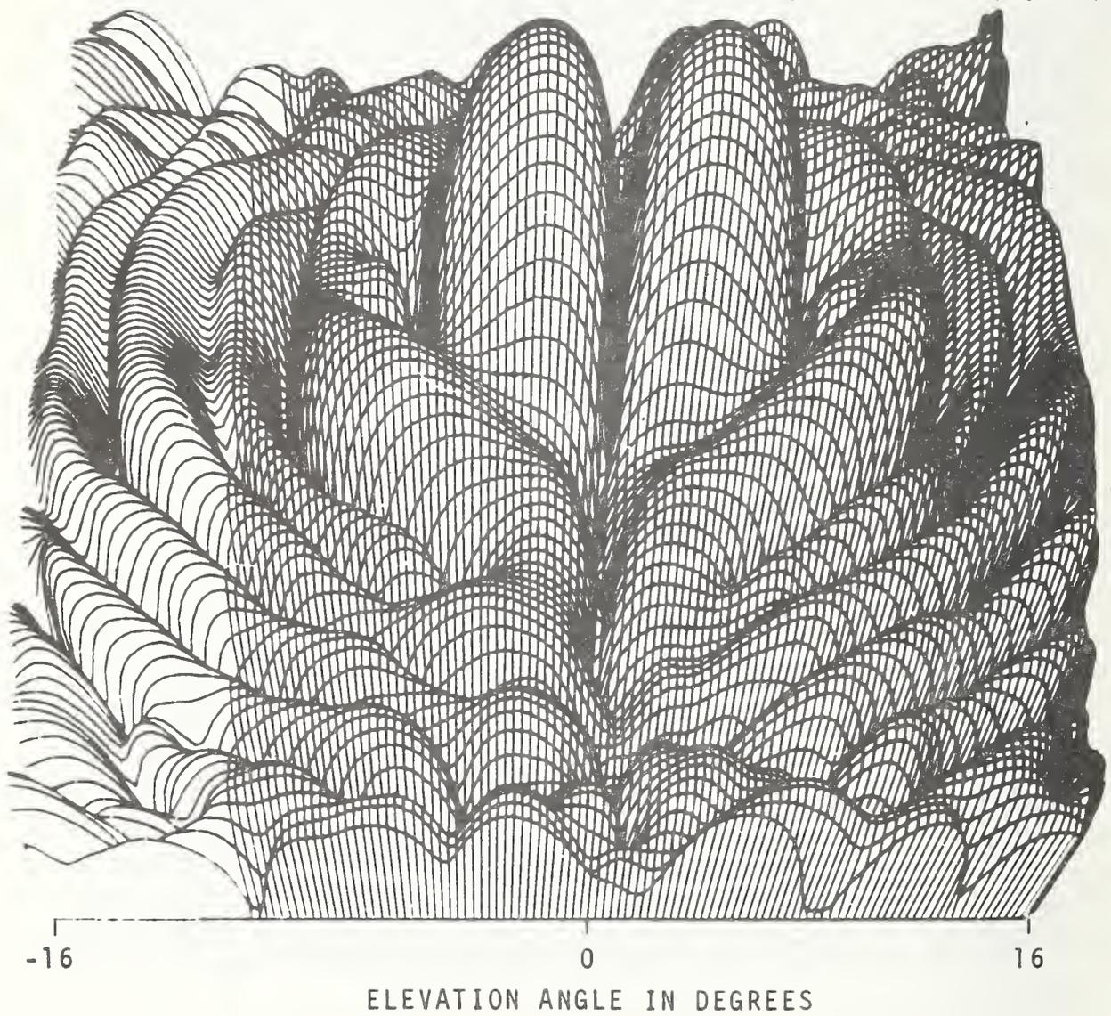
Figure 40. Constrained Lens Elevation Difference Port Log Amplitude,  $f = 9.2$  GHz, Computed from  $z = 25$  cm Data, No Radome.
