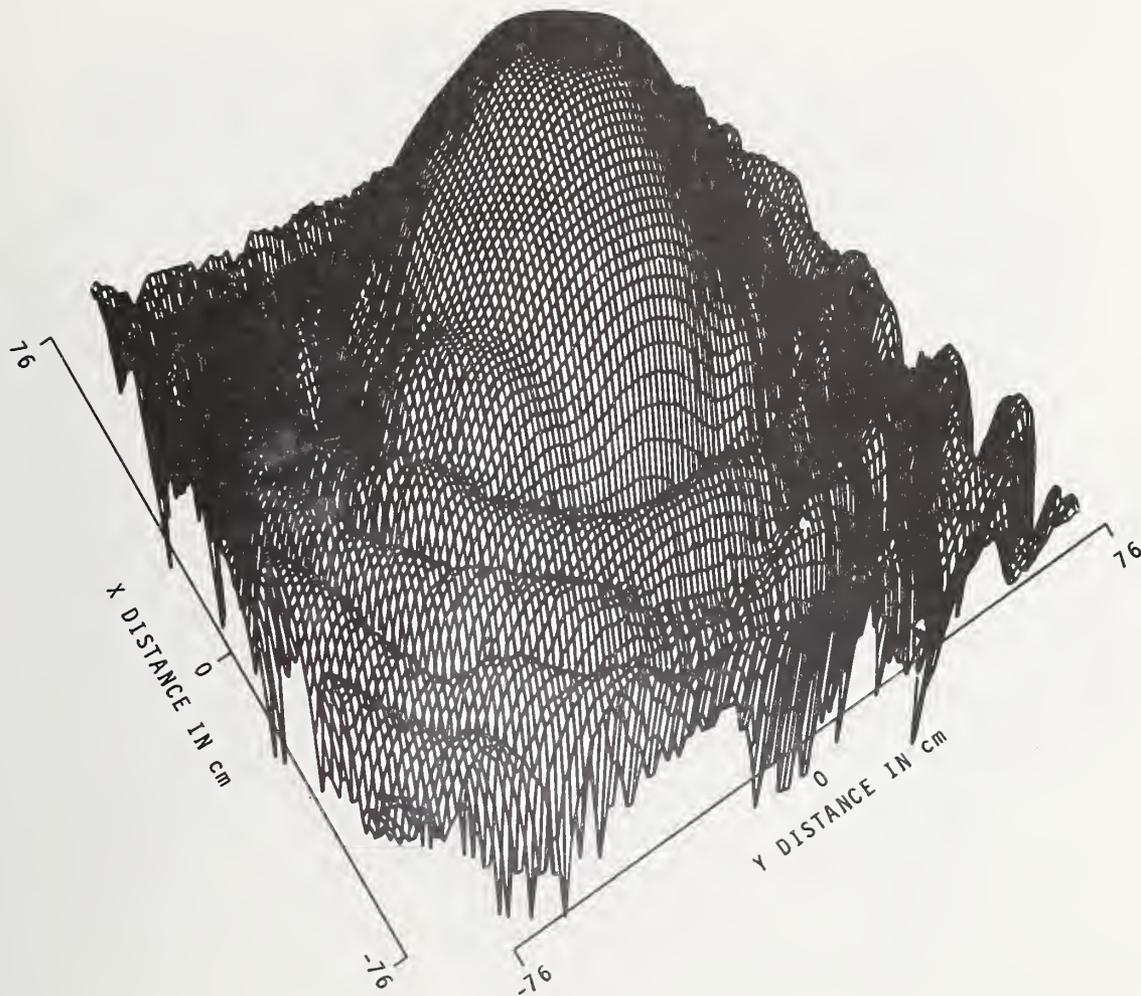
Figure 36a. Constrained Lens Sum Port Near-Field Log Amplitude,  $f = 9.2$  GHz,  $z = 254$  cm, No Radome.
