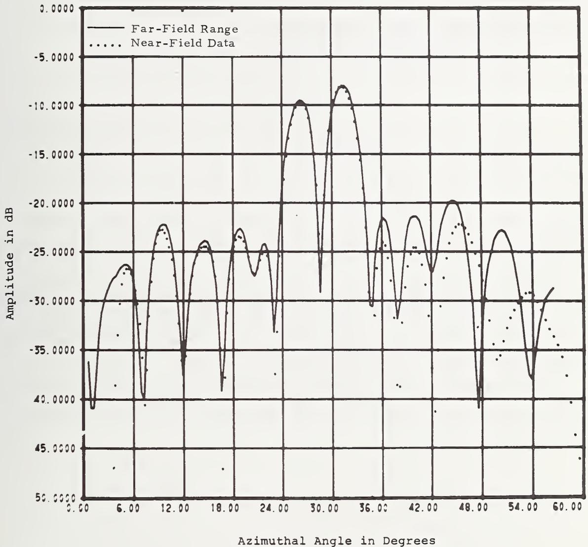
Figure 48. Comparison Between Far-Field Pattern Measured on Far-Field Range and Computed from Near-Field Data. Volphase Antenna, 30° Azimuth Difference Pattern.
