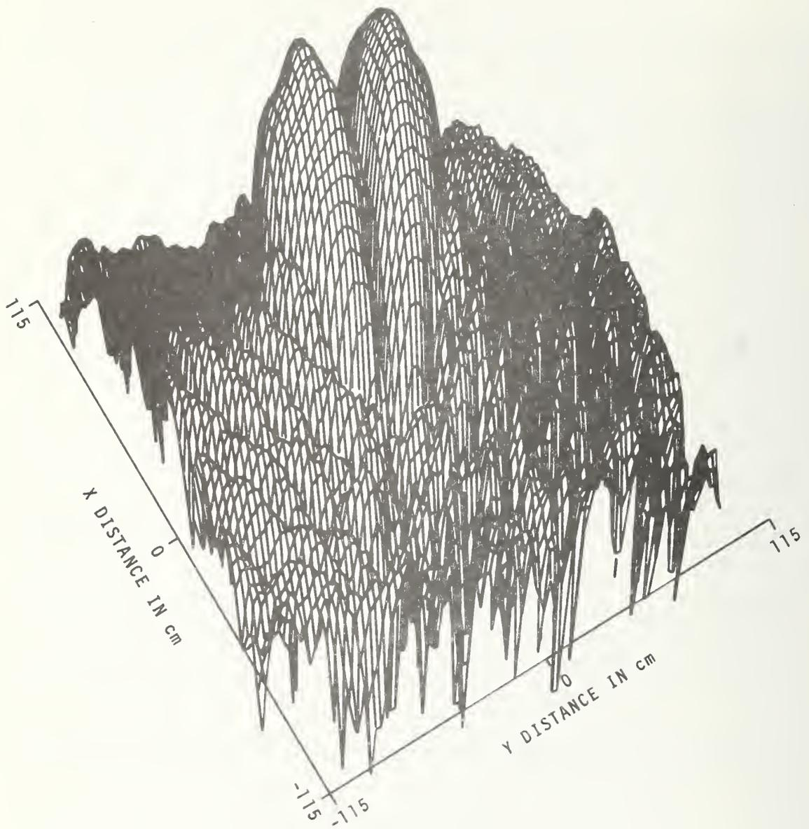
Figure 39a. Constrained Lens Elevation Difference Port Near-Field Log Amplitude,  $f = 9.2$  GHz,  $z = 250$  cm, No Radome.
