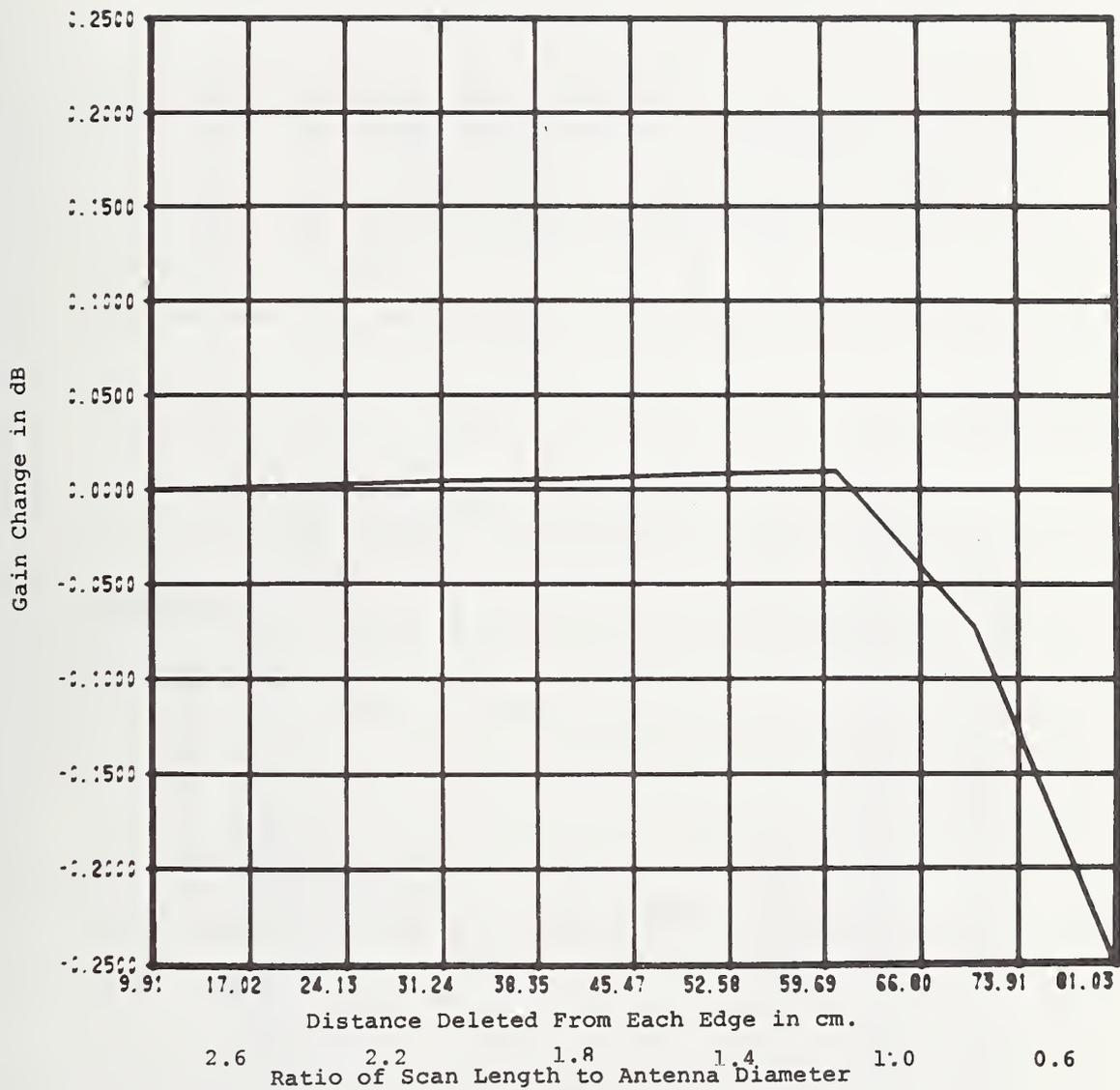
Figure 14. Change in Computed Gain Due to Decreasing Scan Length.
