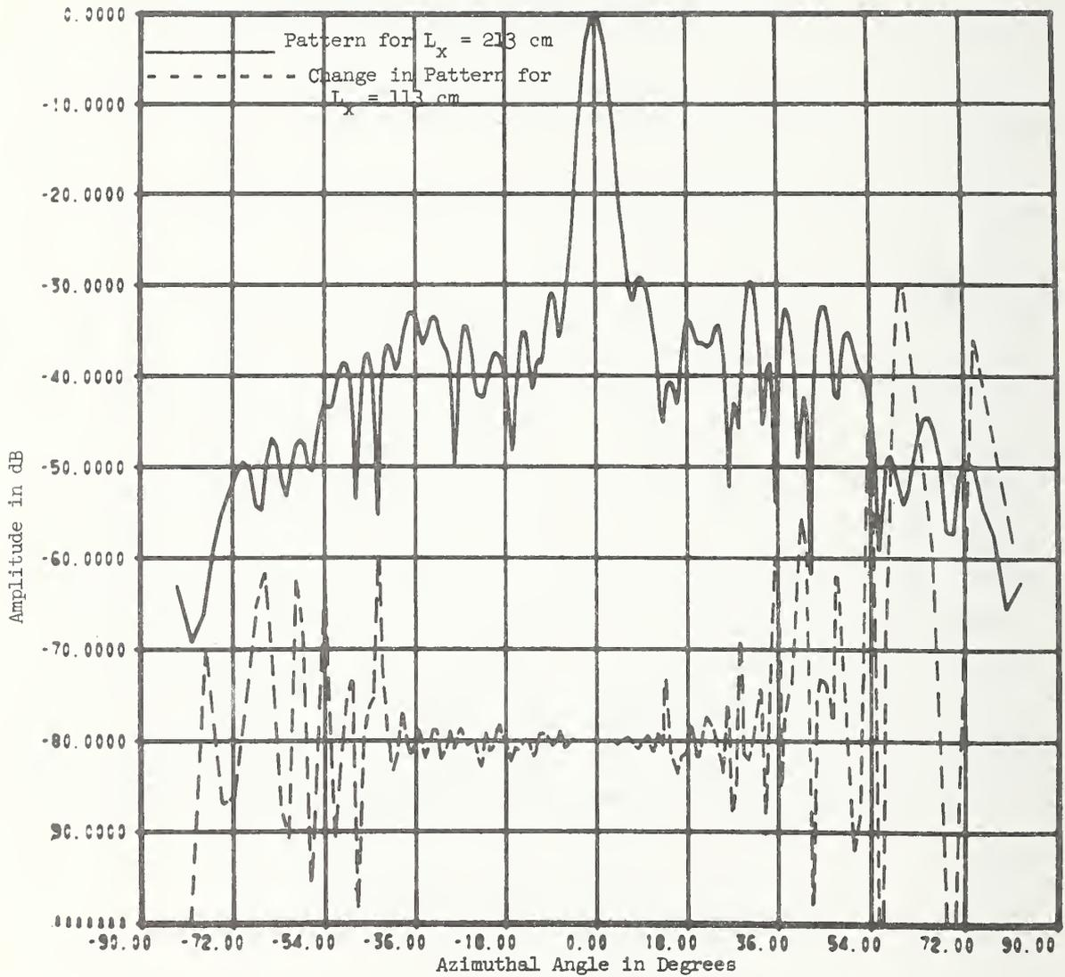
Figure 15. Change in Far-Field Pattern Due to Decreasing Scan Length,  $L_x = 213$  cm and  $L_x = 113$  cm.
