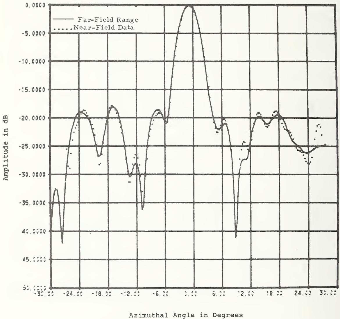
Figure 45. Comparison Between Far-Field Patterns Measured on Far-Field Range and Computed from Near-Field Data. Volphase Antenna, 0° Sum Pattern.
