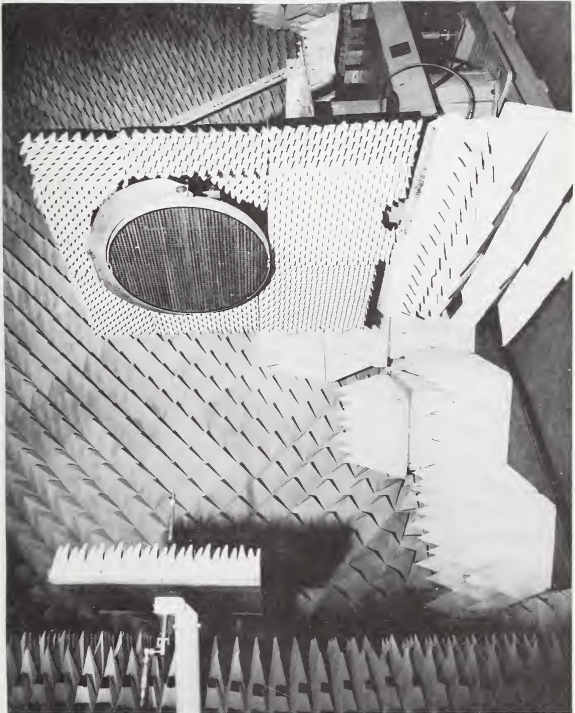
Figure 5. Constrained Lens Antenna and Probe.
