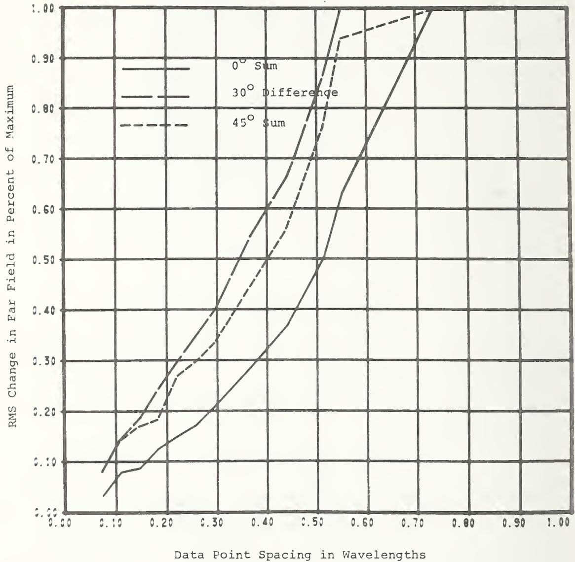
Figure 23. Change in Computed Far-Field Due to Increased Data Point Spacing. Volphase Antenna,  $z = 38$  cm.  $Az = 0^\circ, 30^\circ, 45^\circ, EL = 0^\circ$ .
