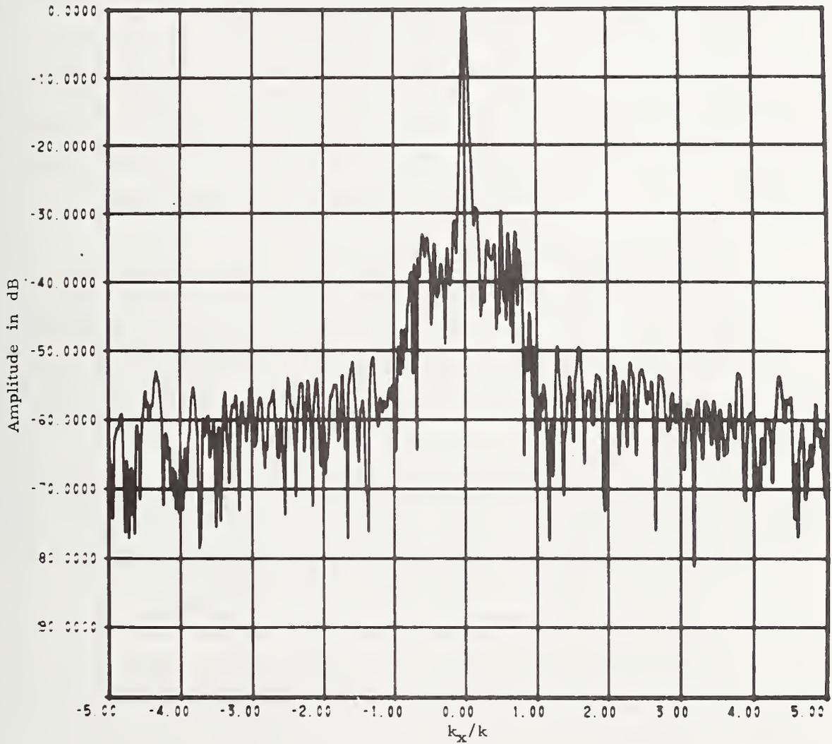
Figure 19. Amplitude Spectrum for Both Propagating and Evanescent Modes on Constrained Lens Antenna.
