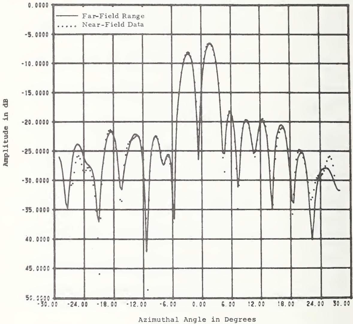
Figure 47. Comparison Between Far-Field Patterns Measured on Far-Field Range and Computed from Near-Field Data. Volphase Antenna, 0° Azimuth Difference Pattern.
