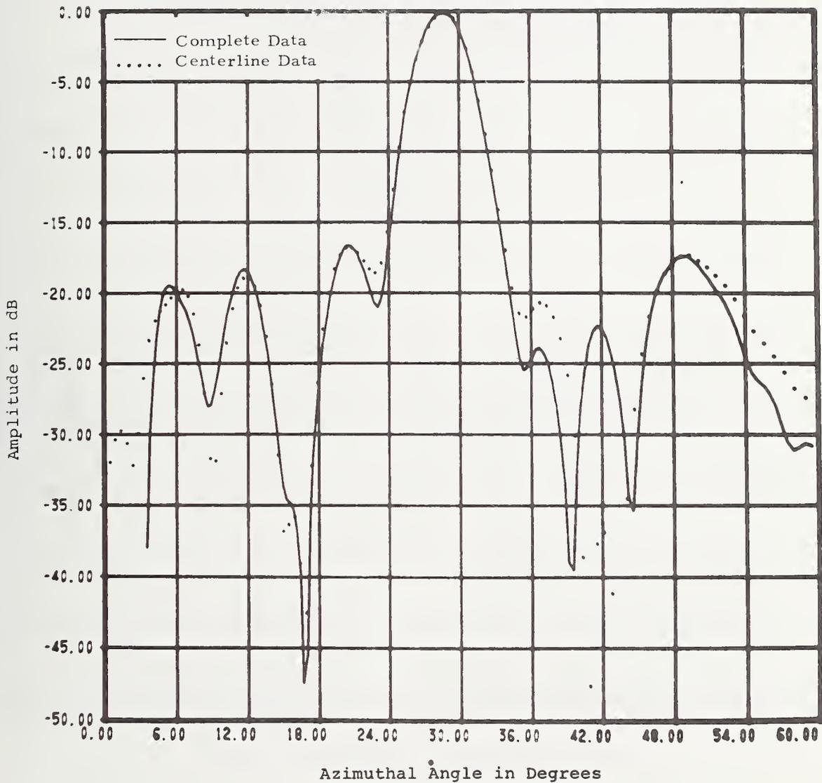
Figure 32. Comparison Between Far-Field Patterns Computed from Complete and Centerline Data. Volphase Antenna, 30° Sum Pattern.
