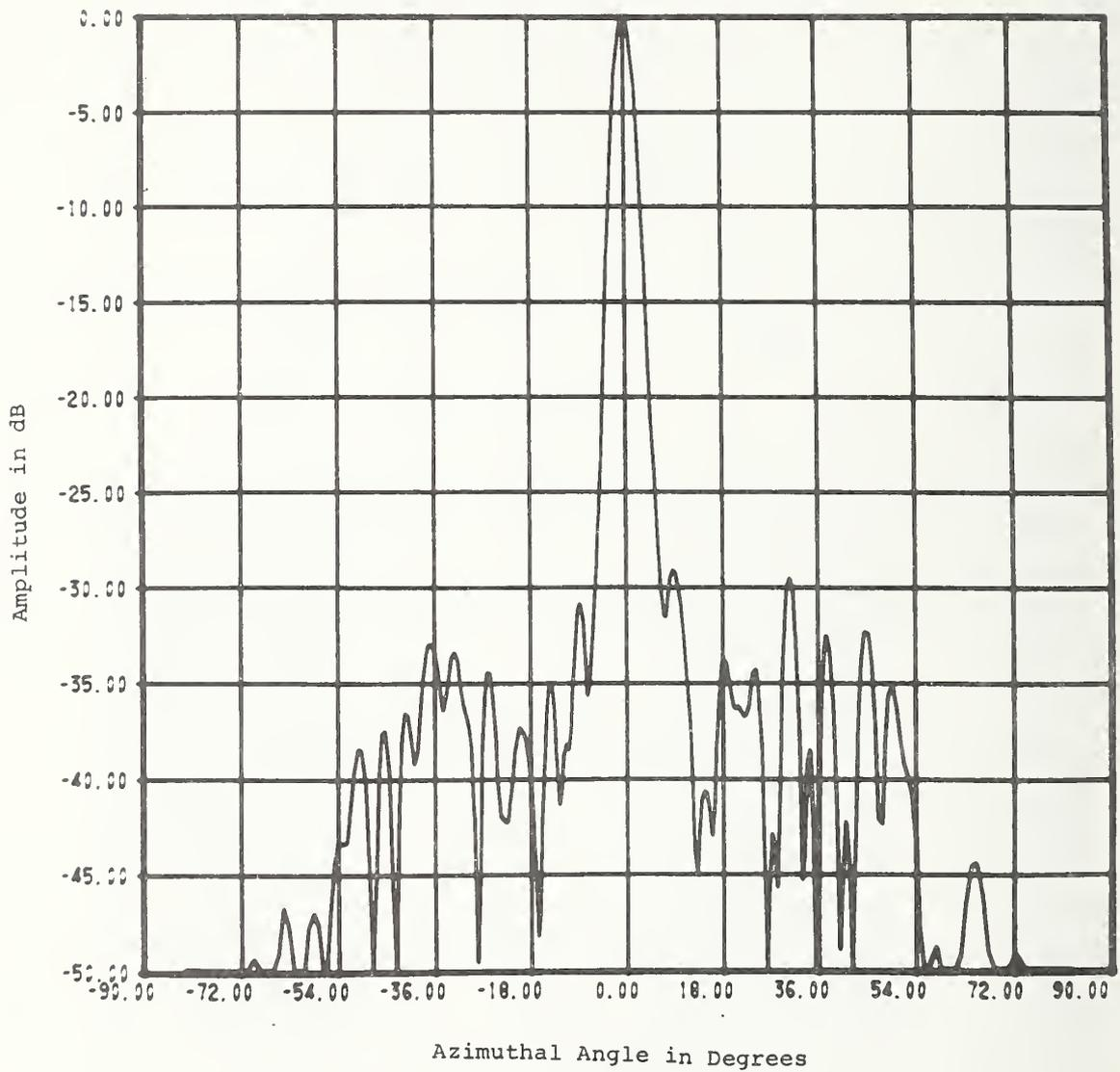
Figure 12. Approximate Far-Field Pattern Computed from Centerline Data Taken on Constrained Lens Antenna.  $z = 25$  cm,  $Az = EL = 0^\circ$ .
