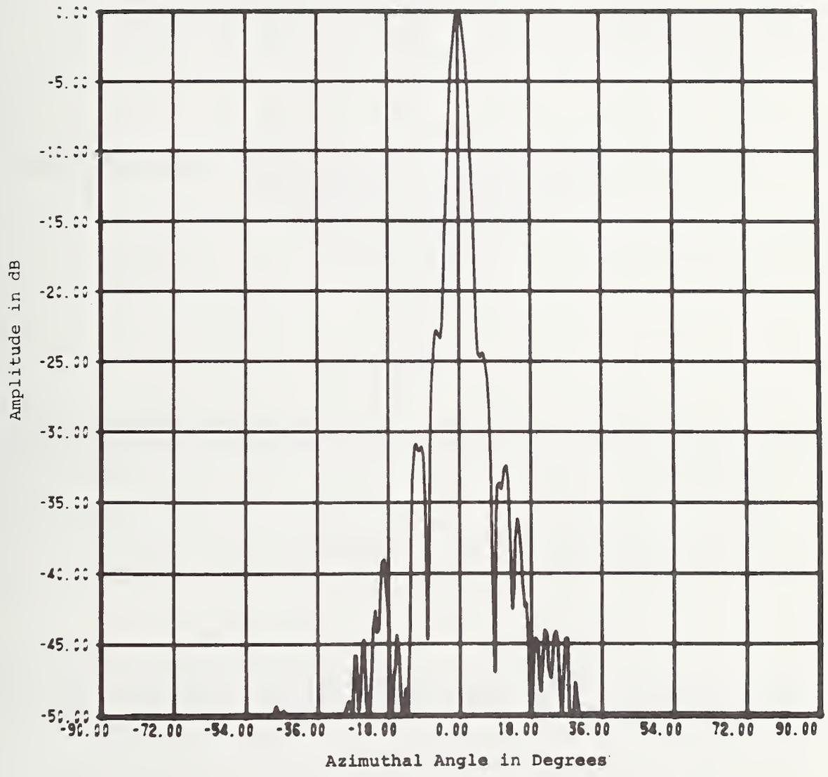
Figure 17. Approximate Far-Field Pattern Computed from Center-line Data Taken on Constrained Lens Antenna,  $z = 254$  cm,  $Az = EL = 0^\circ$ .
