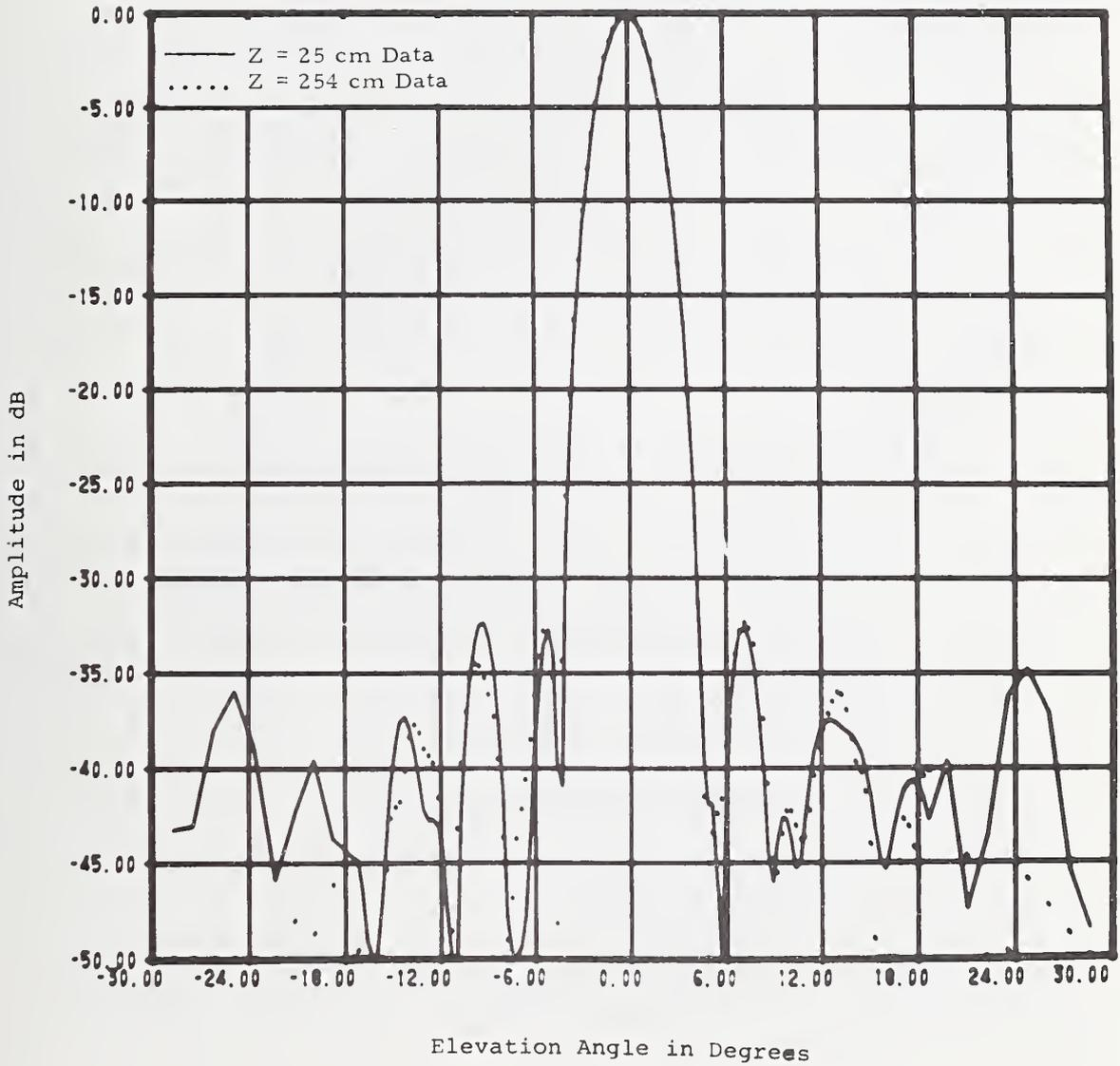
Figure 38. Comparison Between Far-Field Patterns Computed from Near-Field Data taken at Two Different z-Distances. Constrained Lens Antenna, E-Plane Sum Pattern.
