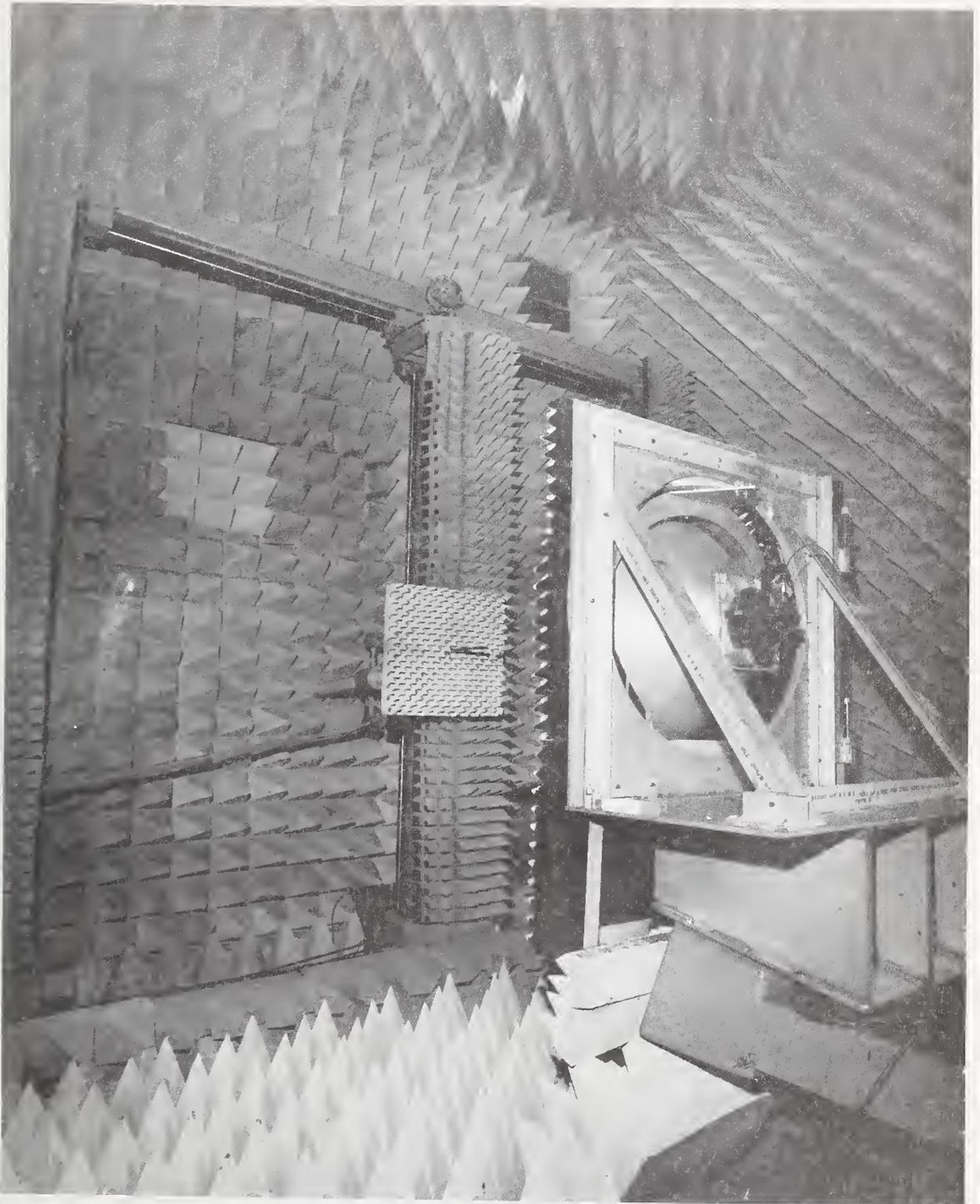
Figure 7. Scanner for Moving Probe in x-y Plane.
