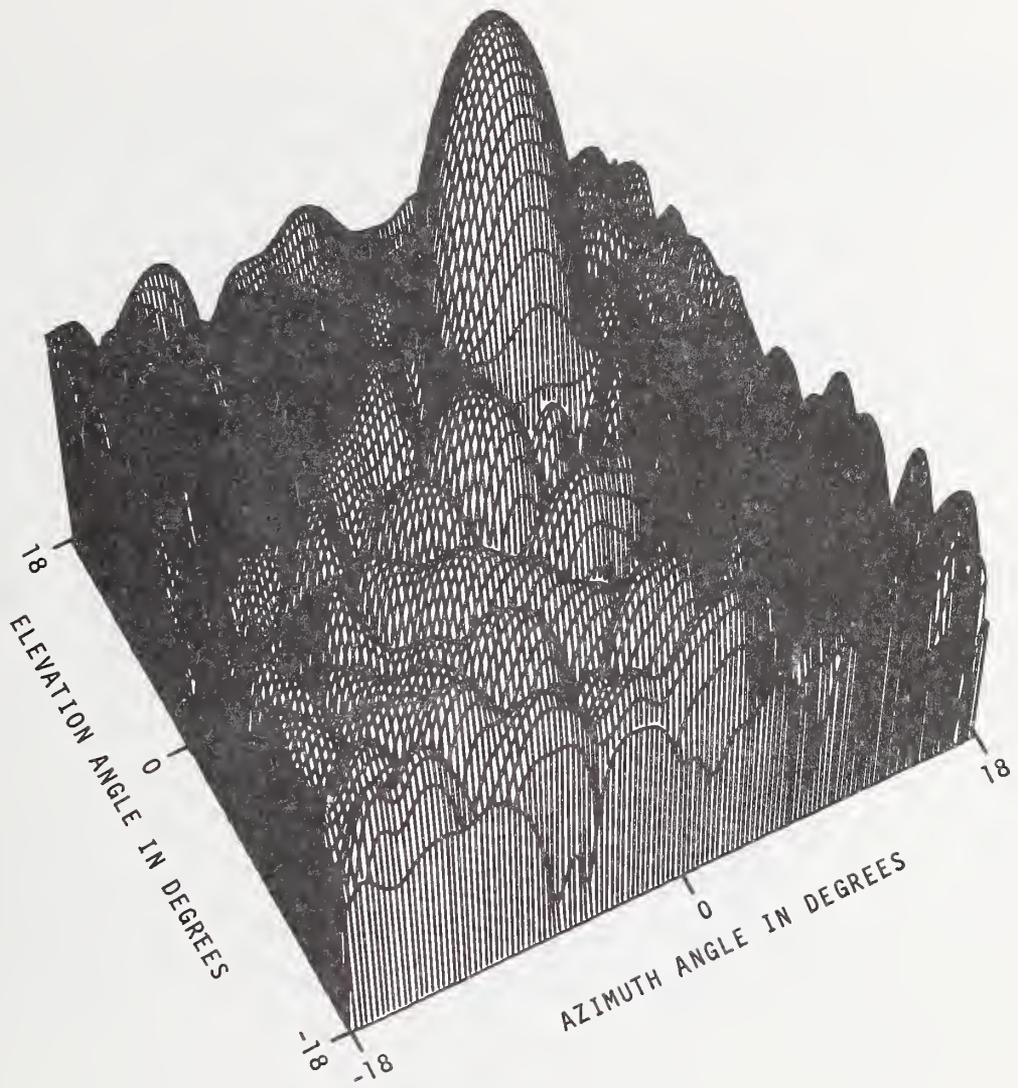
Figure 37. Constrained Lens Sum Port Far-Field Log Amplitude,  $f = 9.2$  GHz, Computed from  $z = 25$  cm Data, No Radome.
