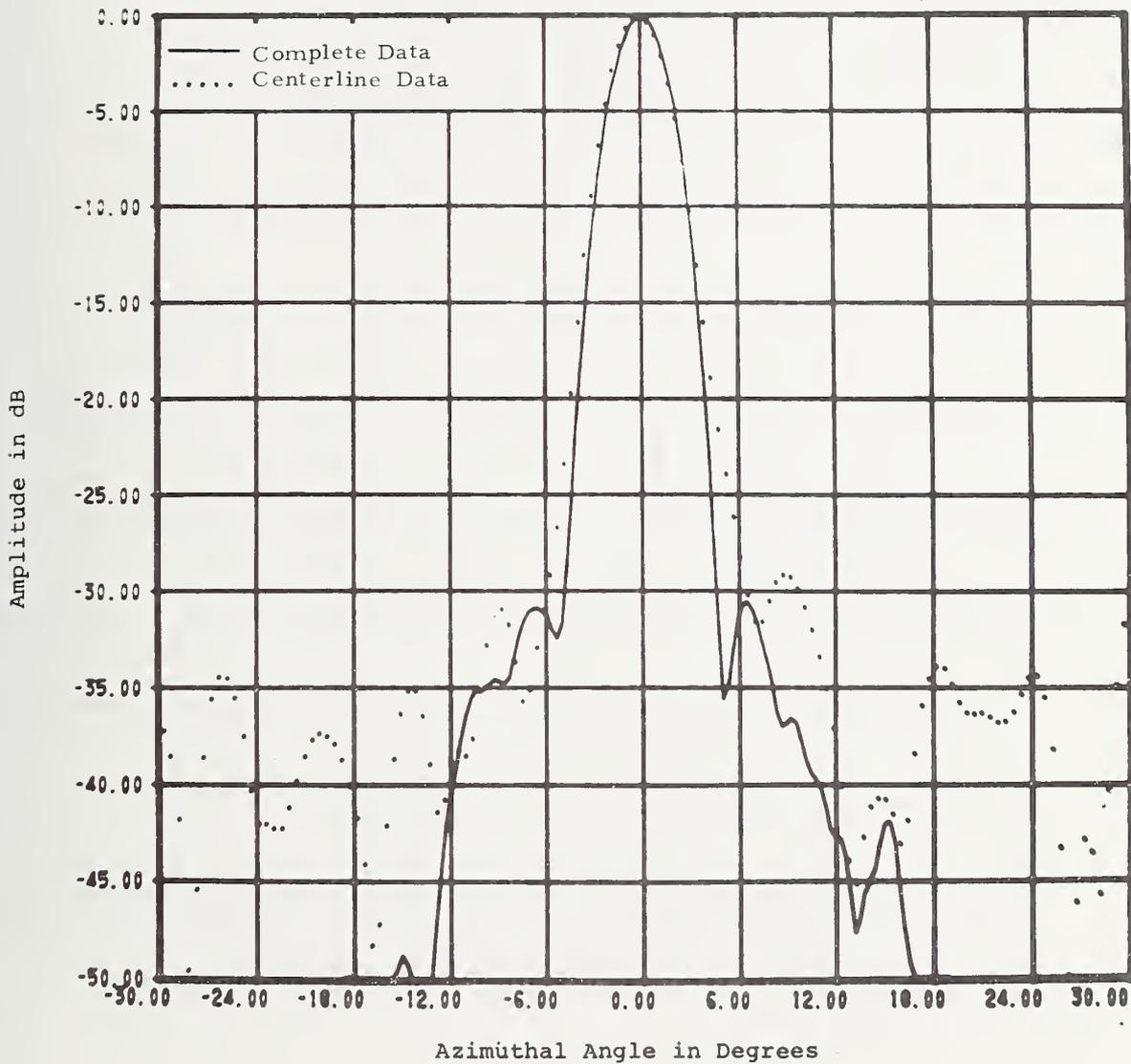
Figure 30. Comparison Between Far-Field Patterns Computed from Complete and Centerline Data. Constrained Lens Antenna, H-Plane Sum Pattern.
