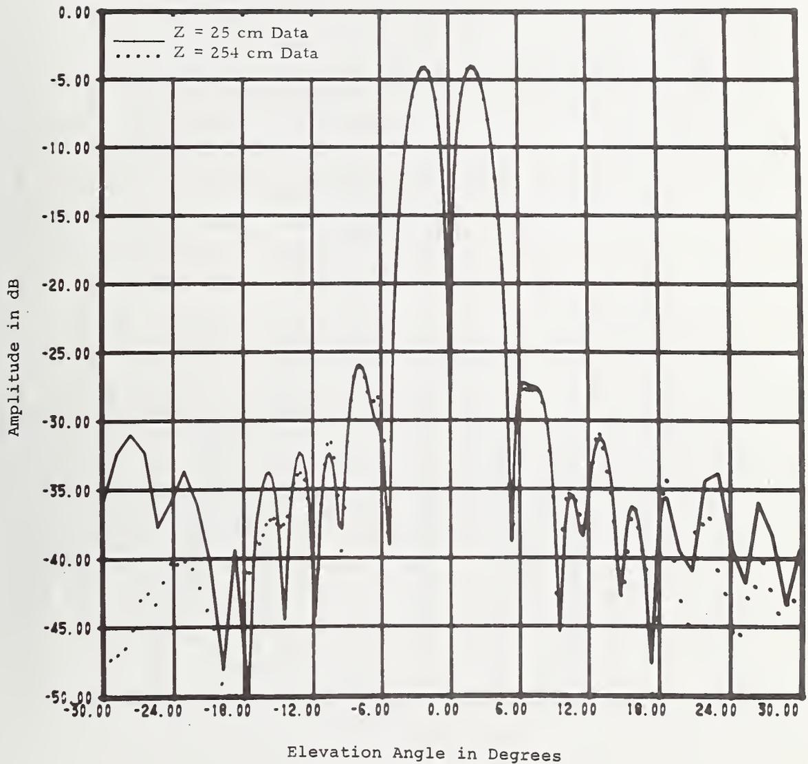
Figure 41. Comparison Between Far-Field Patterns Computed from Near-Field Data taken at Two Different z-Distances. Constrained Lens, E-Plane Elevation Difference Pattern.
