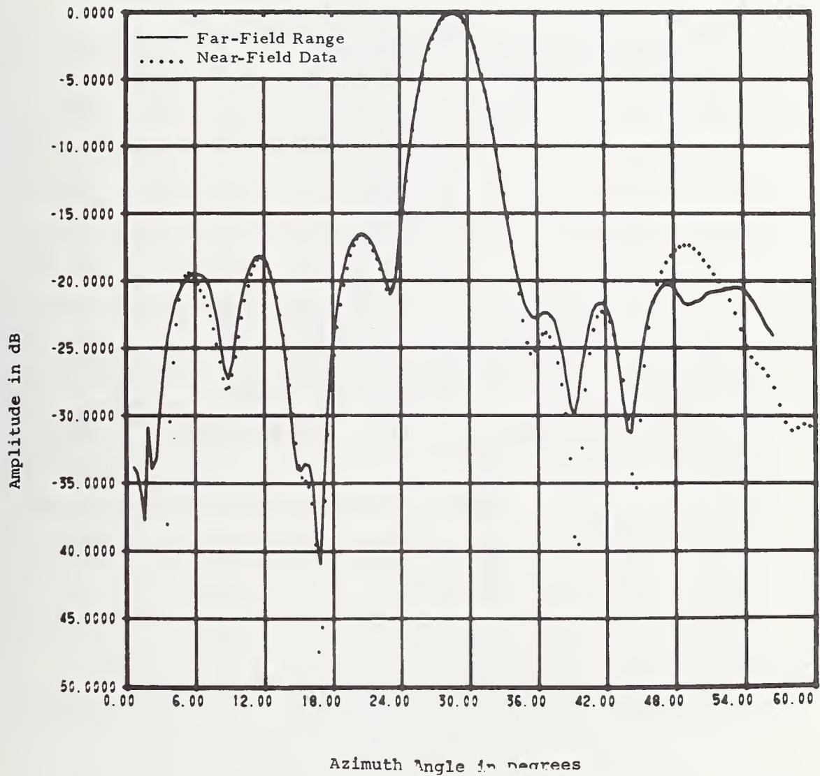
Figure 46. Comparison Between Far-Field Patterns Measured on Far-Field Range and Computed from Near-Field Data. Volphase, 30° Sum Pattern.
