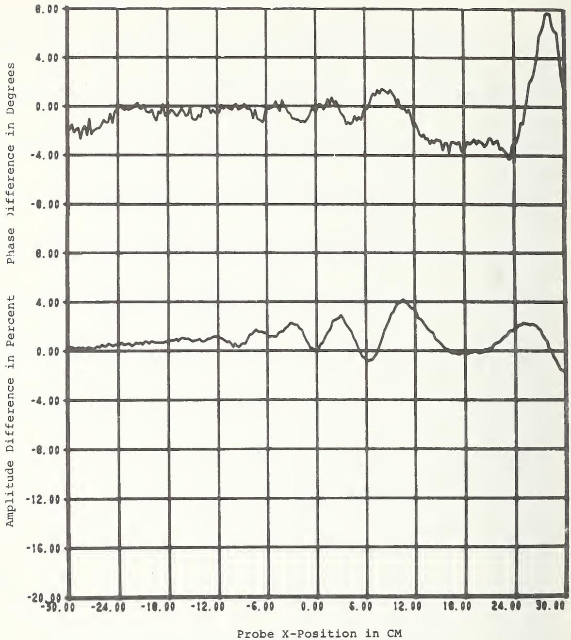
Figure 28. Change in Amplitude and Phase Due to 180° Simulated Fault at x = 18 cm.
