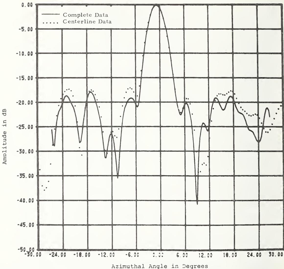
Figure 31. Comparison Between Far-Field Patterns Computed from Complete and Centerline Data. Volphase Antenna, 0° Sum Pattern.
