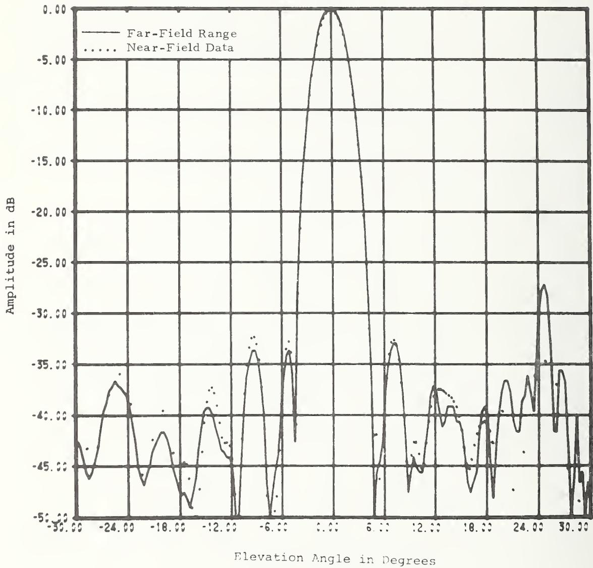
Figure 43. Comparison Between Far-Field Patterns Measured on Far-Field Range and Computed from Near-Field Data. Constrained Lens, E-Plane Sum Pattern.
