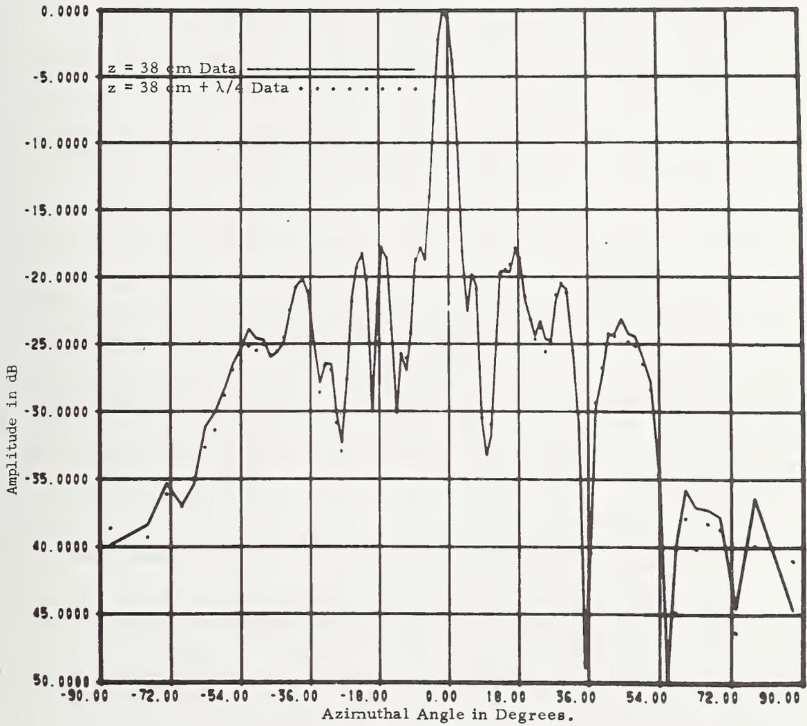
Figure 25. Far-Fields Computed from Data at z-Distance which Differ by  $\lambda/4$ , Volphase Antenna.
