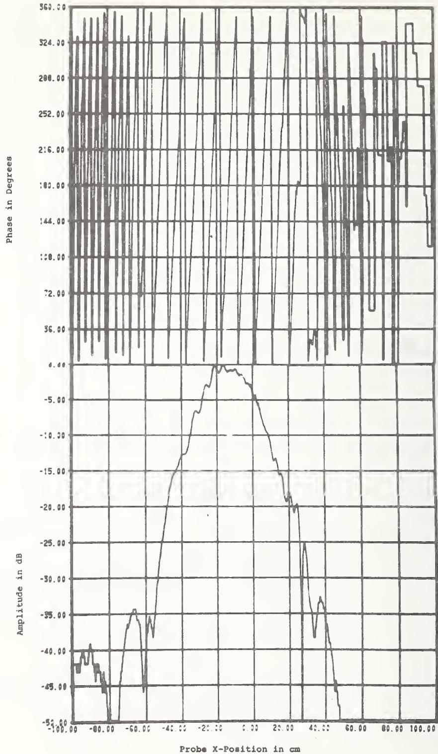
Figure 22. Near-Field Centerline Data, Constrained Lens Antenna,  $z = 25$  cm,  $Az = 20^\circ$ ,  $EL = 0^\circ$ .
