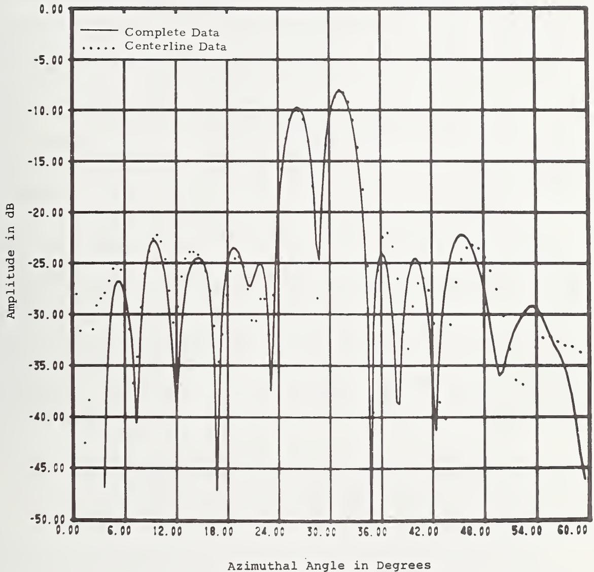
Figure 34. Comparison Between Far-Field Patterns Computed from Complete and Centerline Data. Volphase Antenna, 30° Azimuth Difference Pattern.
