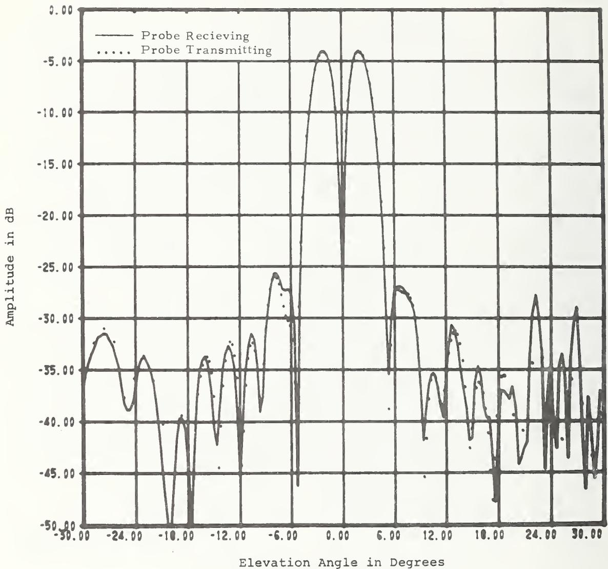
Figure 42. Comparison Between Far-Field Patterns Computed from Near-Field Data with Probe Transmitting and Receiving. Constrained Lens Antenna, E-Plane Elevation Difference Pattern.
