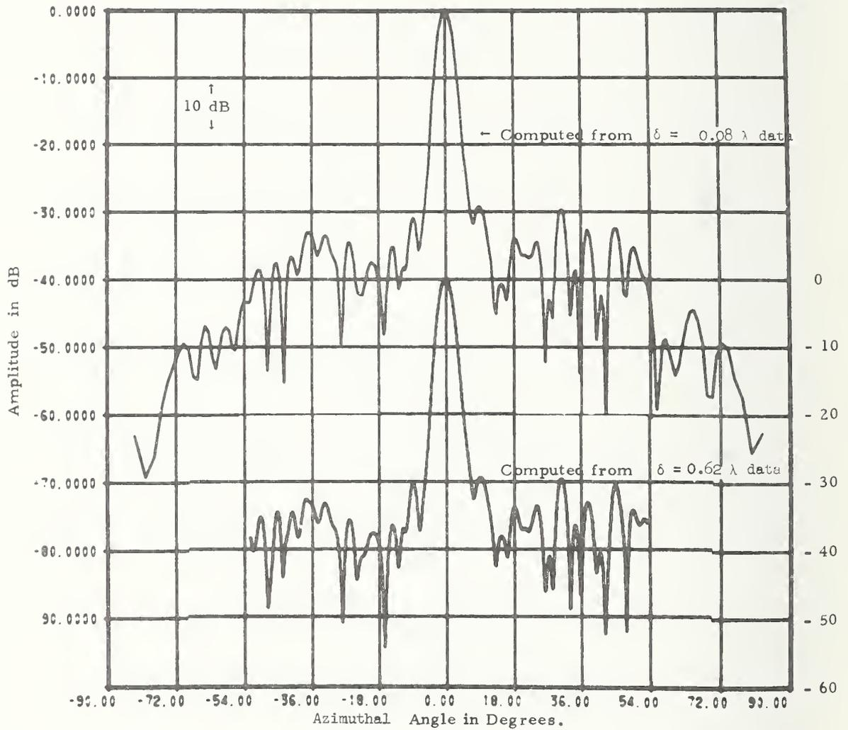
Figure 21. Comparison of Patterns Computed from Near-Field Data with  $\delta_x = .08\lambda$  and  $\delta_x = 0.62\lambda$ , Constrained Lens Antenna.
