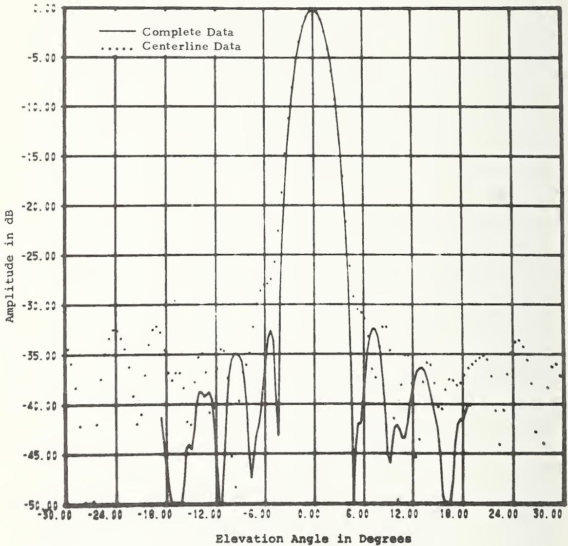
Figure 29. Comparison Between Far-Field Patterns Computed from Complete and Centerline Data. Constrained Lens Antenna, E-Plane Sum Pattern.
