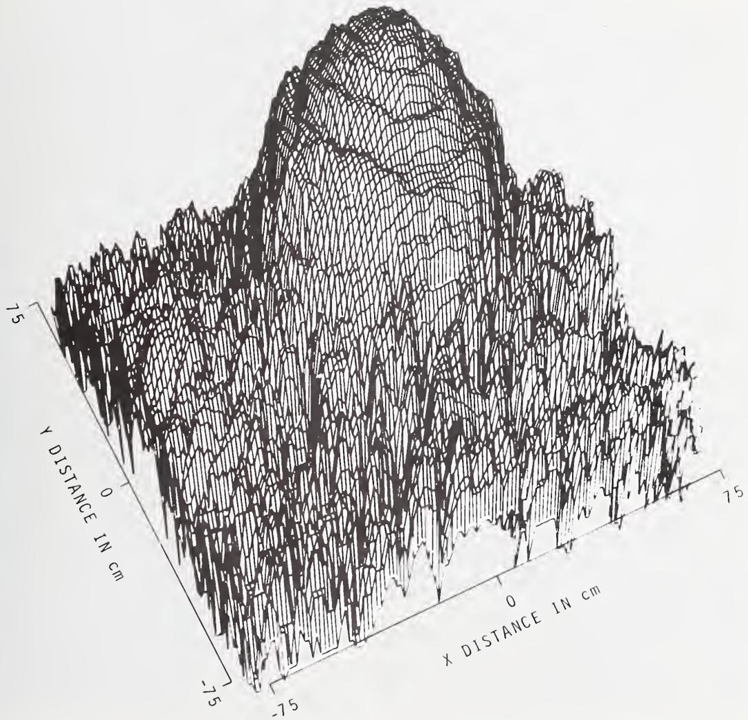
Figure 35a. Constrained Lens Sum Port Near-Field Log Amplitude,  $f = 9.2$  GHz,  $z = 25.0$  cm, No Radome.
