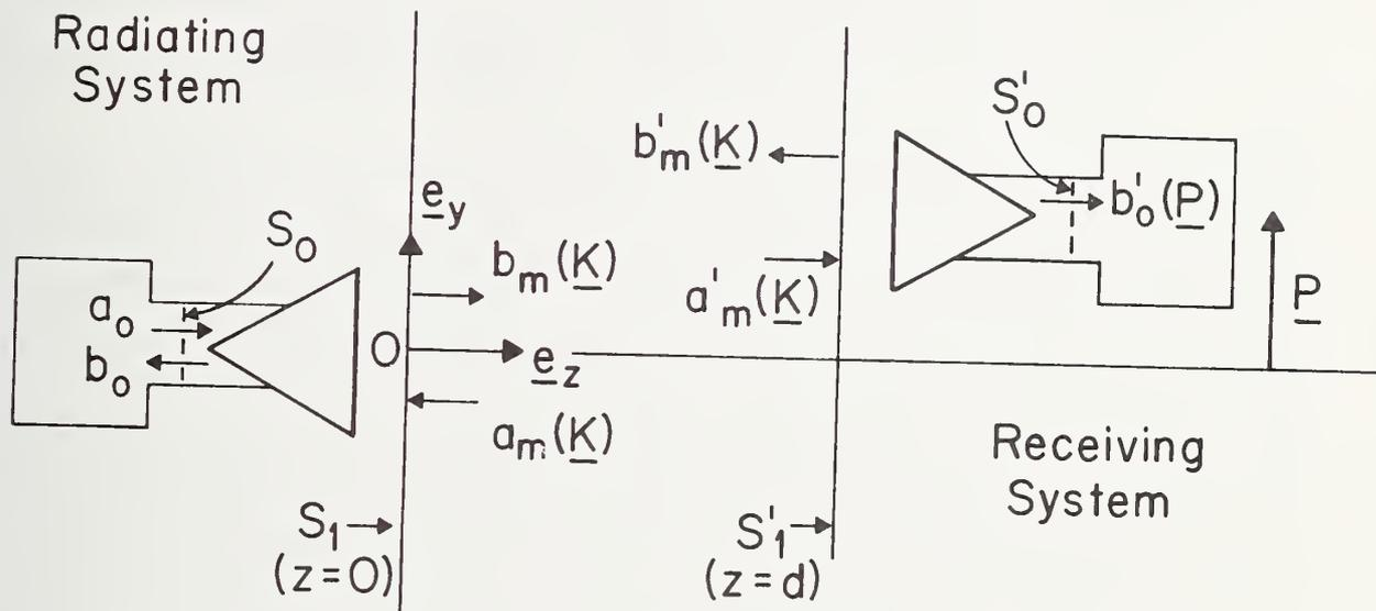
Figure 4. Relative Orientations of the Test Antenna and Probe.
