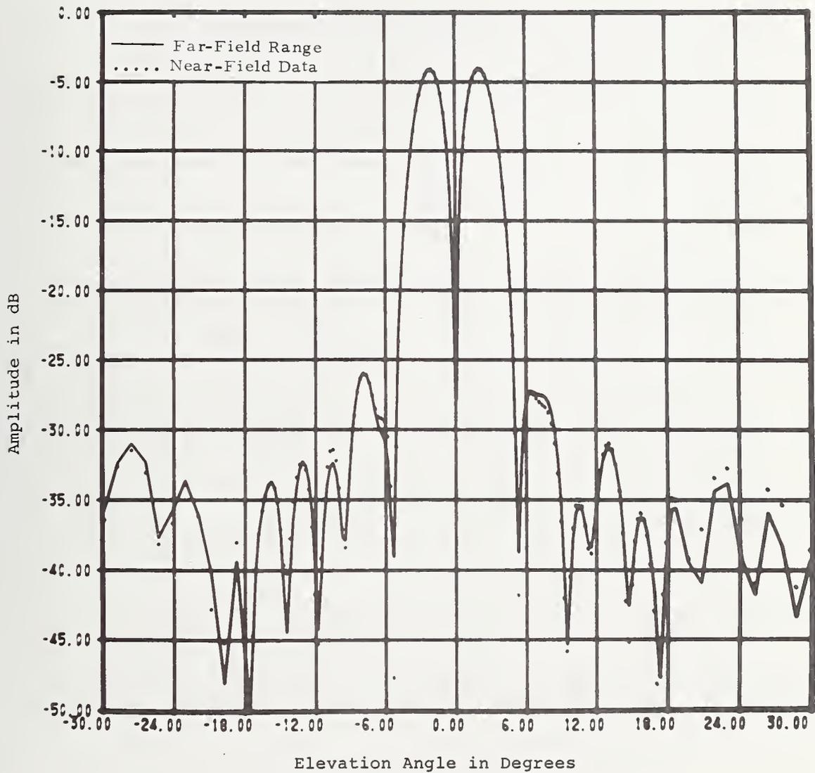
Figure 44. Comparison Between Far-Field Patterns Measured on Far-Field Range and Computed from Near-Field Data. Constrained Lens, E-Plane Elevation Difference.
