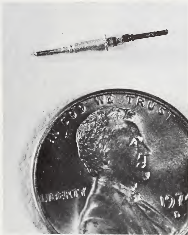
Fig. 6-1. Modified microminiature mercury switch. Center contact and end terminal shorted with silver paint.
