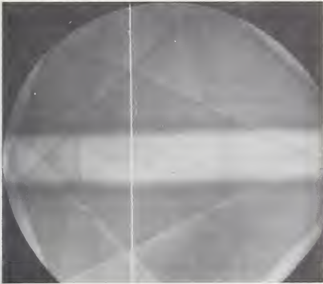
Fig. 2 Electron channelling pattern of annealed, electropolished aluminum. Line indicates region from which profile information was taken.
