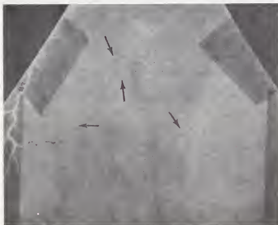
Fig. 24 Reflection Kossel pattern of iron crystal. Lines (indicated by arrows) include \{220\} , \{211\} and \{200\} types.
