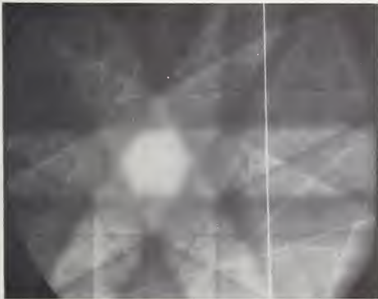
Fig. 20 Electron channelling pattern of silicon with crystal tilted 17^\circ with respect to electron beam axis. Line indicates profile trace position.
