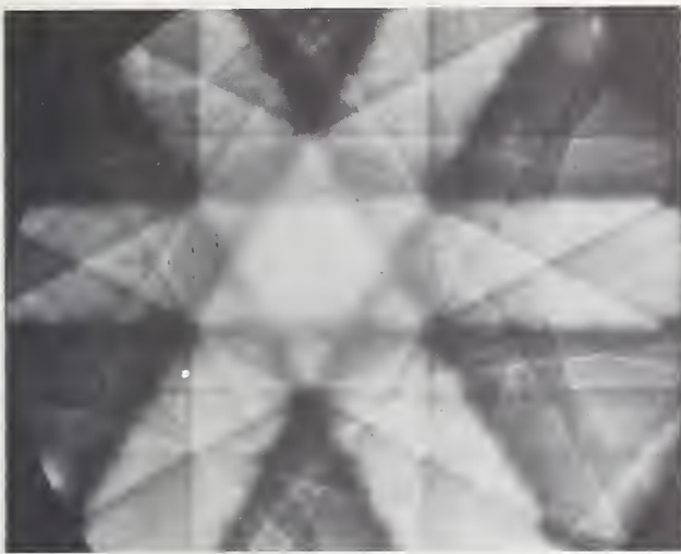
Fig. 18 Electron channelling pattern of silicon with crystal normal to electron beam axis. Line indicates profile trace position.
