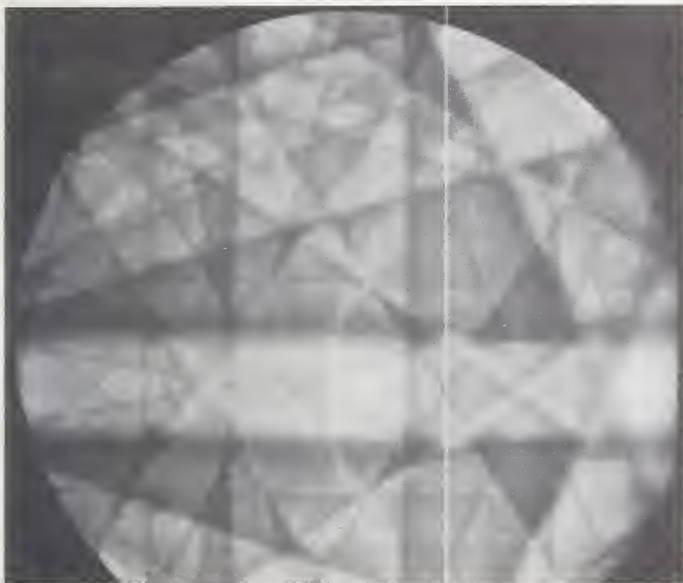
Fig. 6 Electron channelling pattern from chemically polished niobium crystal. Line indicates profile trace position.
