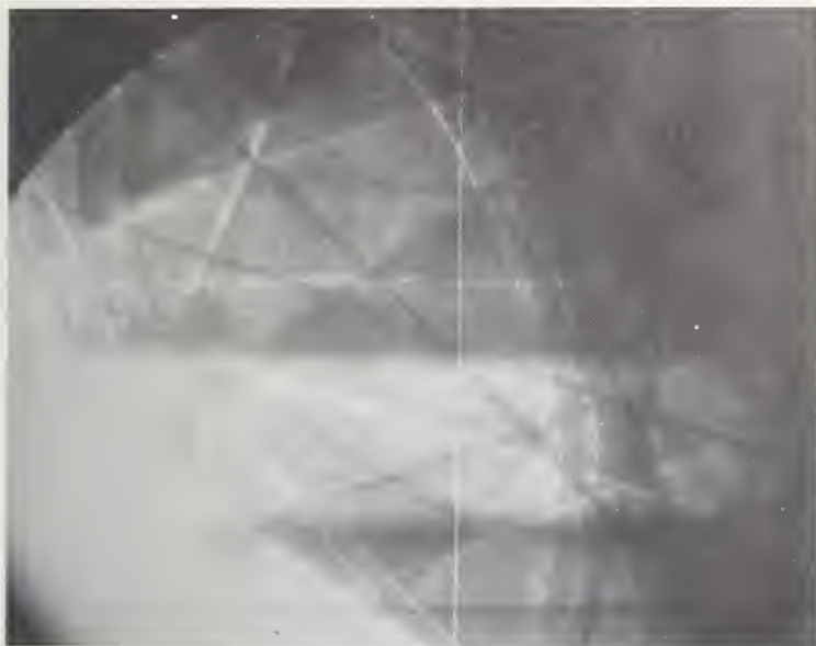
Fig. 22 Electron channelling pattern of silicon with crystal tilted 24.6^\circ with respect to electron beam axis. Line indicates profile trace position.
