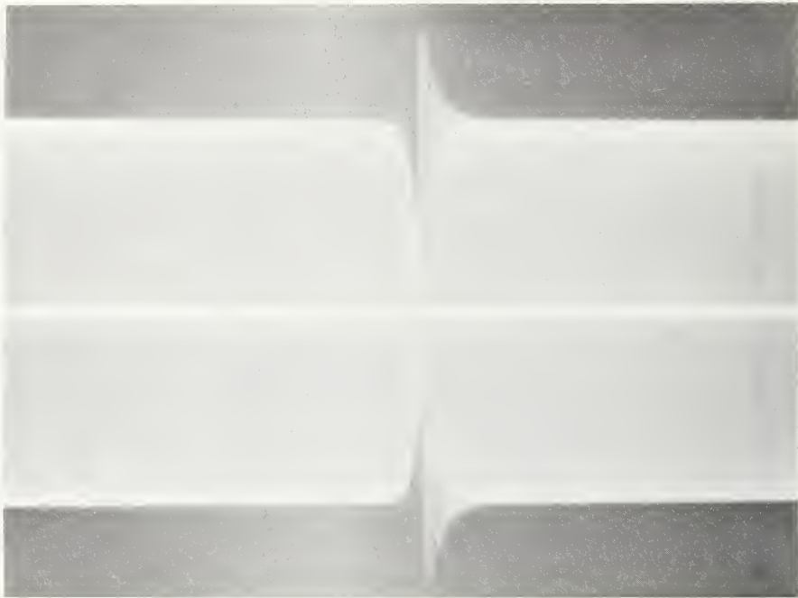
Figure 11(a). Expanded view of signal centered on the first mode. Horizontal scale 1 MHz full scale Pulse frequency 24.09 MHz Vertical scale 0.1 volt/cm
