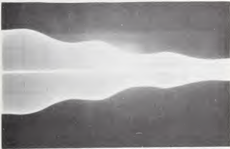
Figure 8(a). Signal reflected from an open coaxial line 20 feet long. Horizontal scale 20 - 50 MHz. Vertical scale 0.1 volt/cm.
