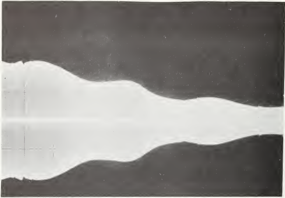
Figure 13(a). Signal from the whip antenna extended 25 inches. Horizontal scale 20 - 50 MHz. Vertical scale 0.1 volt/cm.
