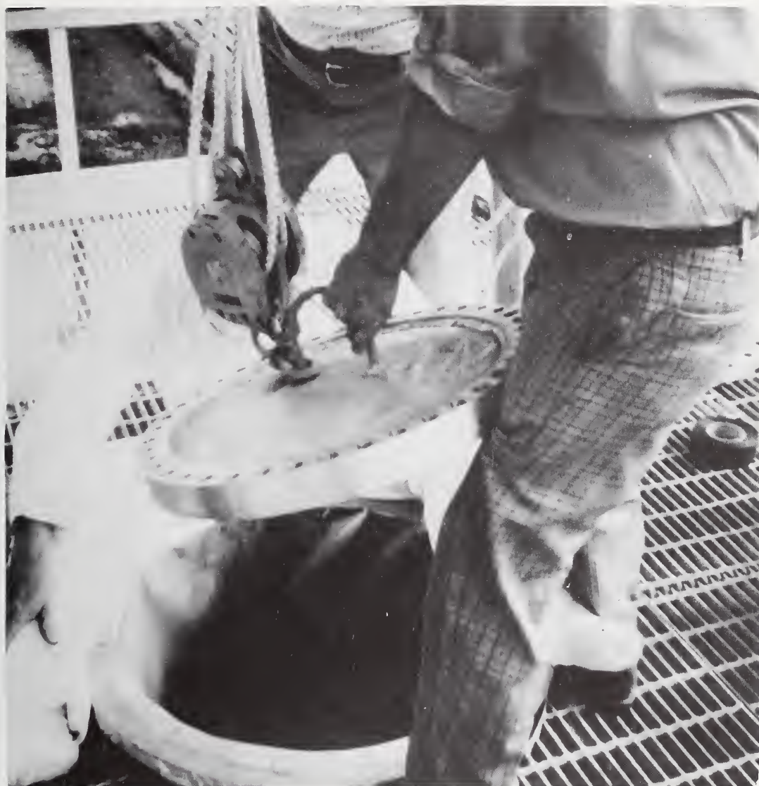
Figure 4. LOX tank inner manhole cover.
