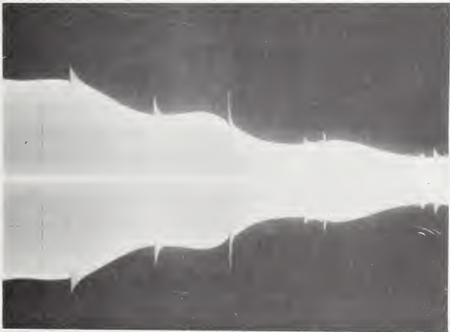
Figure 14(b). Signal from the whip antenna extended 49 inches.
