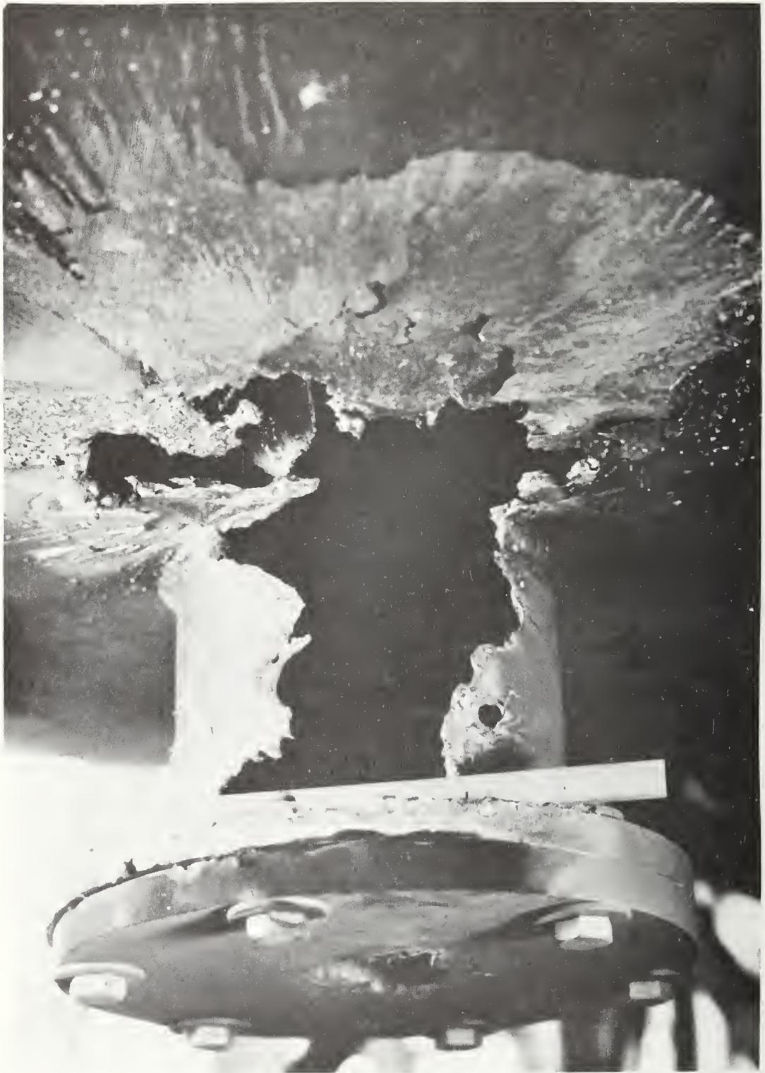
Figure 6. Bottom Port View, Tank Accident
