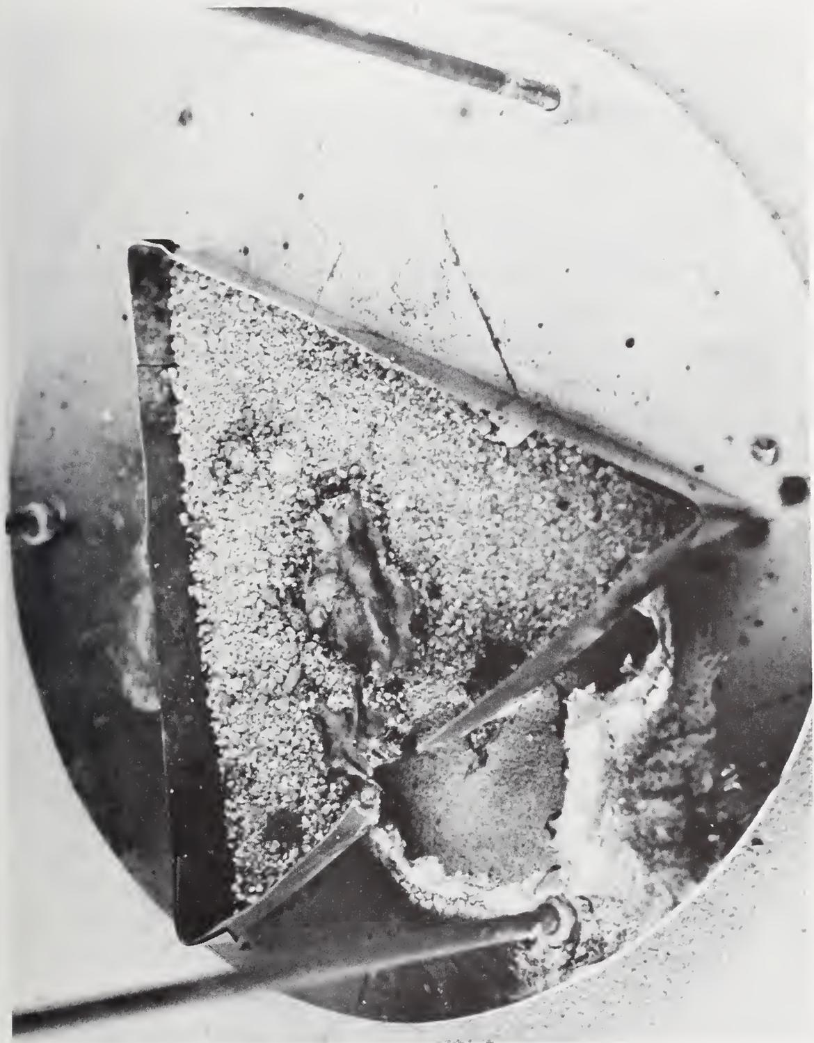
Figure 7. Copper Sand Tray SS Melt
