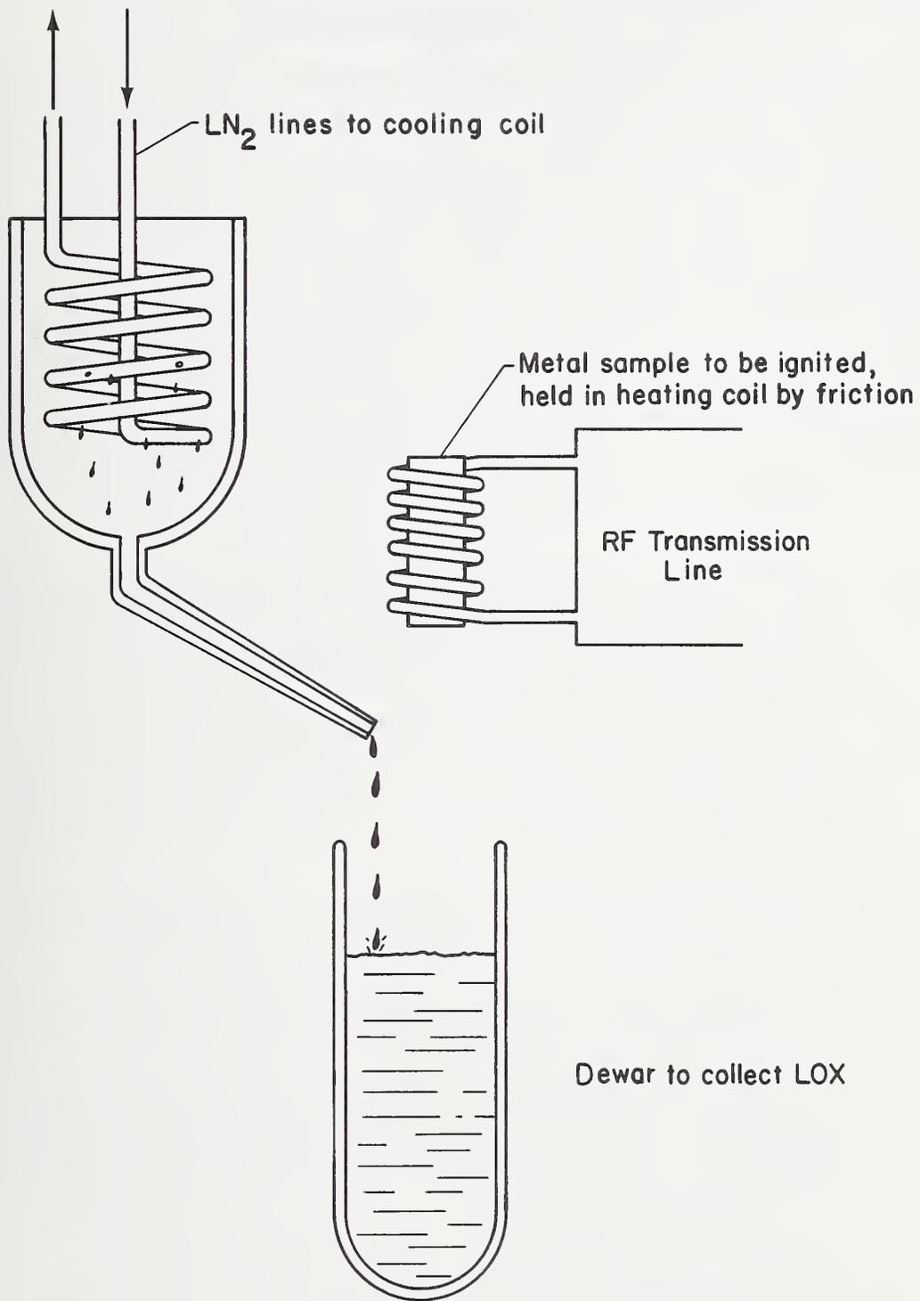
Figure 9. Liquid Oxygen Collection Apparatus
