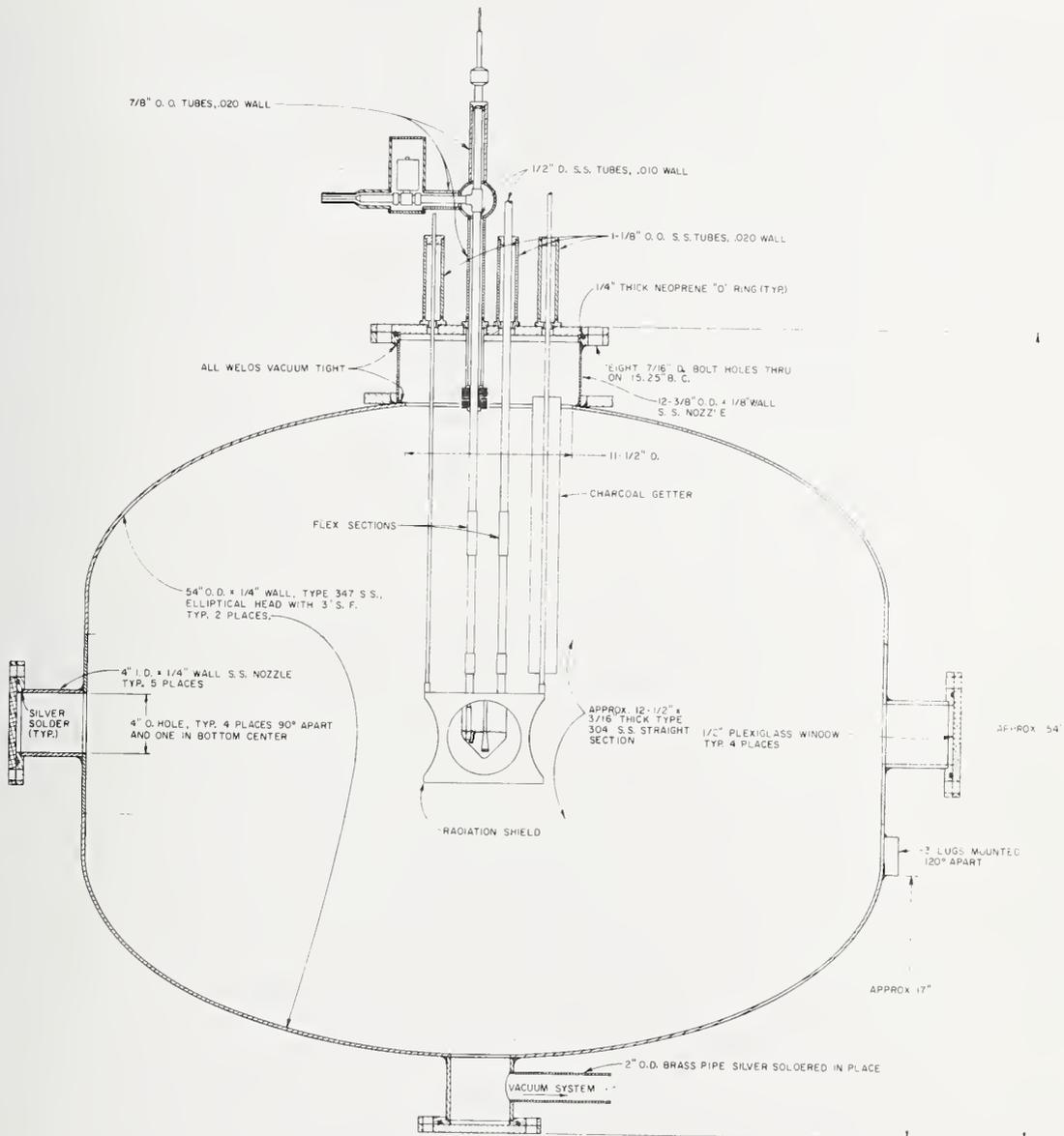
Figure 3.4.2 Assembly of Glass LH<sub>2</sub> Vessel and Large Metal Containment Vessel
