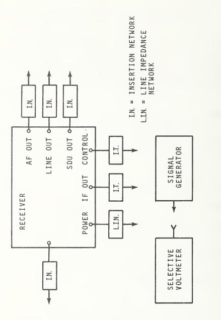
Fig. 4.6.1. Test Set-up for Conducted Emission
