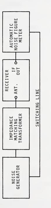
Fig. 4.1.6.1. Test Set-up for Noise Factor, ANFM Method
