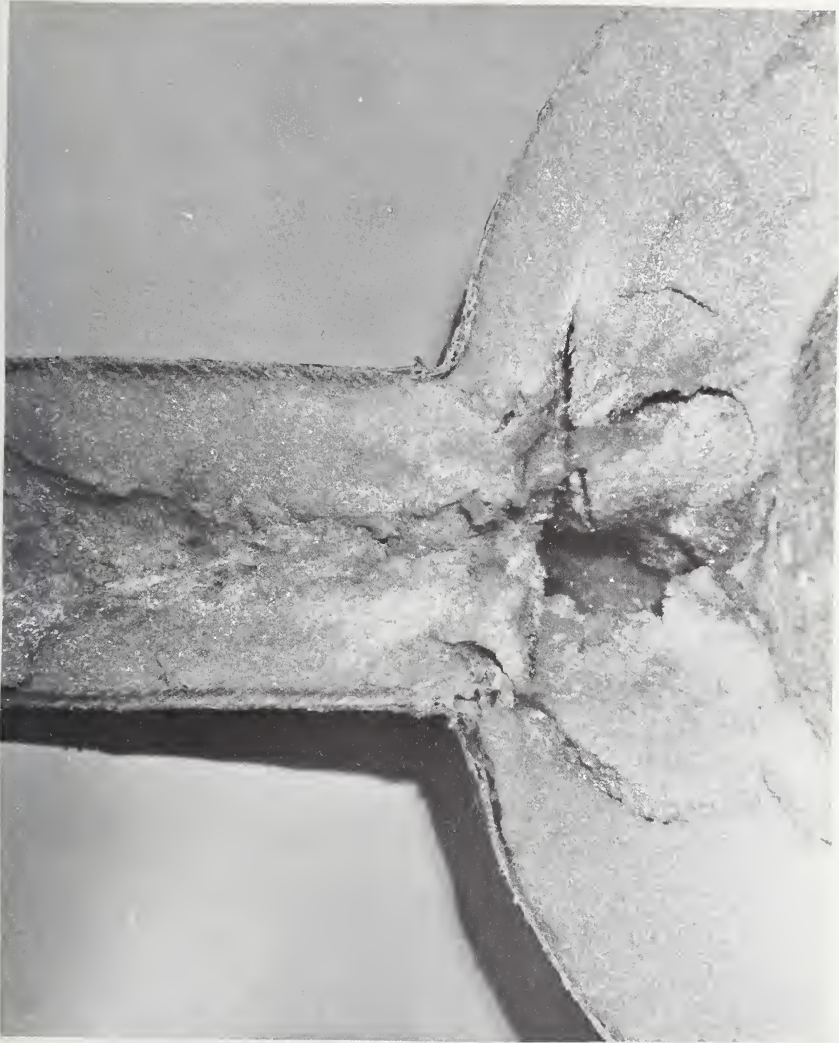
Figure 3. Voids in foam insulation at the dewar neck.
