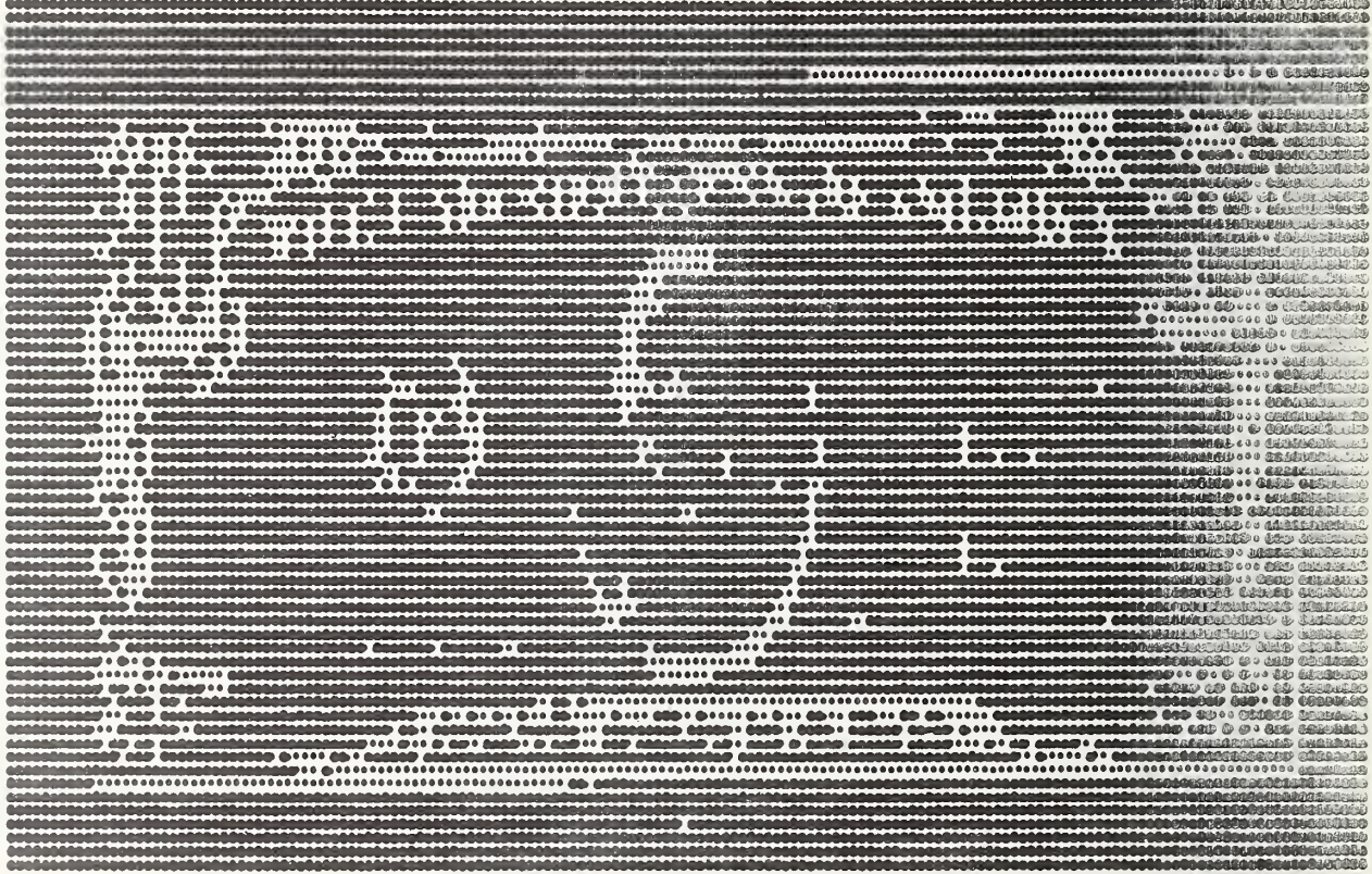
Figure 19. Computer printout showing where light from the images of the front side of a ten and a twenty dollar bill shine through a negative mask of the front side of a ten dollar bill.
