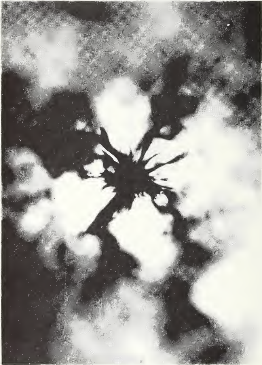
Fig. 12. The same damage site as in Fig. 11 but viewed between crossed polarizers. Note the highly strained region in the immediate vicinity of the damage site and also note the revelation of grain boundaries under stress. The magnification is 75X.
