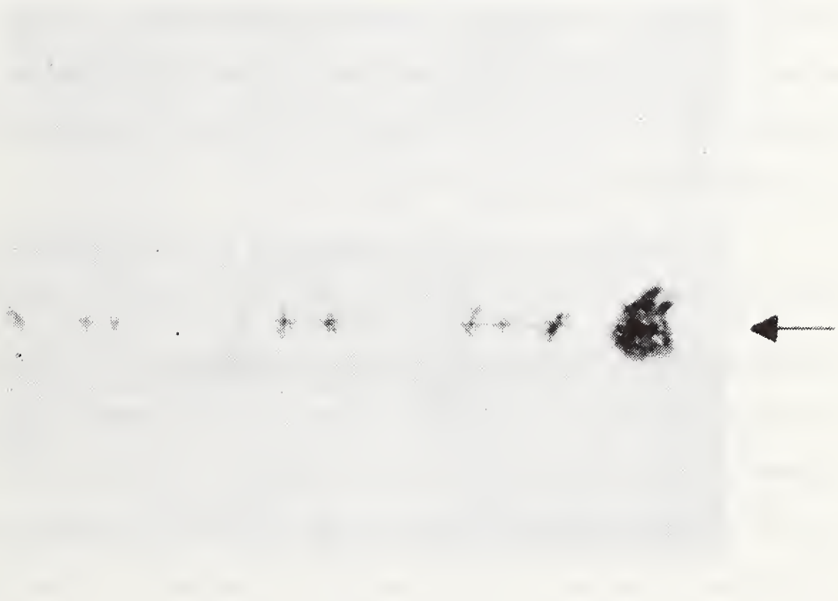
Fig. 10. Filamentary damage in \text{LiNbO}_3 which is indicative of self-focusing. The magnification is 42X.
