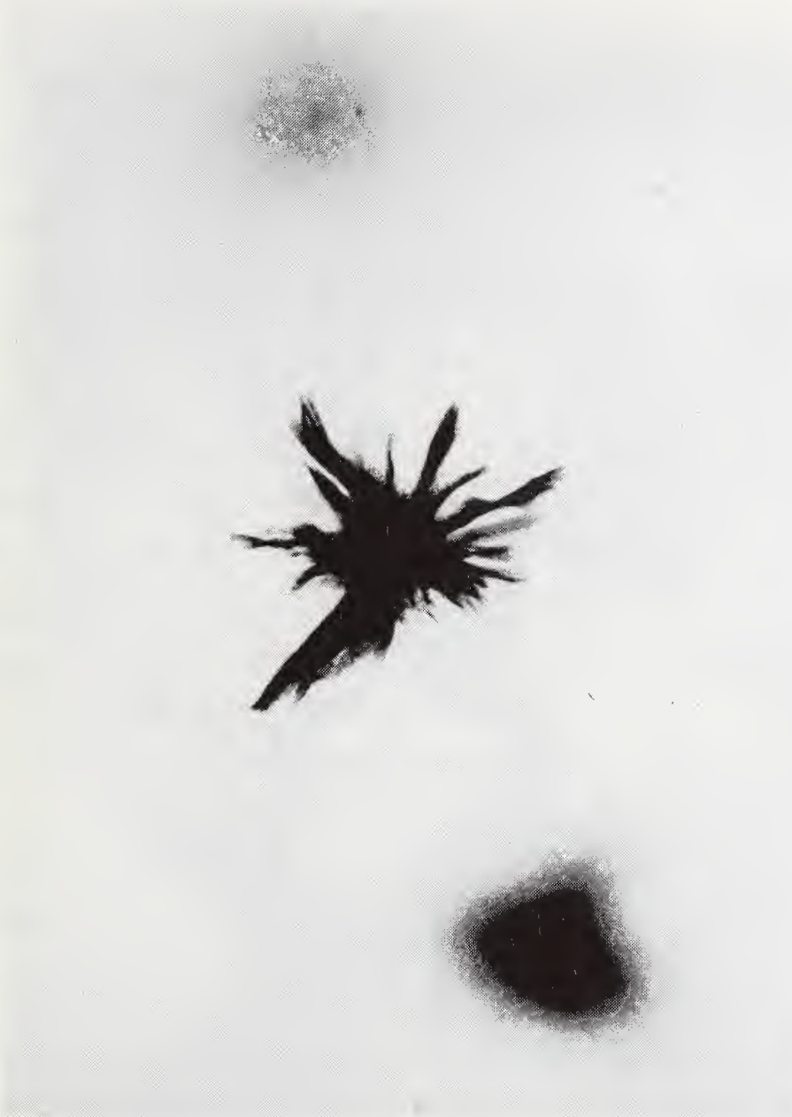
Fig. 11. Bulk damage site in a laser rod of neodymium-doped thoria:yttrium oxide ceramic as viewed along the rod axis in transmitted white light. The magnification is 75X. Note radial cracks that propagate with jogs caused probably by grain boundaries.
