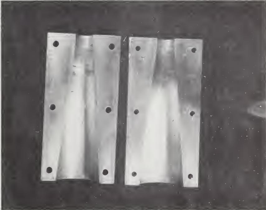
Figure 12 - Aluminum block experimental end fittings.
