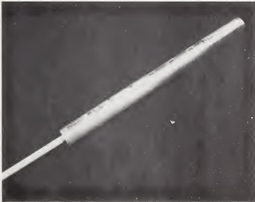
Figure 7 - Mod 4 experimental end fitting. Overall length, 18 in
