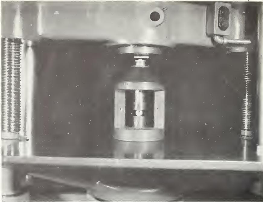
Figure 15 - Fractured disk specimen of FRP rod in subpress after diametral compression test.
