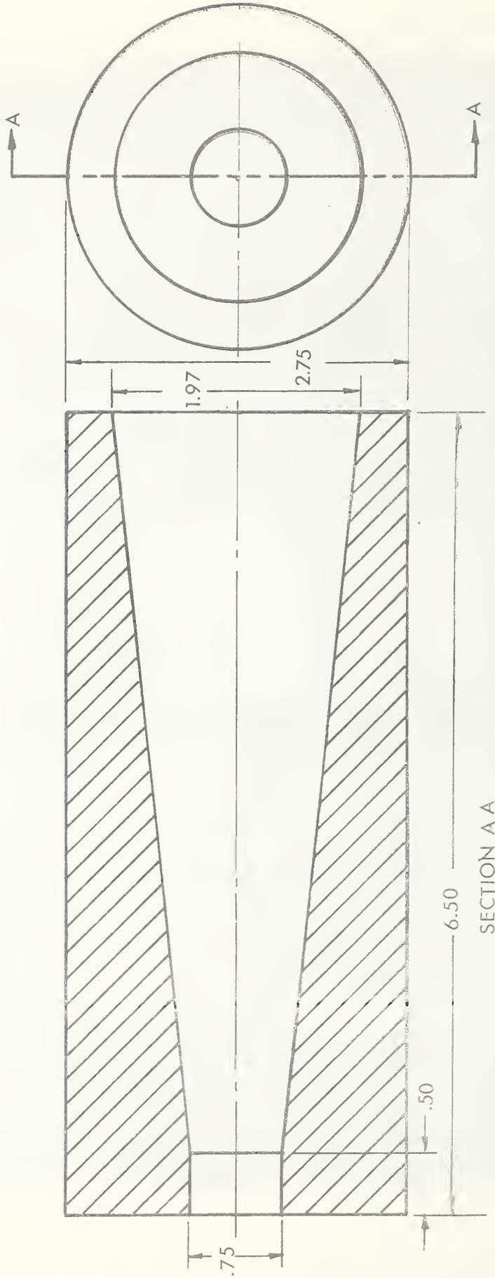
Figure 13 - H3M experimental end fitting. All dimensions in inches.
