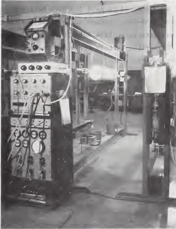
Figure 17 - One of six high-capacity creep testing machines for stress-rupture testing of long, FRP rod specimens under elevated temperature and saturated humidity conditions.
