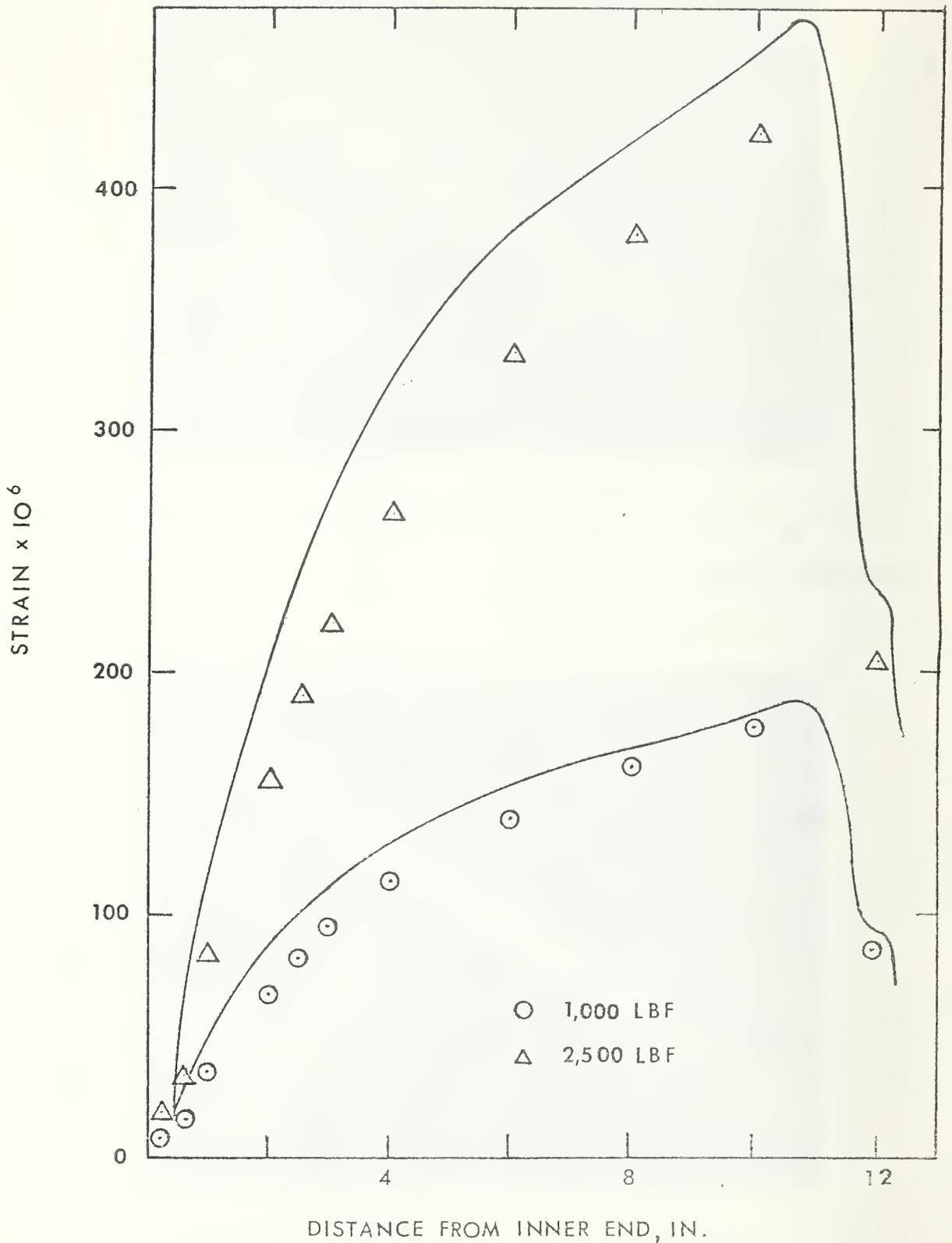
Figure 8 - Longitudinal normal strain on the outer surface of a Mod 4 end fitting, low tension loads. Points are experimental; curves are analytical.
