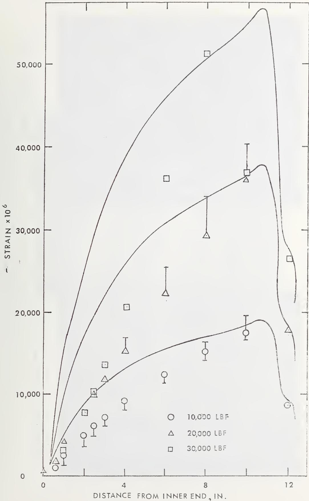
Figure 9 - Longitudinal normal strain on the outer surface of a Mod 4 end fitting, high tension loads. Points are experimental; curves are analytical.
