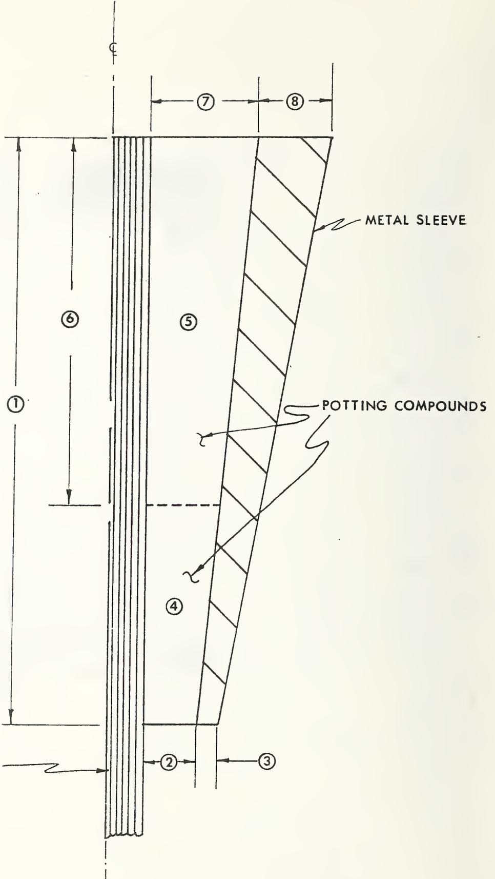
Figure 5 - Parameters for one general class of end fittings.
