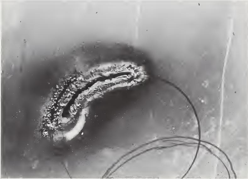
Figure 70. Comparison of Cuts Made by Rocket Torch (Wide) and Oxygen-fed Electric Arc (Narrow)
