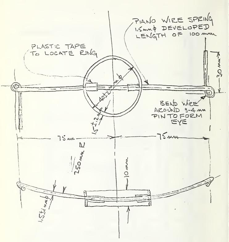
Figure 2 - Alternate Spring Design for Unexposed Thermocouples
