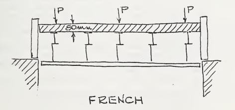
Mr. Malhotra suggested loading the beams without applying load to floor slabs. Professor Kordina agreed to develop the test method and it was accepted that the exposure of the specimen would be affected by the furnace pressure as well as the thermal properties of the floor slab. Britain has performed tests with different furnace pressures and observed significant variations in performance.
