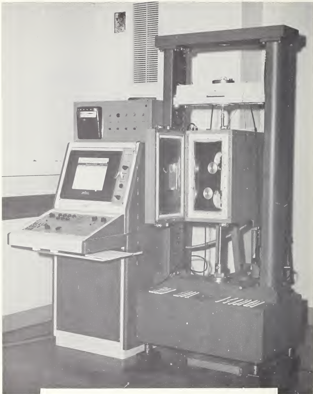
Fig. 2.2.3 Testing machine and temperature chamber.
