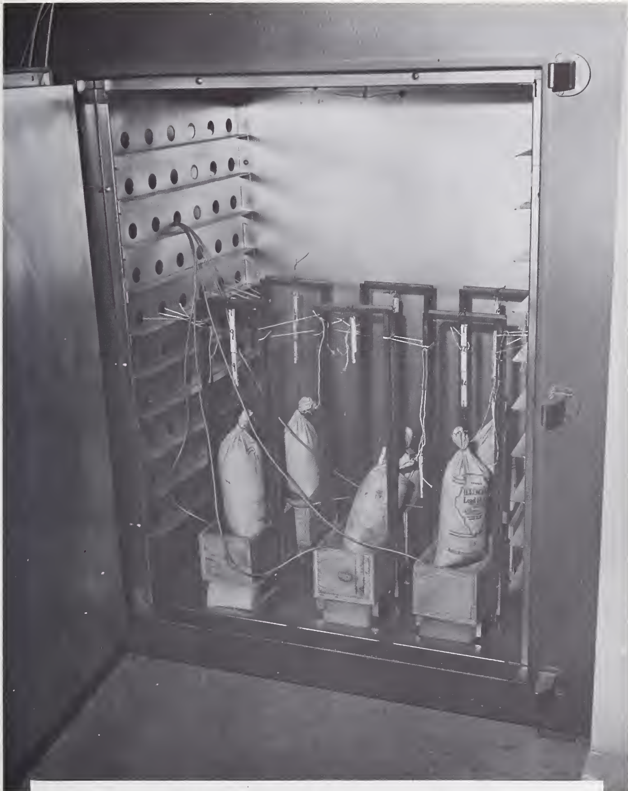
Fig. 2.2.4 Sustained loading apparatus and temperature chamber.
